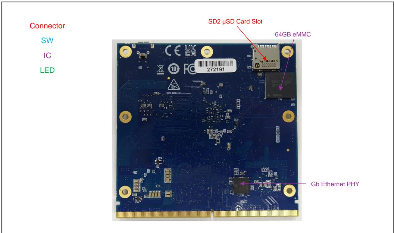
Figure 2.2 RZ/G3S SMARC Module Board Bottom View
