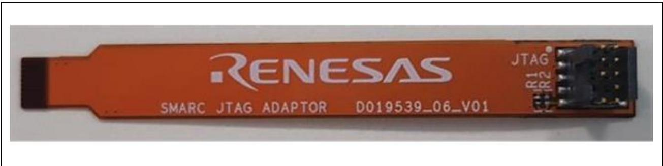
Figure 3.4 SMARC JTAG Adaptor Top View
