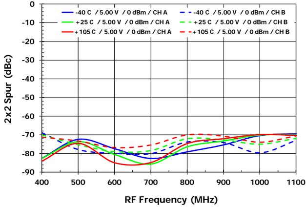
2x2 Rejection vs. T<sub>case</sub> [2x2<sub>MXR</sub>, LS rejection]
