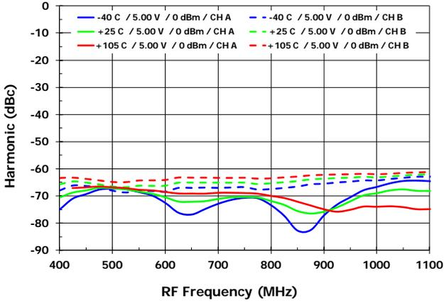
HD2 vs. T<sub>case</sub> [HD2<sub>MXR</sub>, LS injection]
