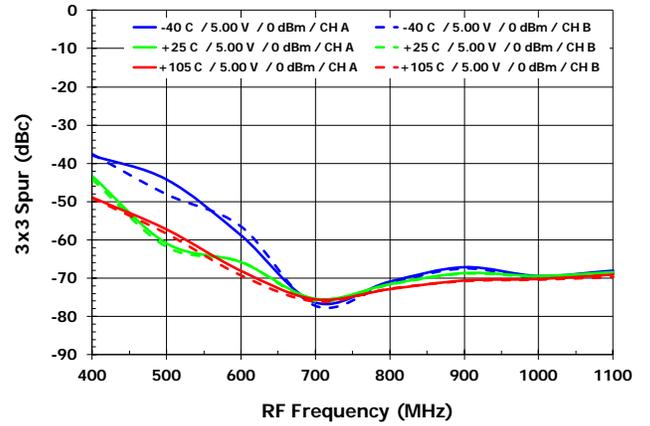
3x3 Rejection vs.  $V_{cc}$  [3x3<sub>MXR</sub>, HS rejection]
