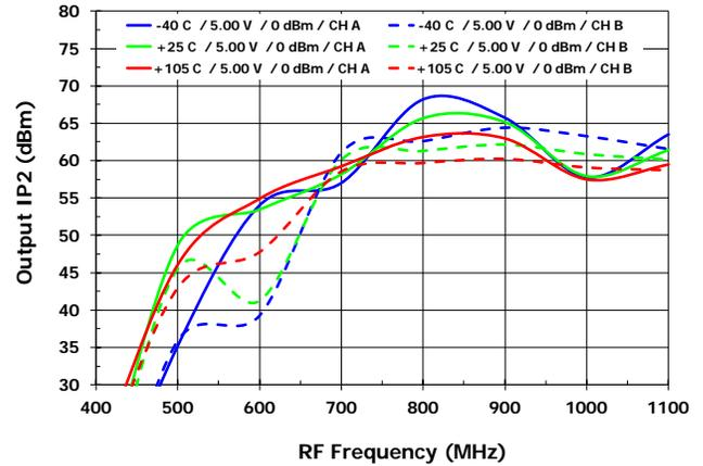
OIP2 vs. V<sub>cc</sub> [OIP2<sub>MXR</sub>, HS injection]
