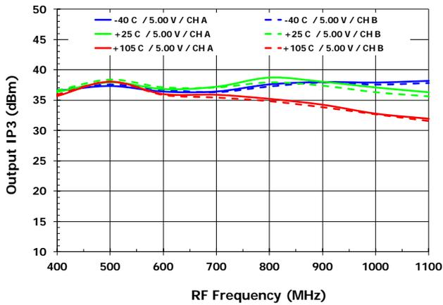
Output IP3 vs.  $V_{cc}$  [OIP3VGA]
