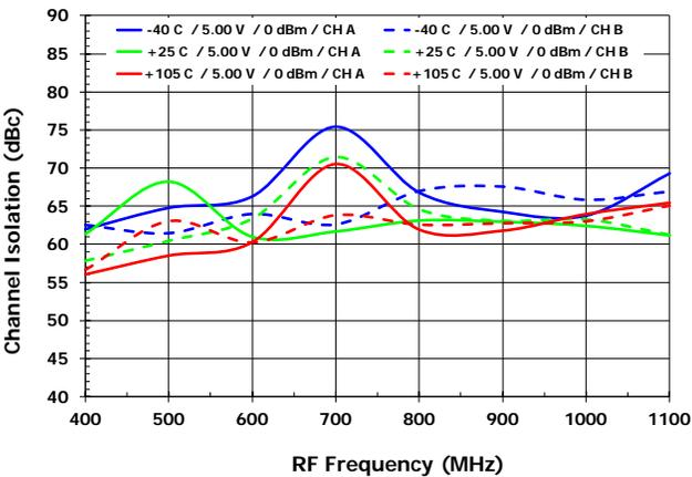
Channel Isolation vs.  $T_{case}$  [ISO<sub>IF</sub>, LS injection]
