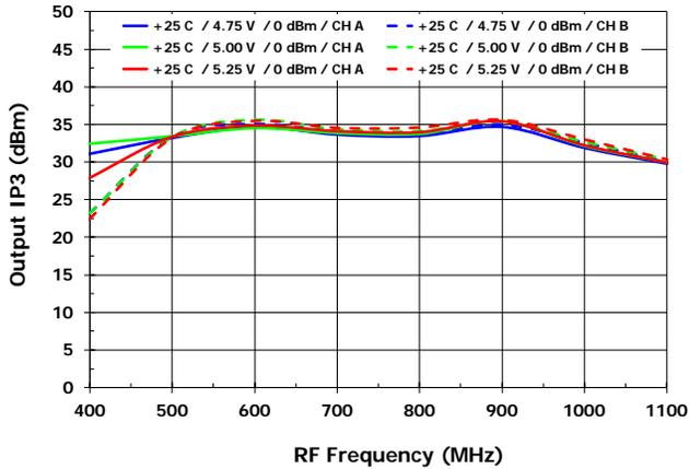
OIP3 vs. V<sub>cc</sub> [OIP3<sub>MXR</sub>, LS injection]
