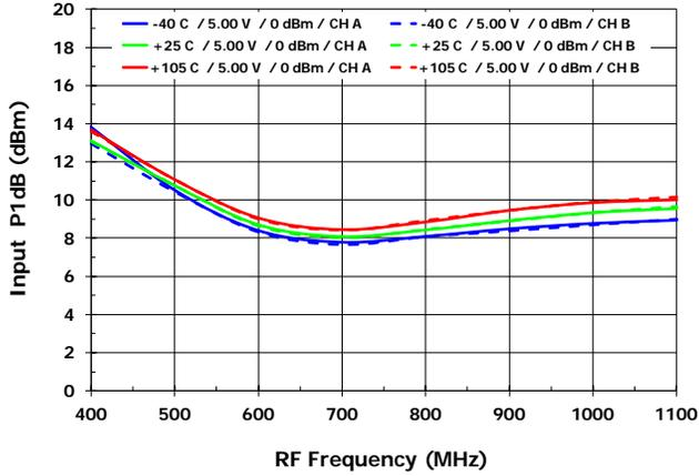
IP1dB vs. T<sub>case</sub> [IP1dB<sub>MXR</sub>, LS injection]
