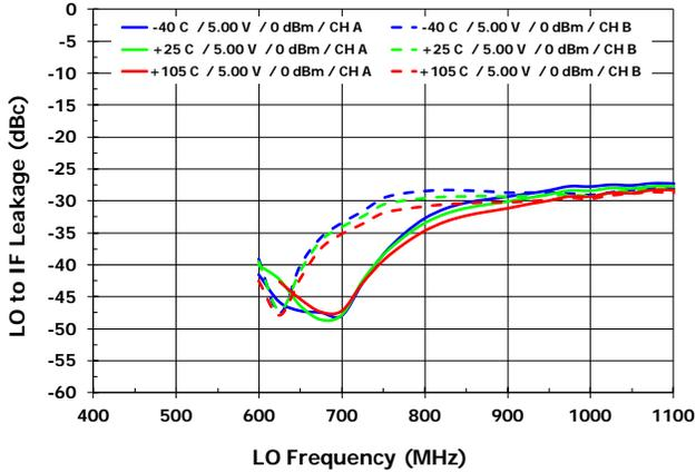
LO to IF Leakage vs.  $T_{case}$  [ISO<sub>LI</sub>, LS injection]
