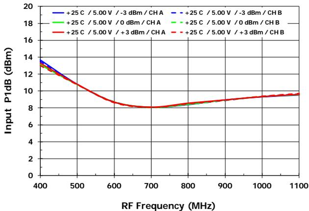
IP1dB vs. LO Power [IP1dB<sub>MXR</sub>, LS injection]
