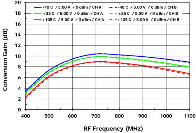
Gain vs. T<sub>case</sub> [G<sub>MXR</sub>, LS Injection]
