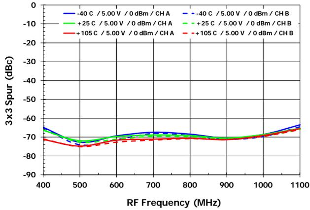
3x3 Rejection vs.  $T_{case}$  [3x3<sub>MXR</sub>, LS rejection]
