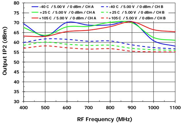
OIP2 vs. T<sub>case</sub> [OIP2<sub>MXR</sub>, LS injection]
