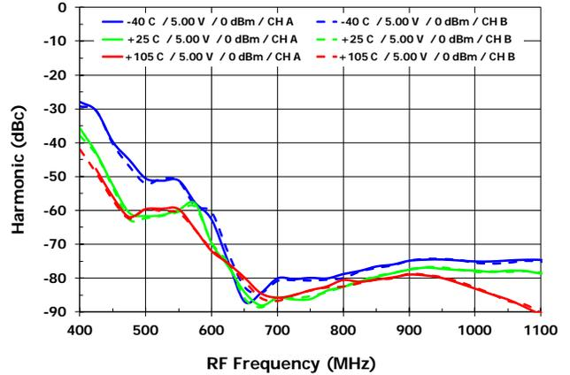
HD3 vs.  $V_{CC}$  [HD3<sub>MXR</sub>, HS injection]
