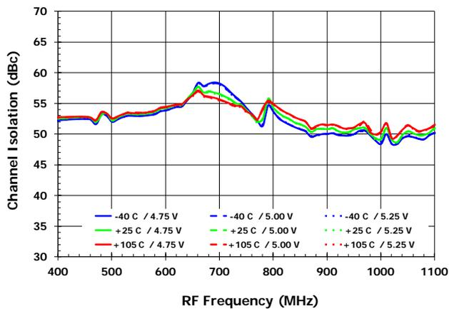
Channel Isolation vs.  $T_{case}$  &  $V_{cc}$  [ISO<sub>B-A</sub>]
