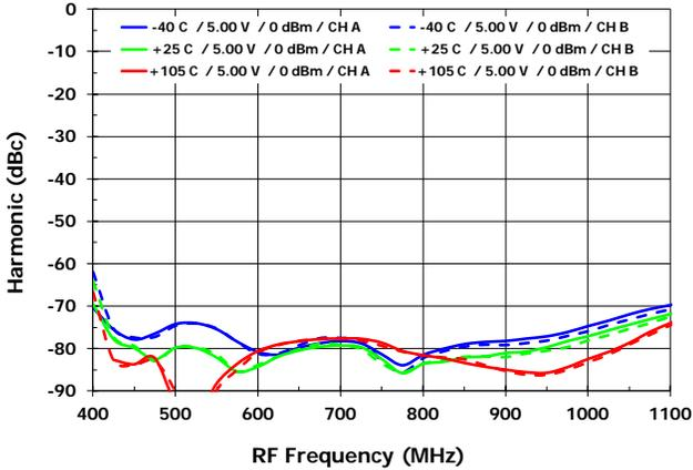
HD3 vs.  $T_{case}$  [HD3<sub>MXR</sub>, LS injection]
