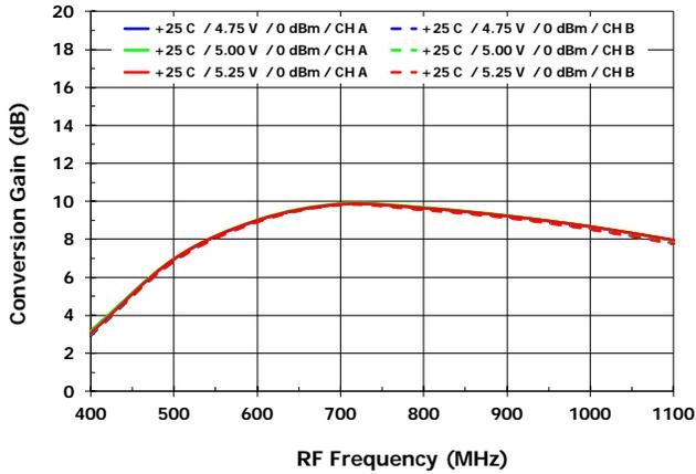
Gain vs. V<sub>cc</sub> [G<sub>MXR</sub>, LS Injection]
