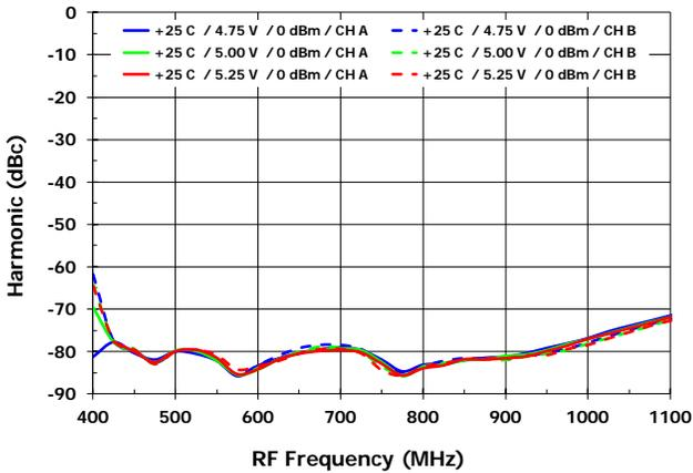
HD3 vs.  $V_{CC}$  [HD3<sub>MXR</sub>, LS injection]
