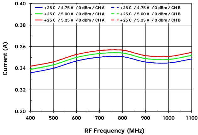
Current consumption vs.  $V_{cc}$  [LS injection]
