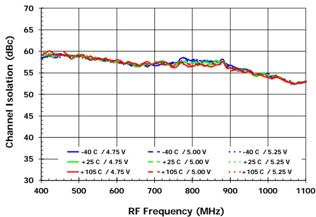
Channel Isolation vs.  $T_{case}$  &  $V_{cc}$  [ $ISO_{B-A}$ ]
