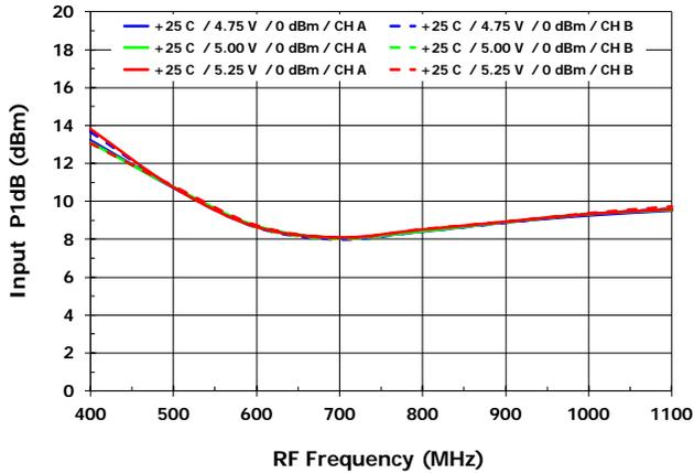
IP1dB vs. V<sub>cc</sub> [IP1dB<sub>MXR</sub>, LS injection]
