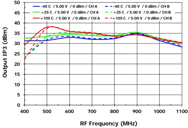
OIP3 vs. T<sub>case</sub> [OIP3<sub>MXR</sub>, LS injection]
