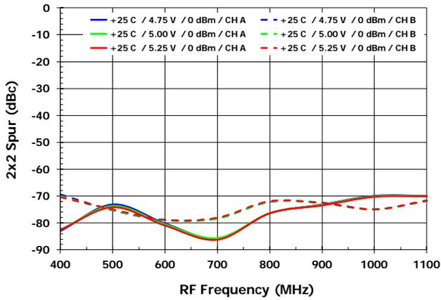
2x2 Rejection vs. V<sub>cc</sub> [2x2<sub>MXR</sub>, LS rejection]
