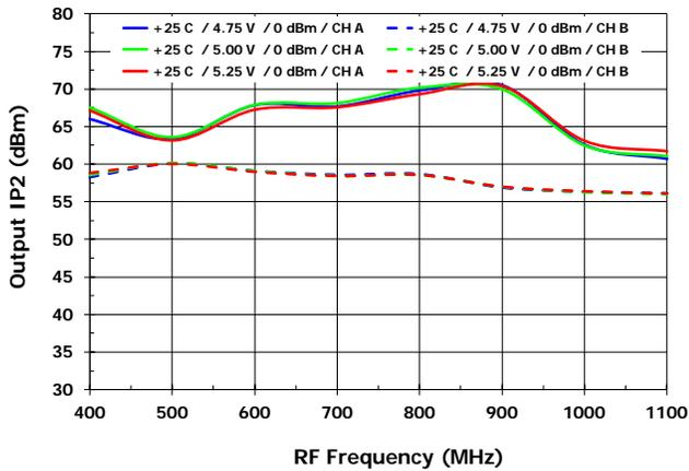
OIP2 vs. V<sub>cc</sub> [OIP2<sub>MXR</sub>, LS injection]
