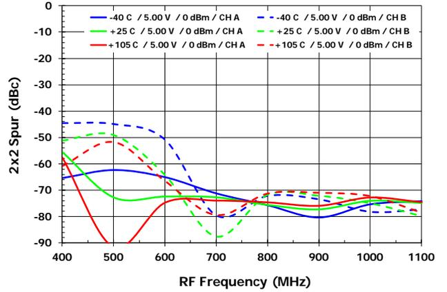
2x2 Rejection vs. V<sub>cc</sub> [2x2<sub>MXR</sub>, HS rejection]
