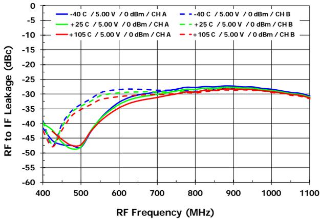
RF to IF Rejection vs.  $T_{case}$  [ISO<sub>RI</sub>, LS injection]
