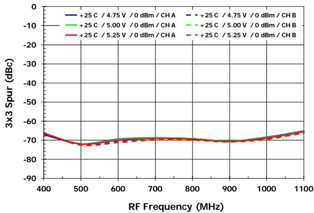
3x3 Rejection vs.  $V_{cc}$  [3x3<sub>MXR</sub>, LS rejection]
