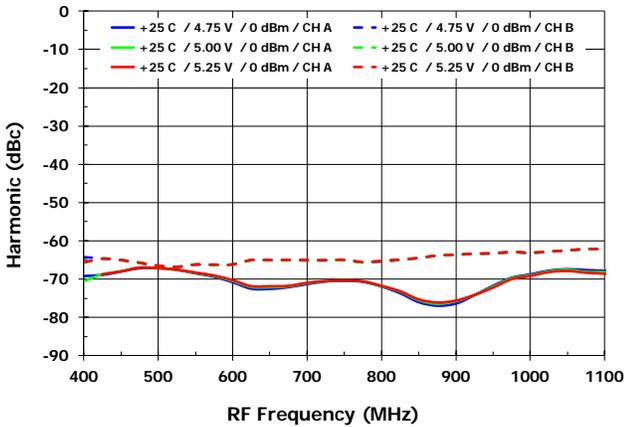
HD2 vs. V<sub>CC</sub> [HD2<sub>MXR</sub>, LS injection]
