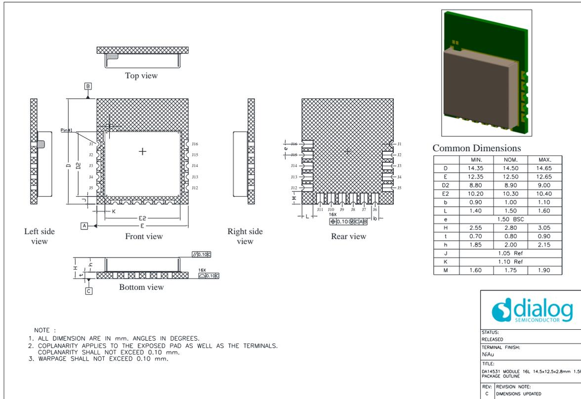
Figure 3: Mechanical Drawing
