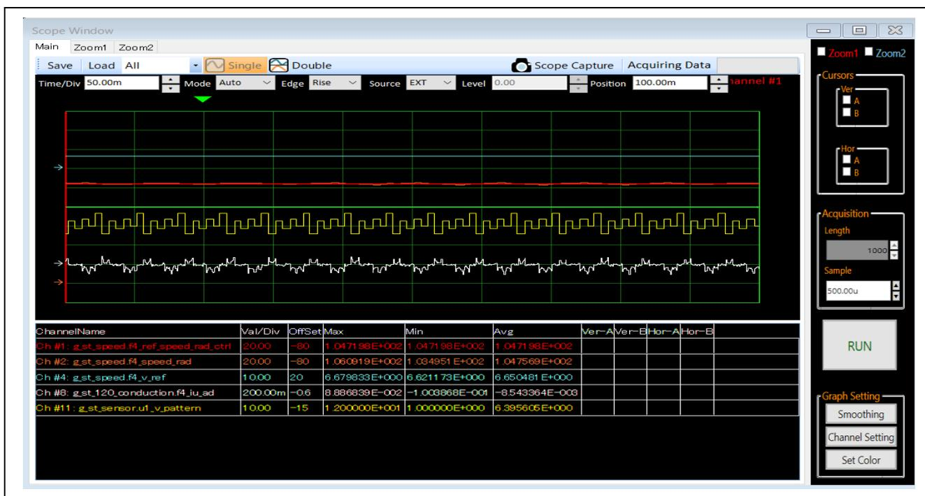
**Figure 7-1 Speed control using Hall 120-degree conducting control**
