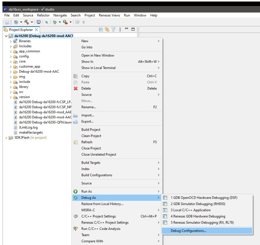
Figure 36: Run Debug Mode
