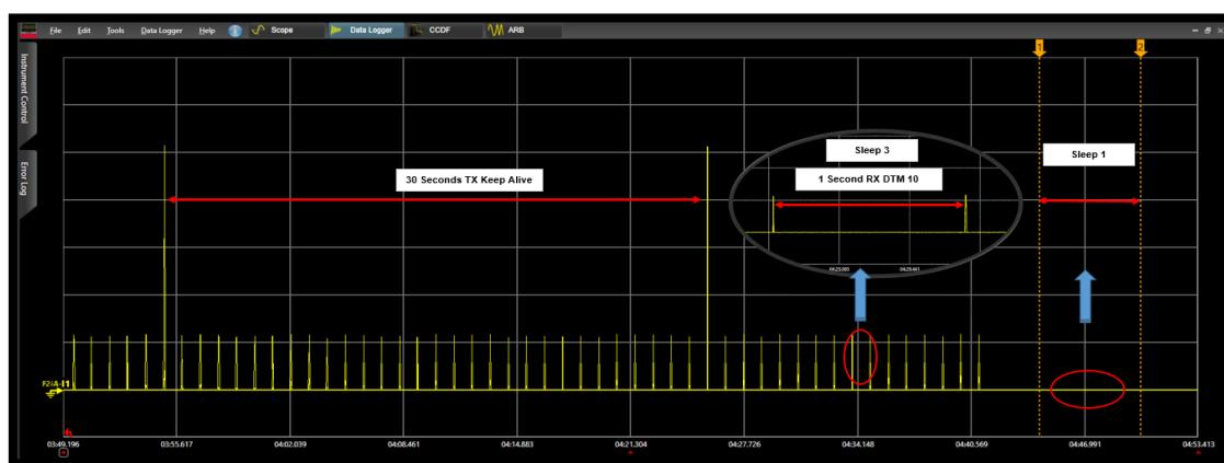
Figure 63: Measuring Current in DPM Low Power Mode
