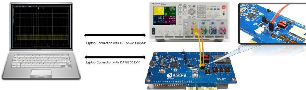
**Figure 49: Current Test Environment with 14585A**
