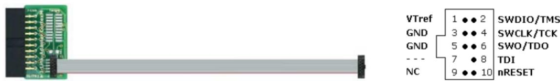
**Figure 34: J-Link 9-pin Cortex-M Adapter**
