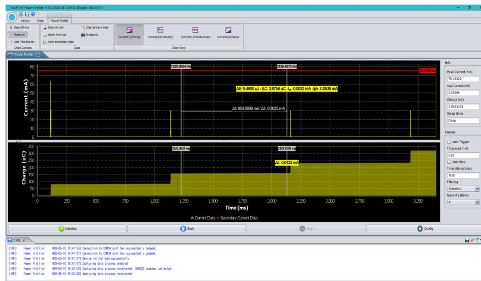
**Figure 60: Measuring Consumption by Using Chart Controls**
