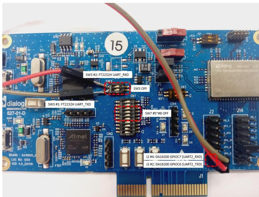
**Figure 70: Modification and Connection of EVB V4.0**
