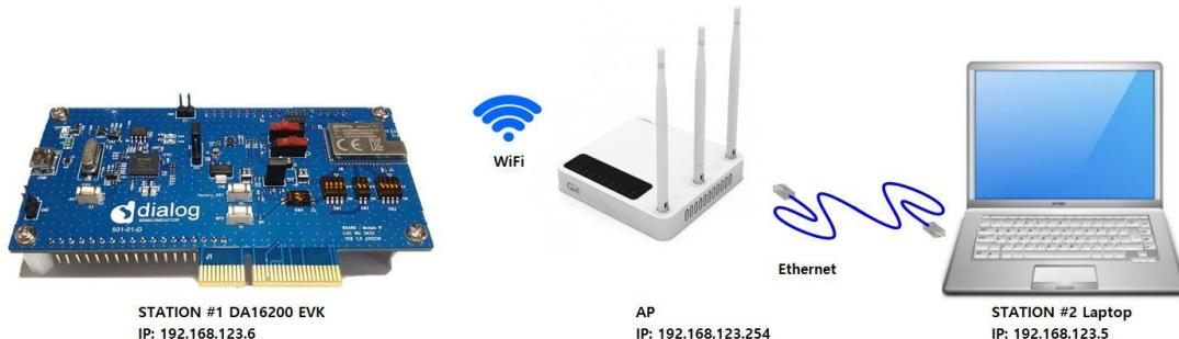
Figure 47: Throughput Test Environment
