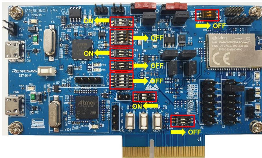
**Figure 10: Configure DA16600 EVB for AT Command - UART to FT2232H****Table 11: DA16600 EVB Switch Configuration for AT Command - UART to FT2232H**
