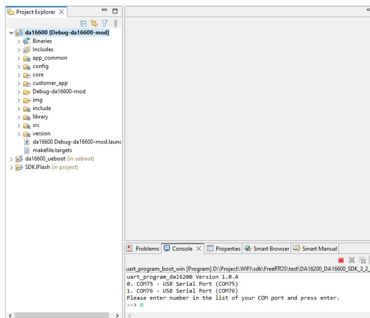
Figure 42: Select Number from Serial Interface List
