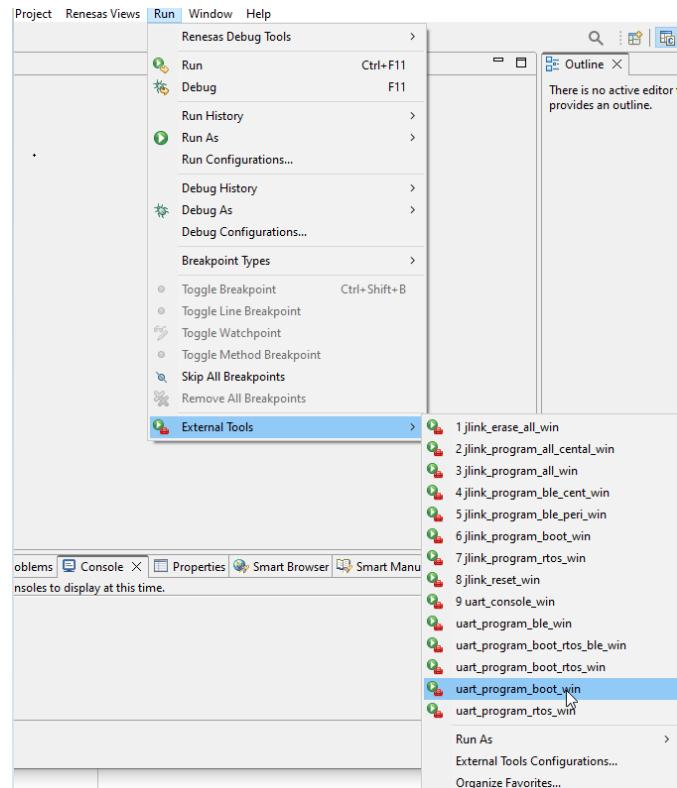
**Figure 41: Launch Configurations for Programming Firmware Images**
