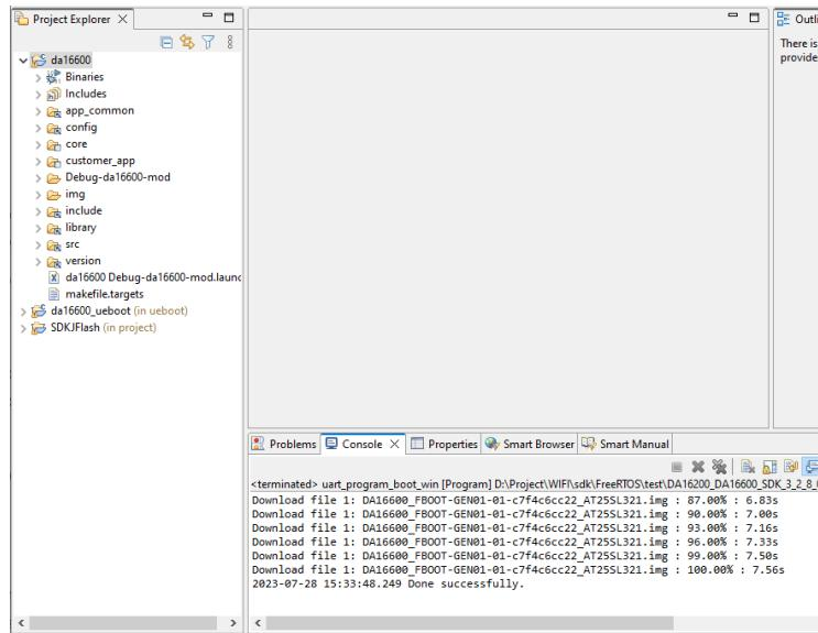
**Figure 43: Programming Firmware Image over Serial Interface**
