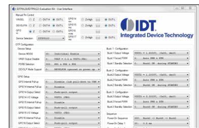
Various device features can be configured during production using one time programmable fuse memory (OTP). During evaluation, the options can be evaluated using the compatible IDT P9120 Evaluation Kit (IDTP9120-EVAL) and USB-Bridge (USB-BRIDGEV2-EVAL).
