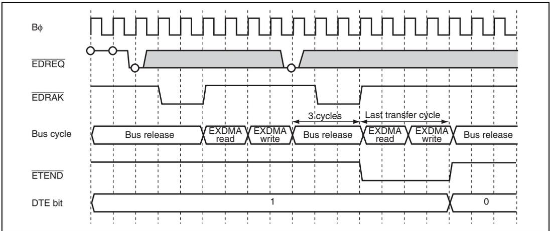
**Figure 11.44 External Request/Normal Transfer Mode/Cycle Steal Mode
