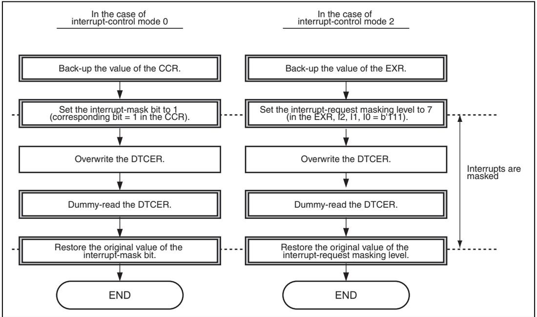
**Figure 12.17 Example of Procedures for Overwriting the DTCER**
