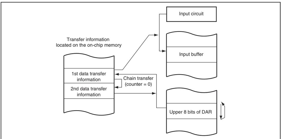
**Figure 12.16 Chain Transfer when Counter = 0**
