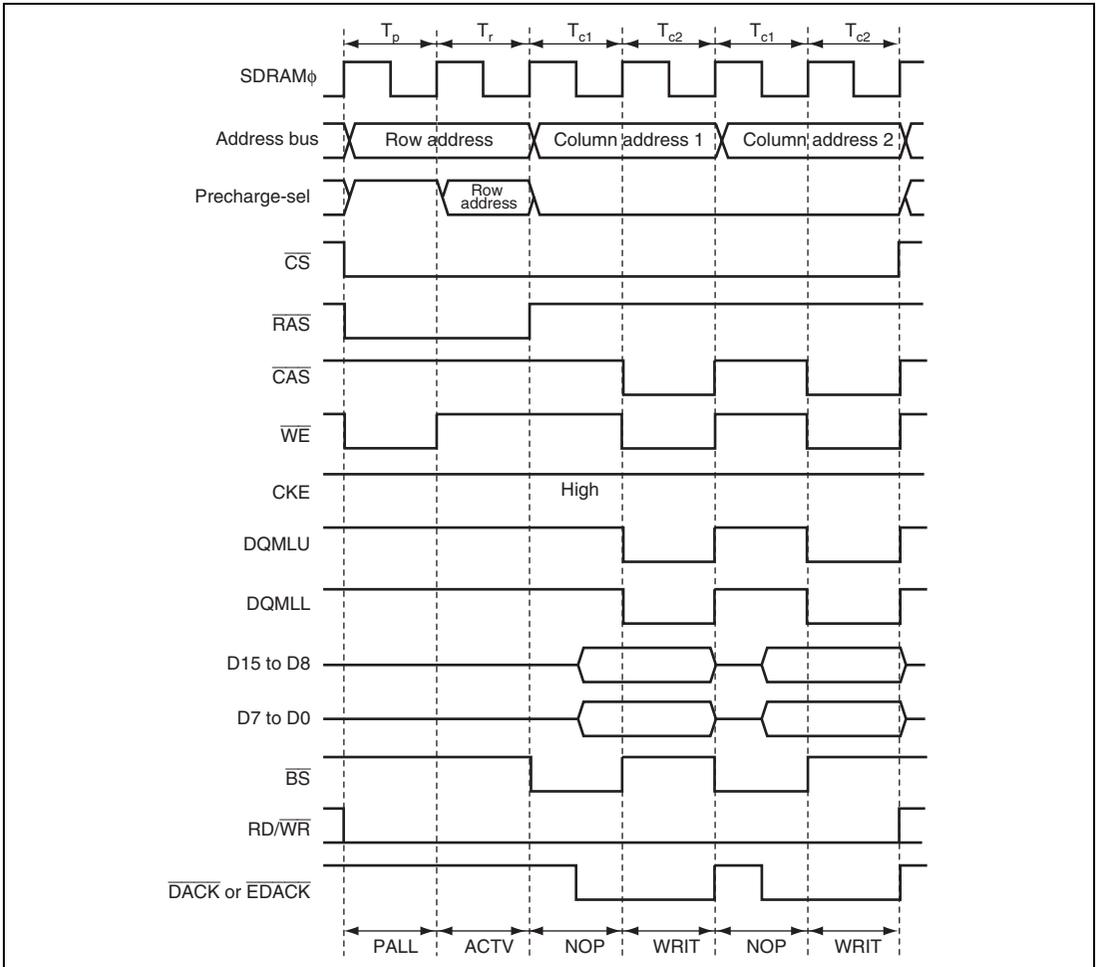
**Figure 9.83 Output Timing Example of  $\overline{\text{DACK}}$  and  $\overline{\text{EDACK}}$  when  $\text{DDS} = 1$  or  $\text{EDDS} = 1$  (Write)**
