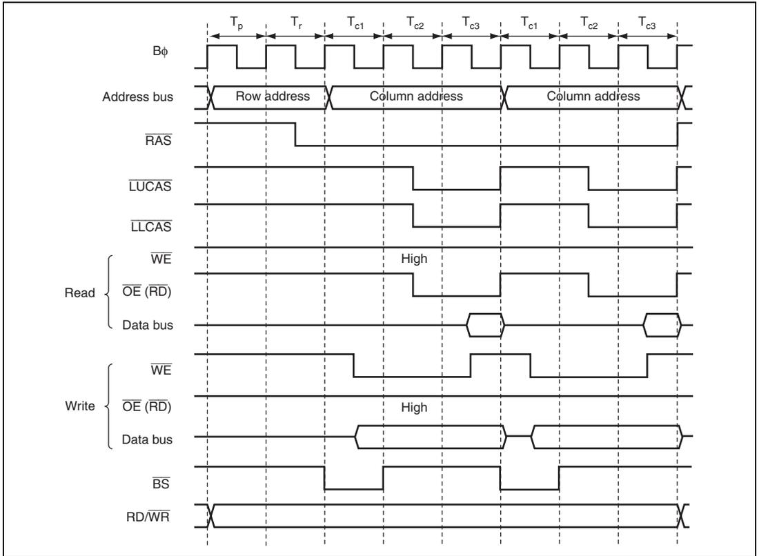
**Figure 9.49 Operation Timing of Fast-Page Mode (RAST = 0, CAST = 1)**
