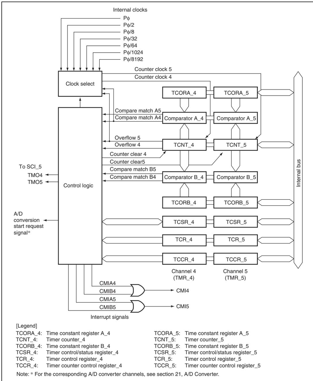
Figure 16.3 Block Diagram of 8-Bit Timer Module (Unit 2)
