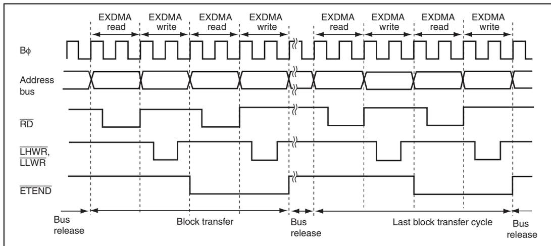
**Figure 11.28 Example of Block Transfer Mode Transfer**
