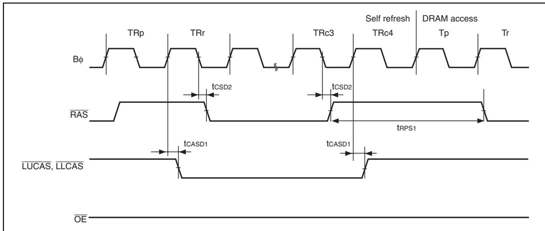
Figure 29.28 Self-Refresh Timing (After Leaving Software Standby: RAST=1)\*
