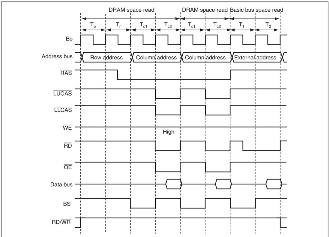
**Figure 9.51 Timing Example of RAS Up Mode (RAST = 0, CAST = 0)**
