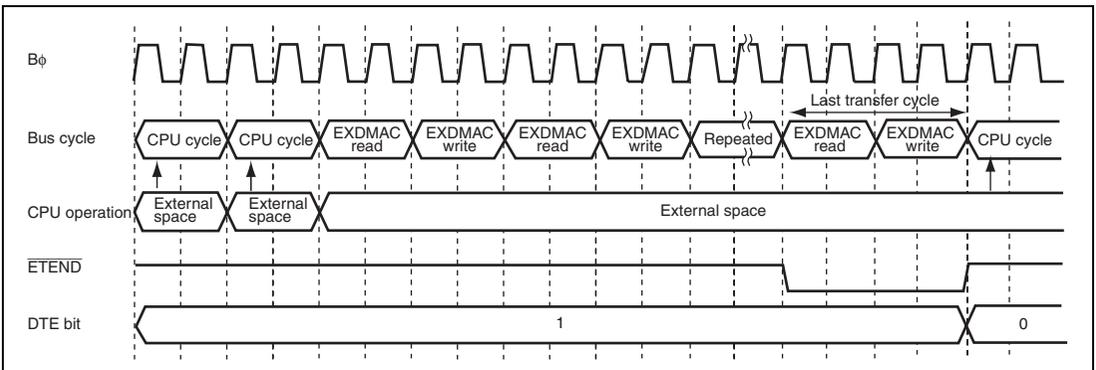
**Figure 11.41 Auto-Request/Normal Transfer Mode/Burst Mode
