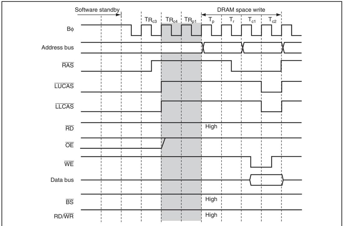
**Figure 9.57** Timing Example when 1 Precharge Cycle Added
