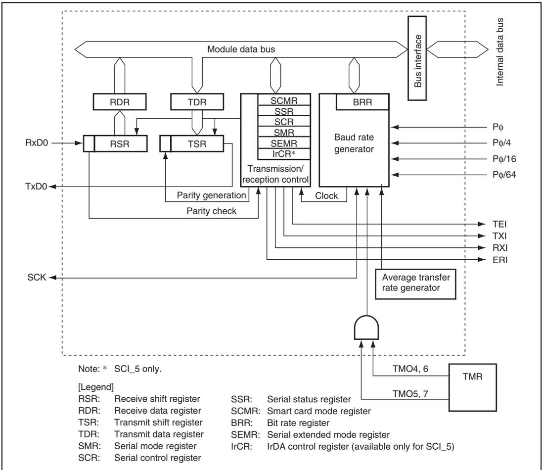
**Figure 19.2 Block Diagram of SCI\_5 and SCI\_6**
