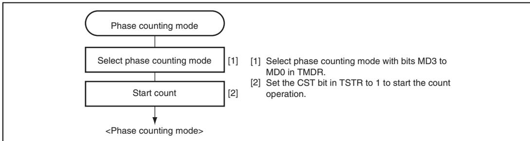
**Figure 14.25 Example of Phase Counting Mode Setting Procedure**
