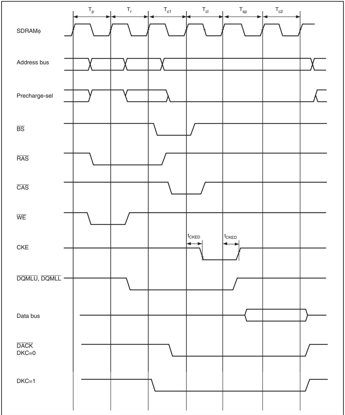
Figure 29.31 Extended Read Data Cycle (CAS Latency 2)\*
