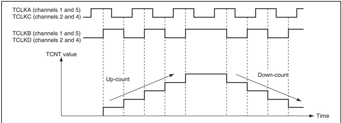
**Figure 14.29 Example of Phase Counting Mode 4 Operation**
