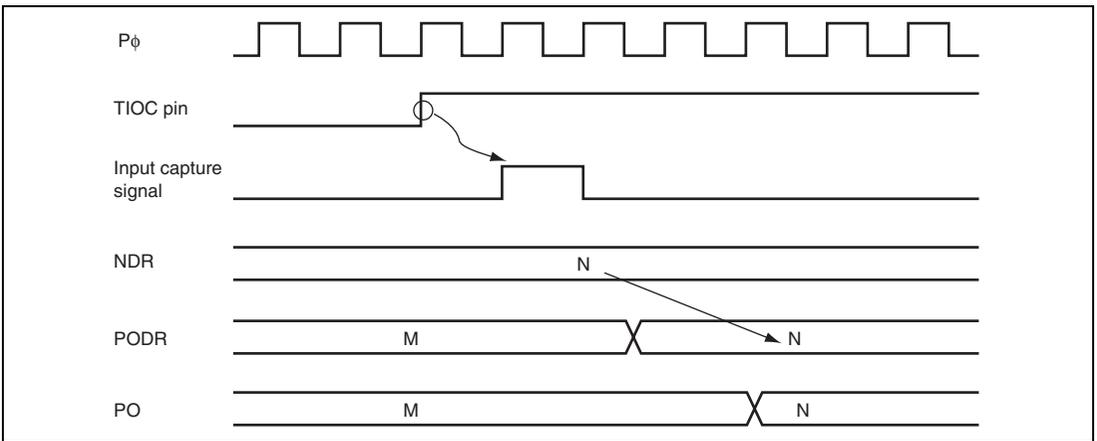
**Figure 15.14 Pulse Output Triggered by Input Capture (Example)**
