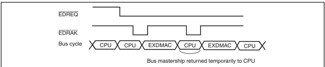
**Figure 11.13 Example of Timing in Cycle Steal Mode**
