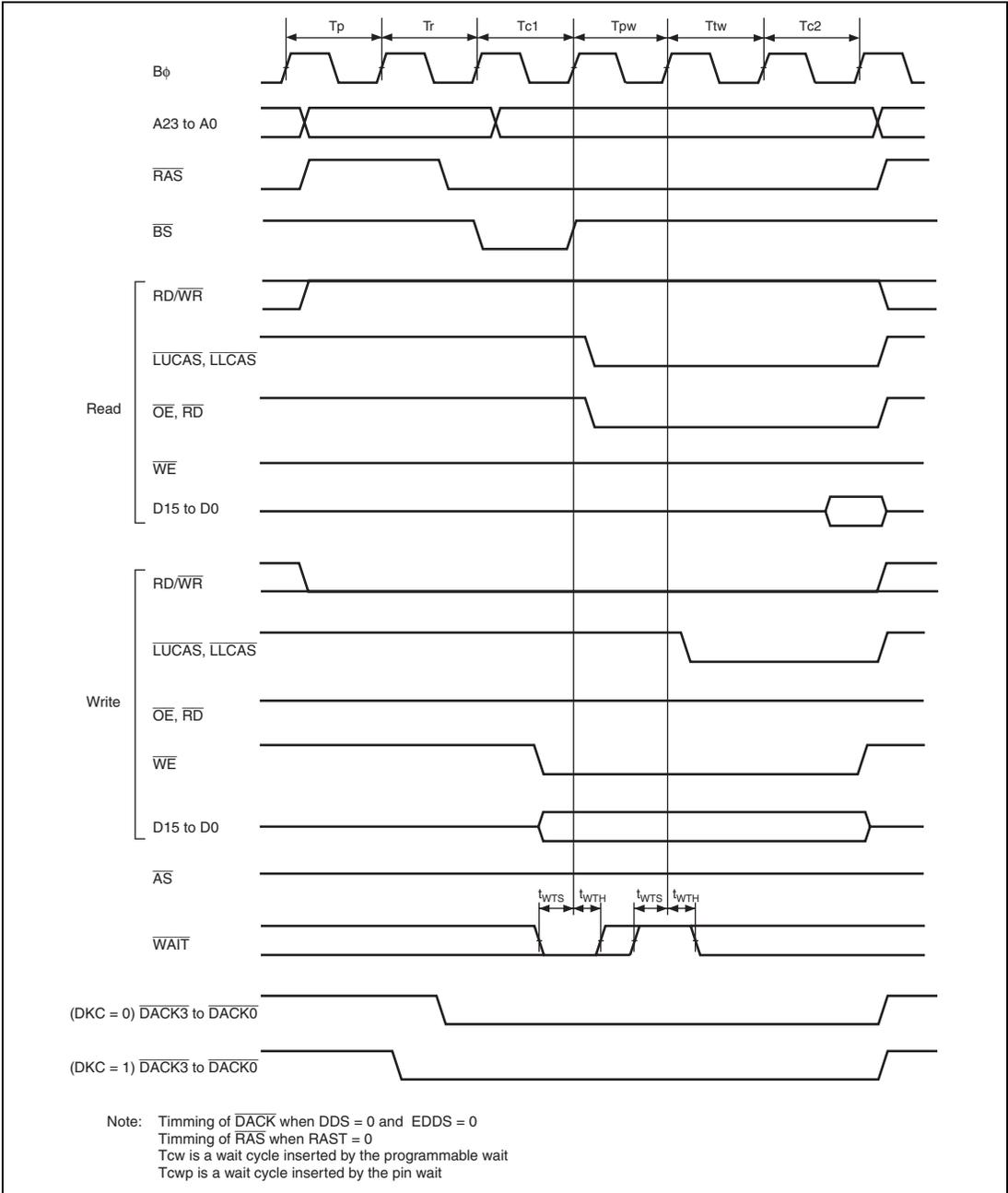
**Figure 29.20 DRAM Access Timing / Two-State Access, One Wait\***
