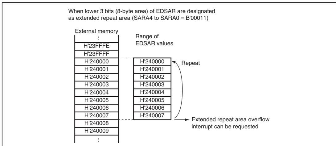
**Figure 11.15 Example of Extended Repeat Area Function Operation**
