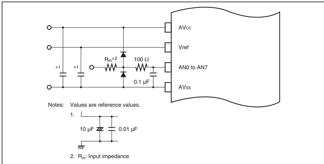
**Figure 21.14 Example of Analog Input Protection Circuit**
