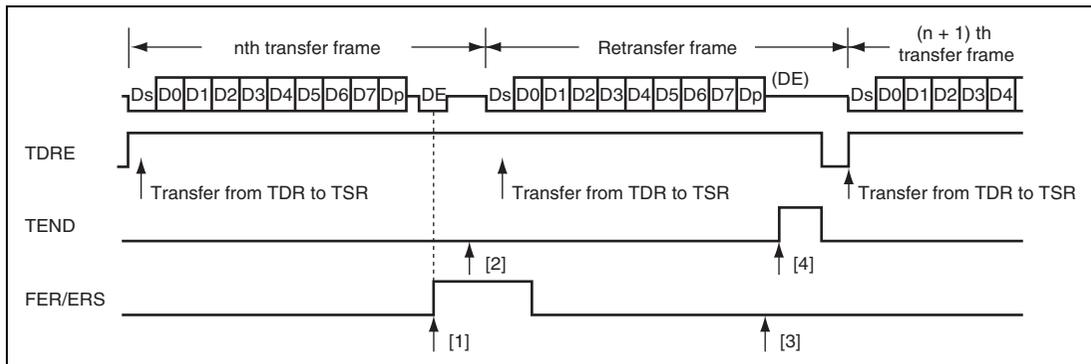
**Figure 19.29 Data Re-Transfer Operation in SCI Transmission Mode**
