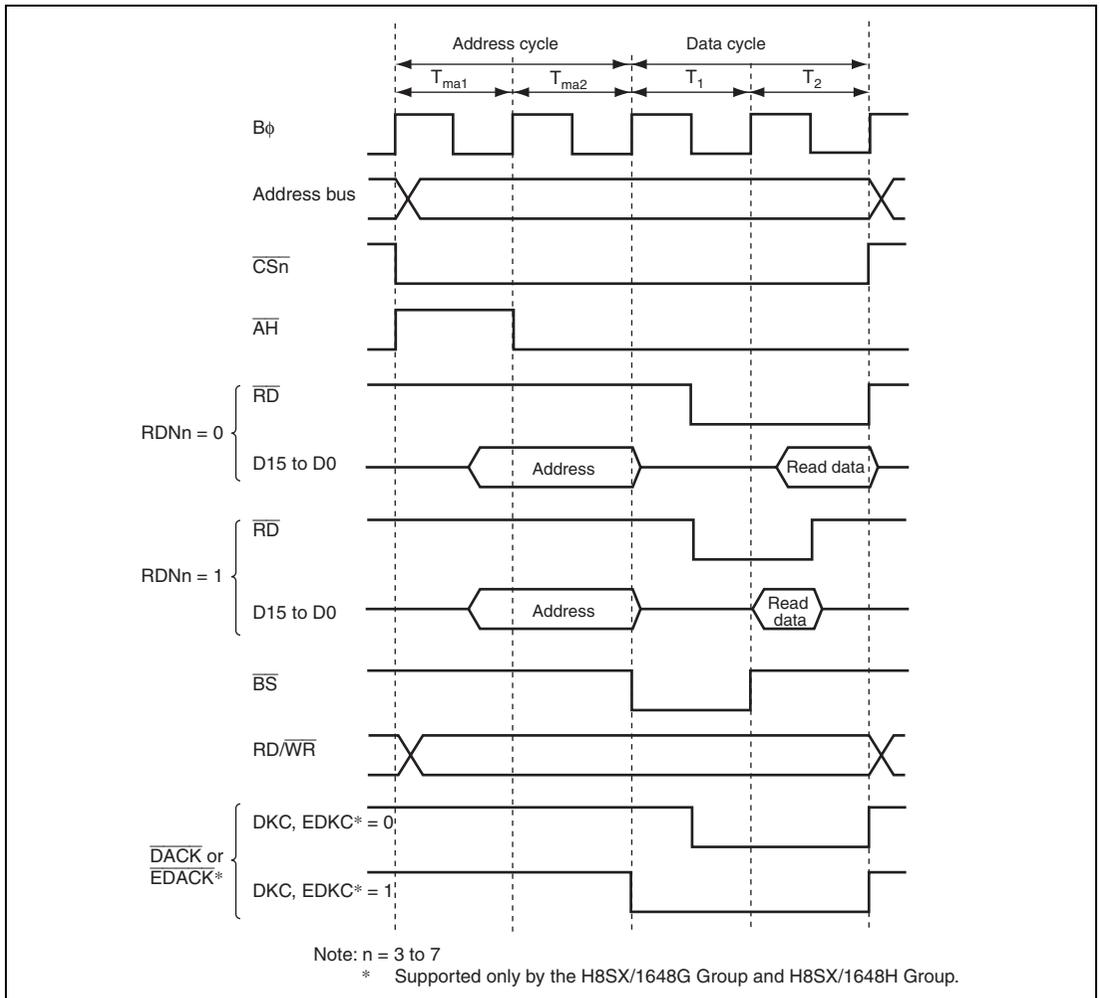
**Figure 9.37 Output Timing for  $\overline{\text{DACK}}$  and  $\overline{\text{EDACK}}^*$  Signals**
