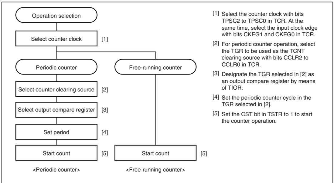
**Figure 14.3 Example of Counter Operation Setting Procedure**
