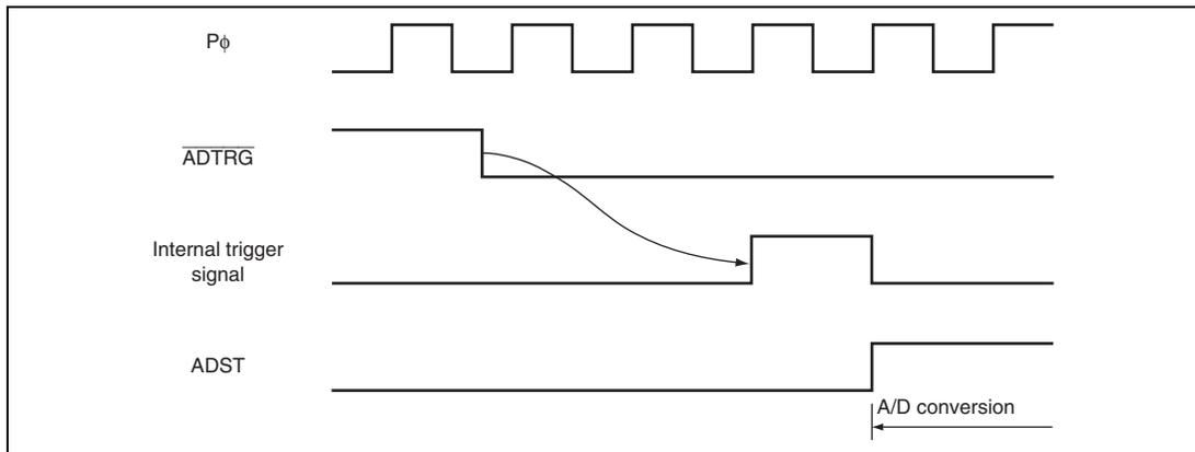
**Figure 21.8 External Trigger Input Timing (TRGS1, TRGS0, and EXTRGS  $\neq$  B'111)**
