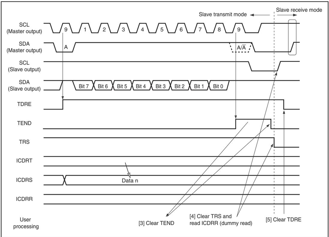
**Figure 20.10 Slave Transmit Mode Operation Timing 2**
