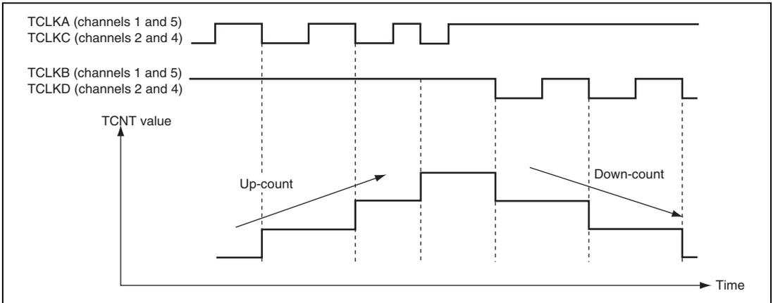
**Figure 14.28 Example of Phase Counting Mode 3 Operation**
