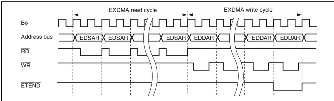
**Figure 11.54 Timing in Cluster Transfer Dual Address Mode**
