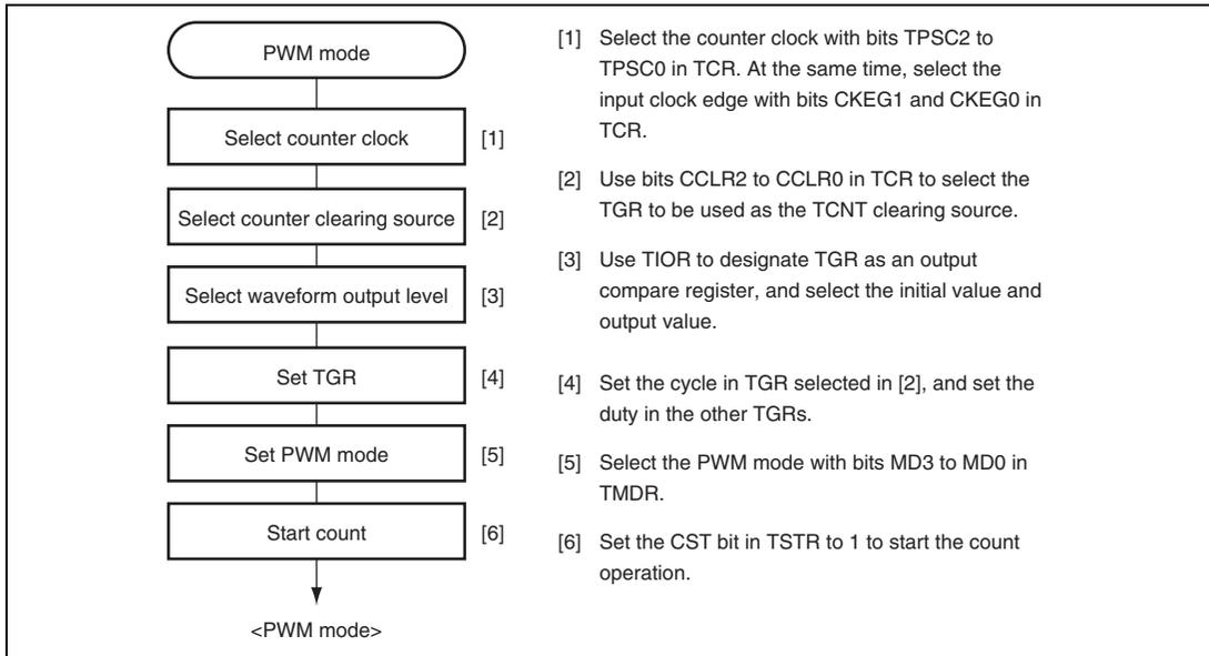
**Figure 14.21 Example of PWM Mode Setting Procedure**
