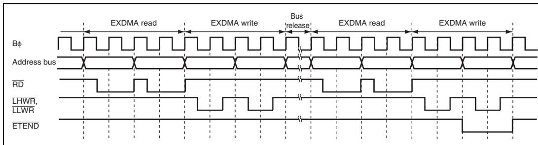
**Figure 11.61 Example of Cluster Transfer Mode Transfer**
