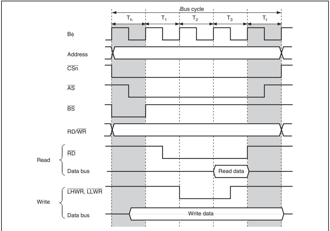
**Figure 9.3  $\overline{CS}$  and Address Assertion Period Extension**
