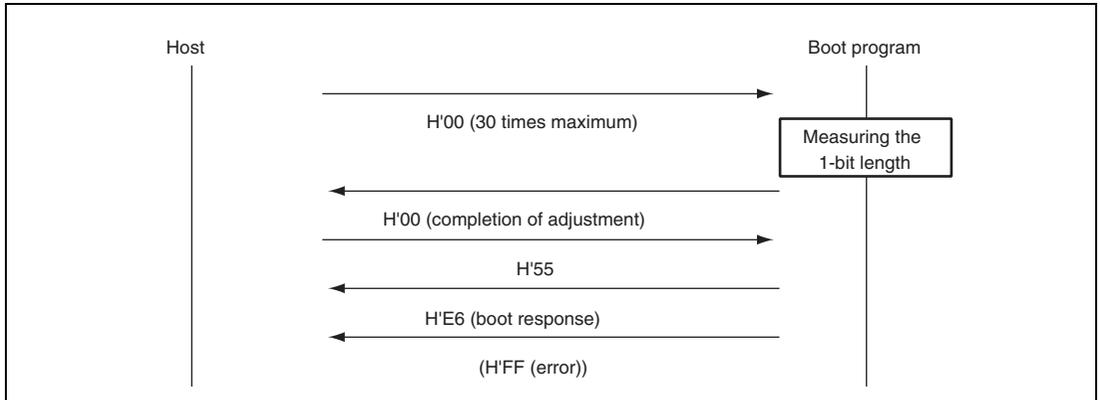
**Figure 24.22 Bit-Rate-Adjustment Sequence**
