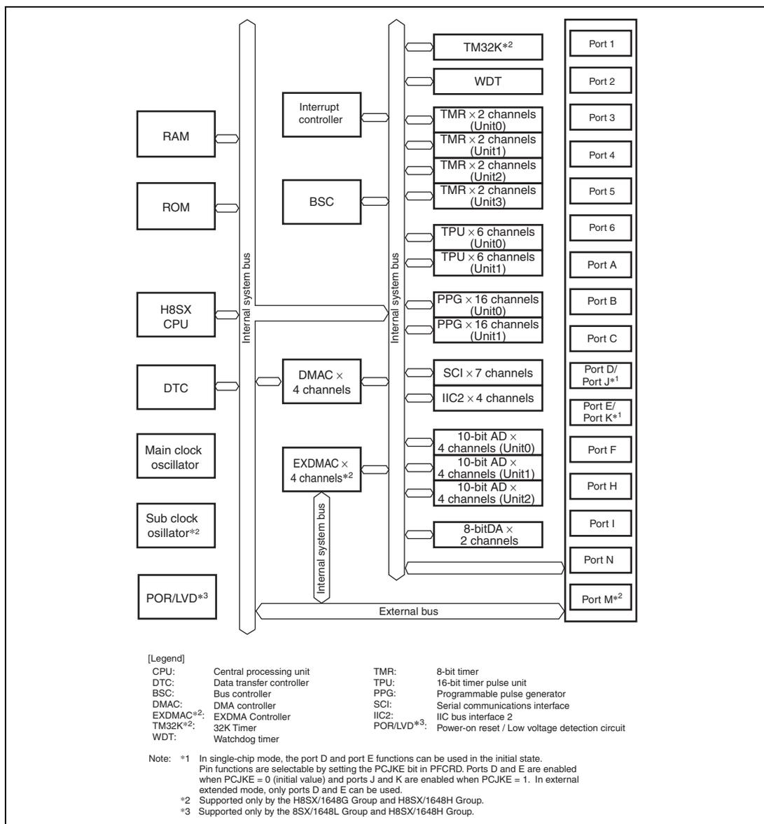
**Figure 1.2 Block Diagram**
