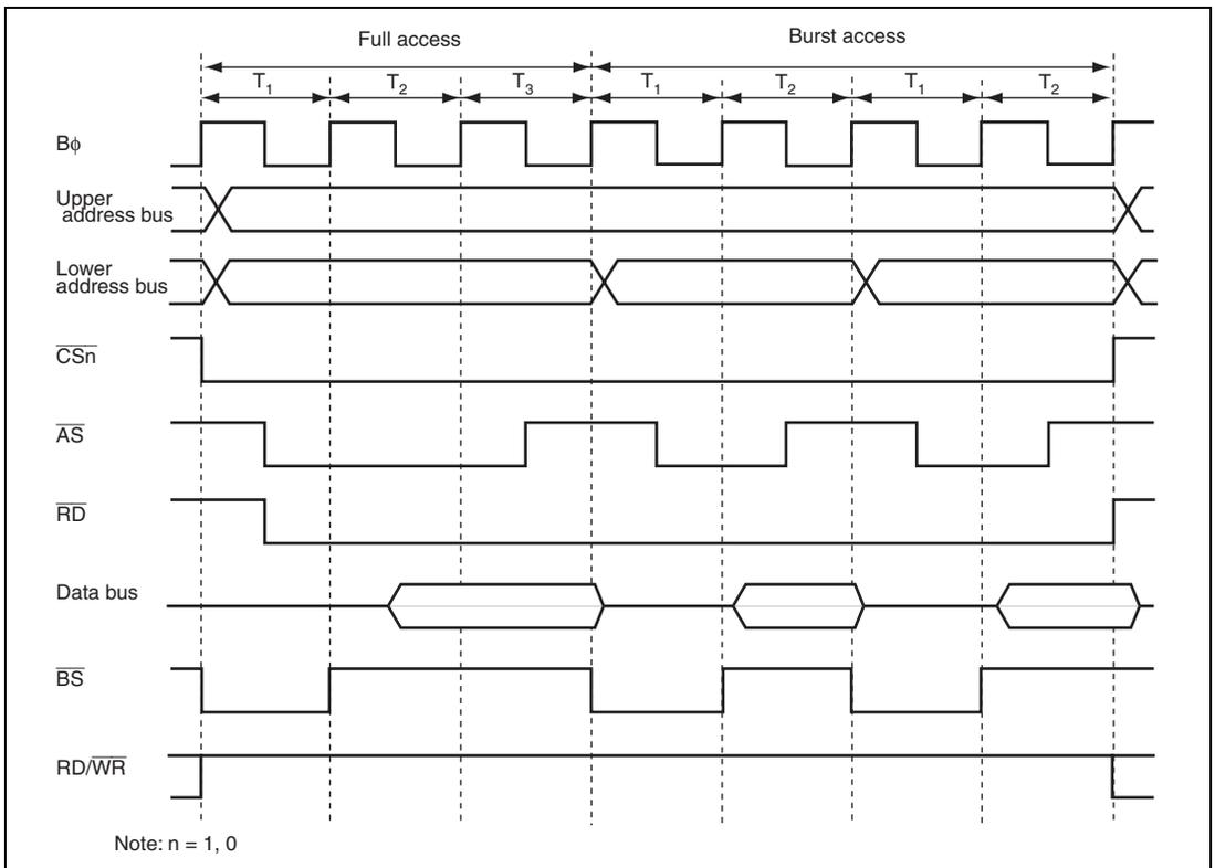
**Figure 9.29 Example of Burst ROM Access Timing (AST<sub>n</sub> = 1, Two Burst Cycles)**
