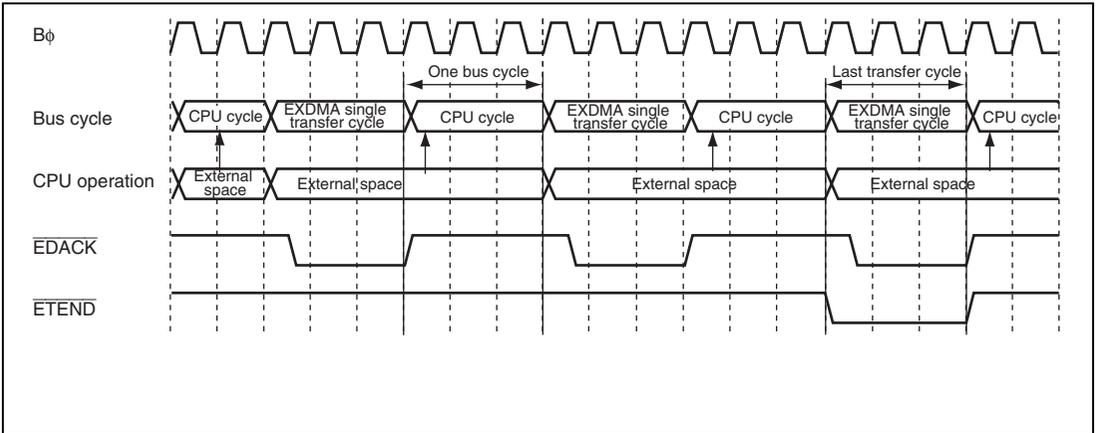
**Figure 11.40 Auto-Request/Normal Transfer Mode/Cycle Steal Mode
