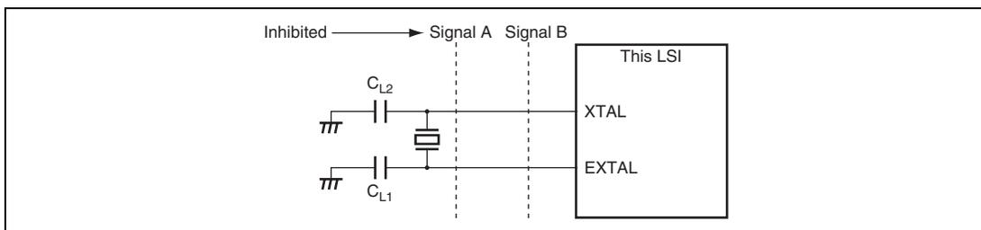
**Figure 26.10 Note on Board Design for Oscillation Circuit**
