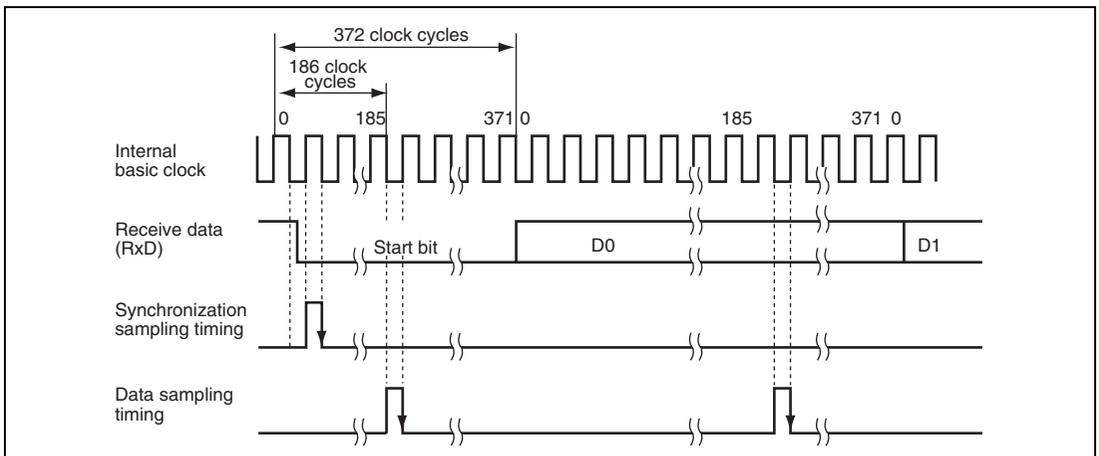
**Figure 19.28 Receive Data Sampling Timing in Smart Card Interface Mode (When Clock Frequency is 372 Times the Bit Rate)**
