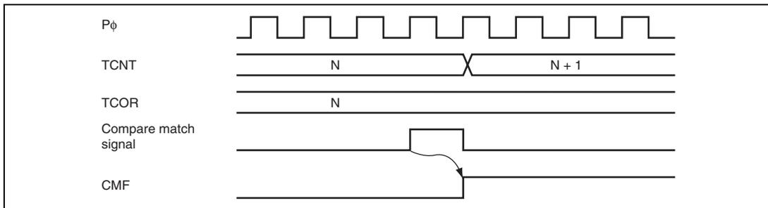
**Figure 16.9 Timing of CMF Setting at Compare Match**
