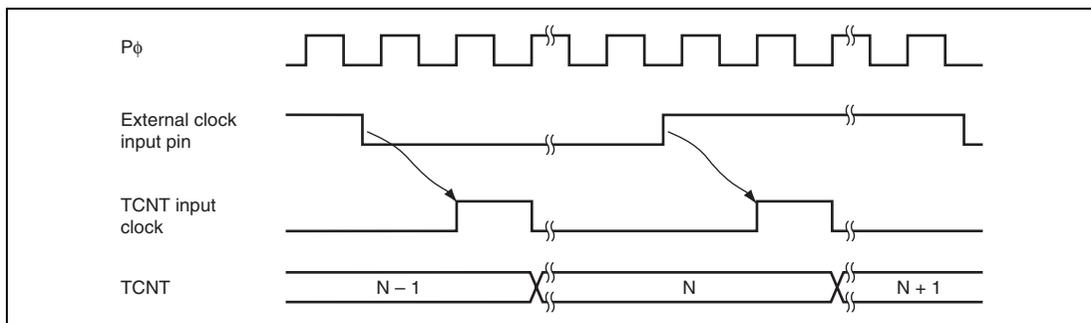
**Figure 16.8** Count Timing for External Clock Input
