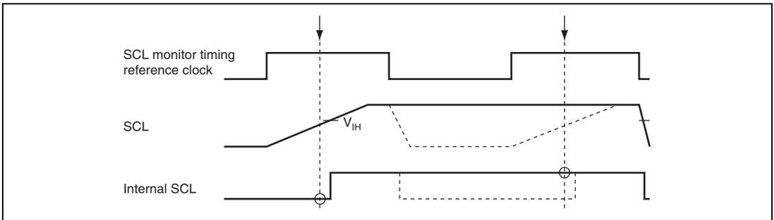
**Figure 20.18 Timing of the Bit Synchronous Circuit**
