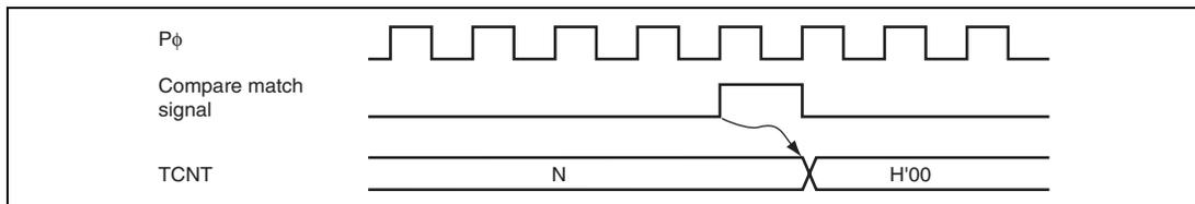
**Figure 16.11 Timing of Counter Clear by Compare Match**
