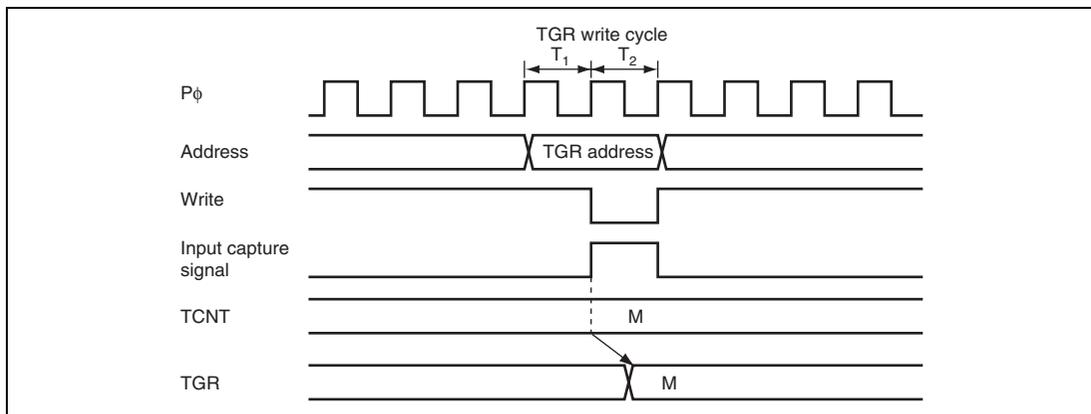
**Figure 14.52 Conflict between TGR Write and Input Capture**
