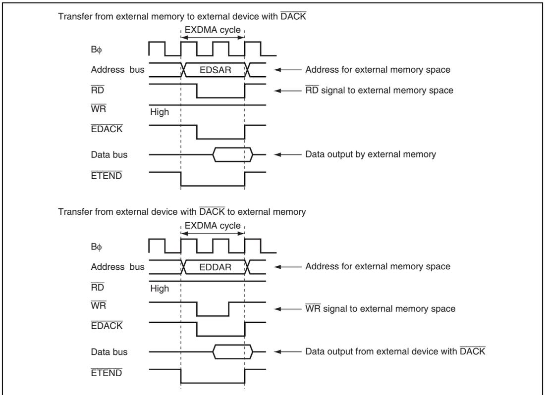
**Figure 11.5 Example of Timing in Single Address Mode**
