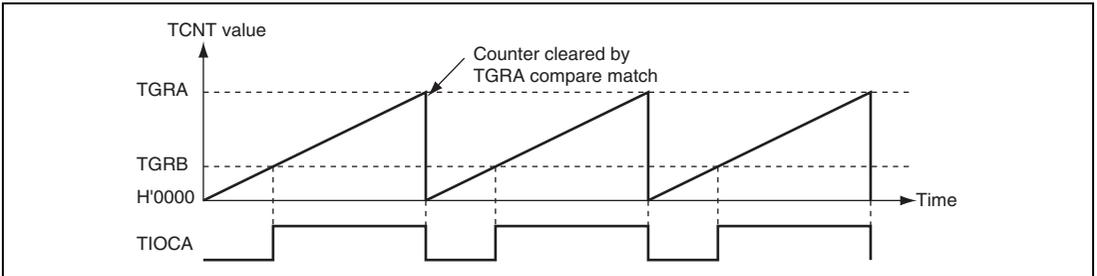
**Figure 14.22 Example of PWM Mode Operation (1)**
