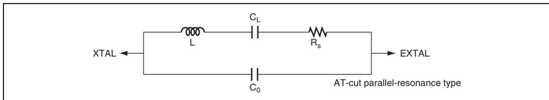
**Figure 26.3 Crystal Resonator Equivalent Circuit**
