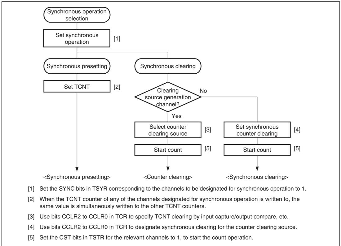
**Figure 14.11 Example of Synchronous Operation Setting Procedure**
