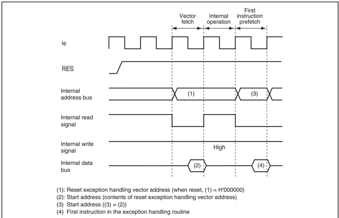
**Figure 6.1 Reset Sequence (On-chip ROM Enabled Advanced Mode)**
