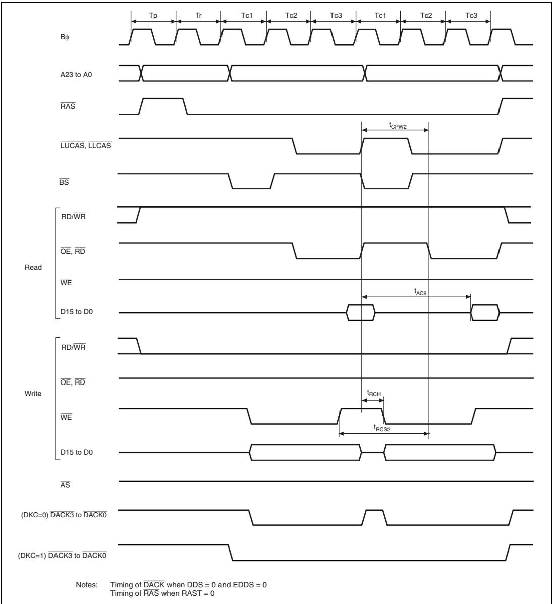
Figure 29.24 DRAM Access Timing / Three-State Burst Access\*
