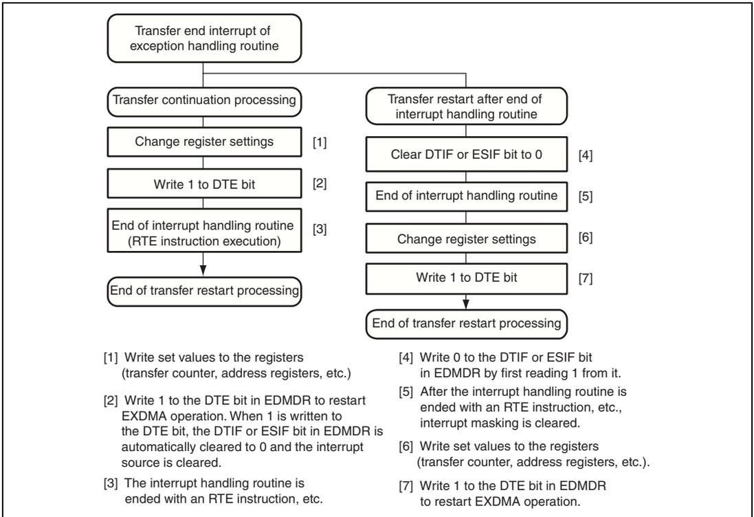
**Figure 11.71 Procedure for Clearing Transfer End Interrupt and Restarting Transfer**
