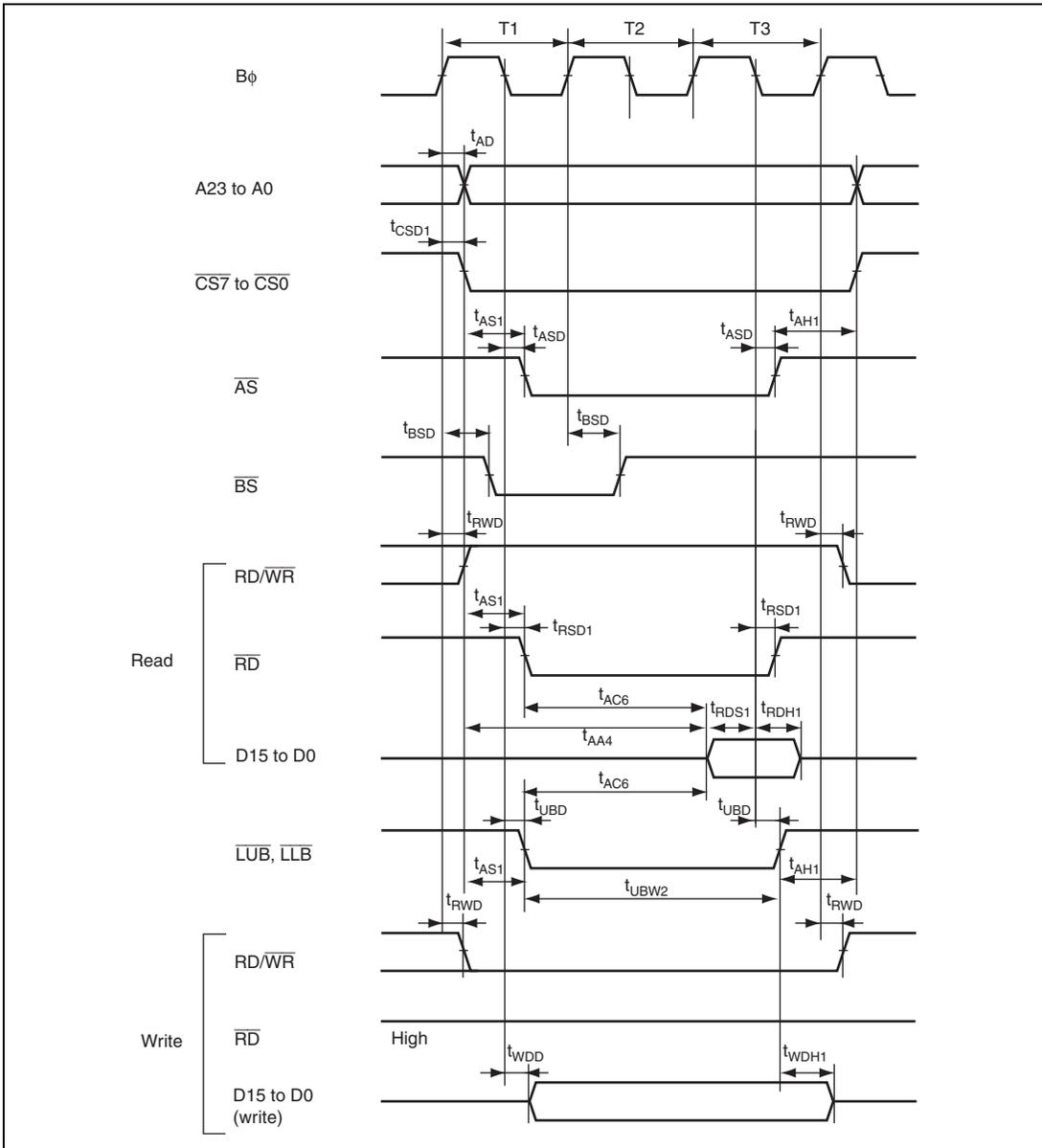
Figure 29.14 Byte Control SRAM: Three-State Read/Write Access
