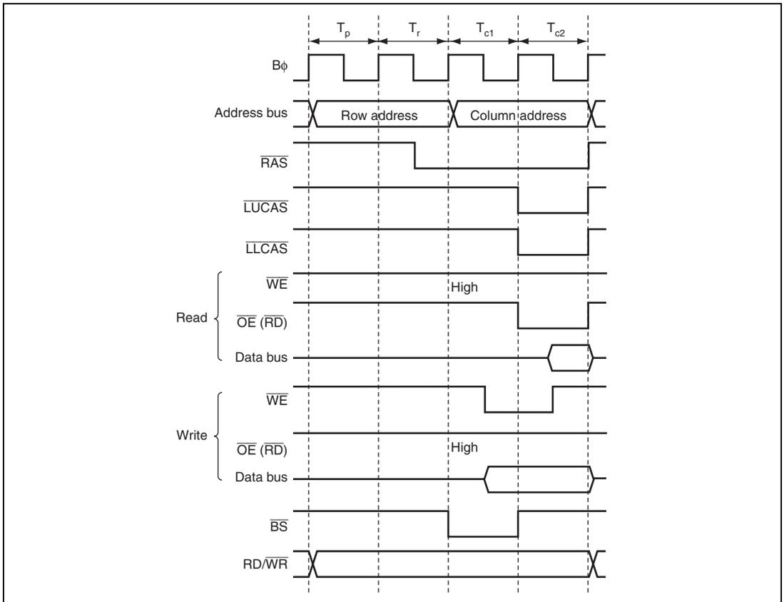
**Figure 9.38 DRAM Basic Access Timing (RAS = 0 and CAST = 0)**
