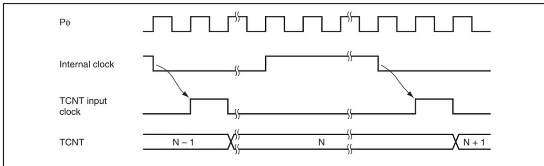
**Figure 16.7** Count Timing for Internal Clock Input
