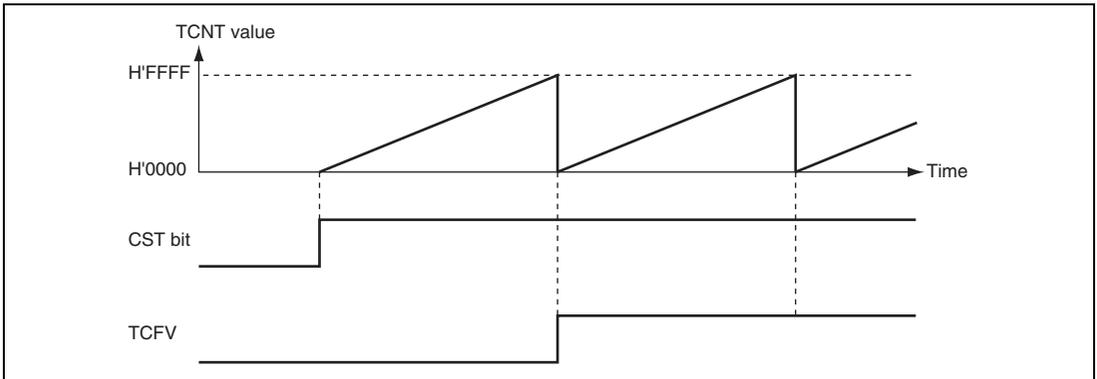
**Figure 14.4 Free-Running Counter Operation**
