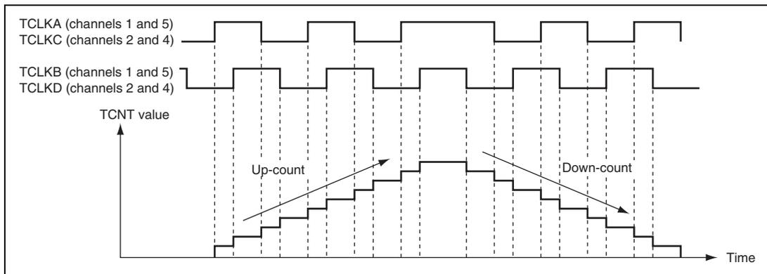
**Figure 14.26 Example of Phase Counting Mode 1 Operation**
