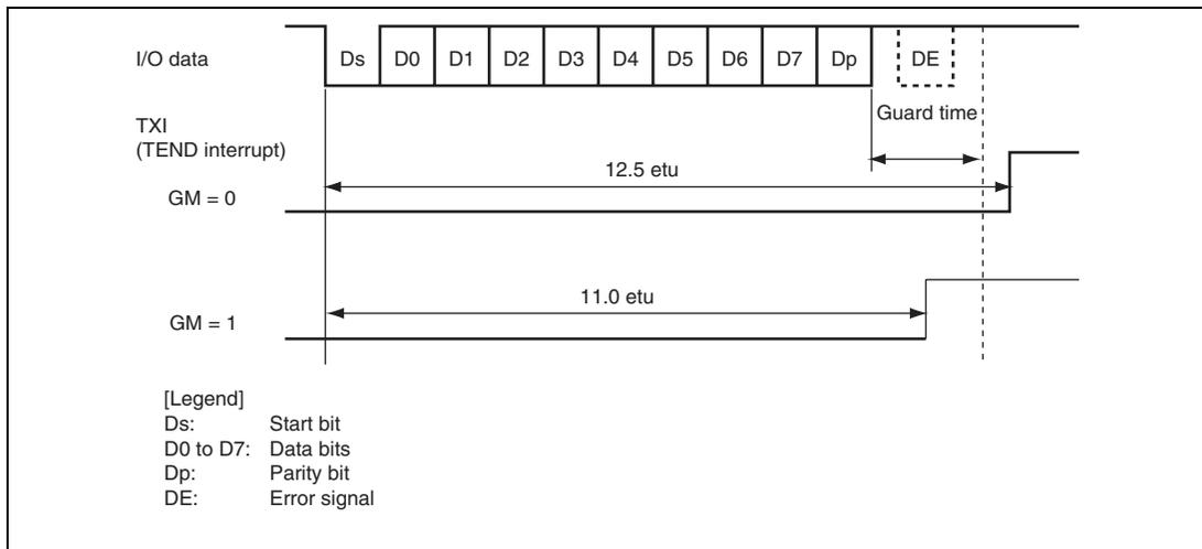
**Figure 19.30 TEND Flag Set Timing during Transmission**
