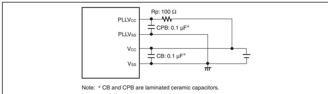
**Figure 26.11 Recommended External Circuitry for PLL Circuit**
