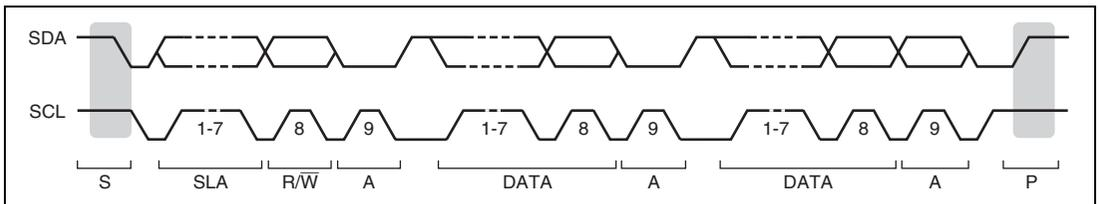
**Figure 20.4 I<sup>2</sup>C Bus Timing**
