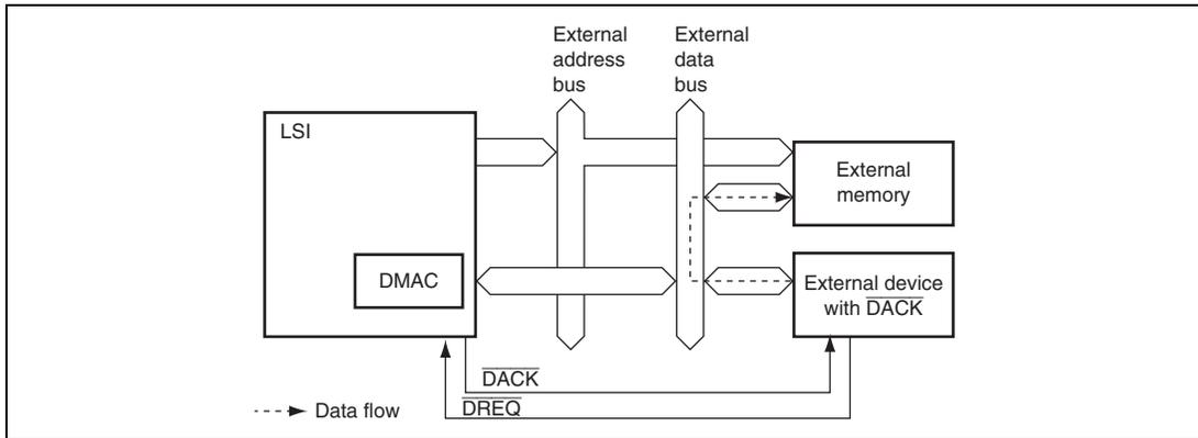
**Figure 10.4 Data Flow in Single Address Mode**
