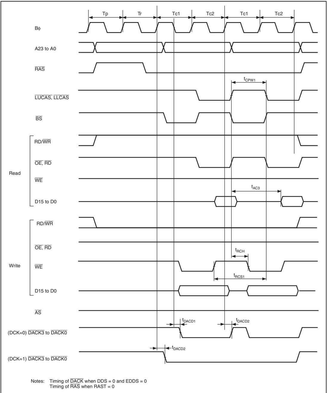
Figure 29.21 DRAM Access Timing / Two-State Burst Access\*
