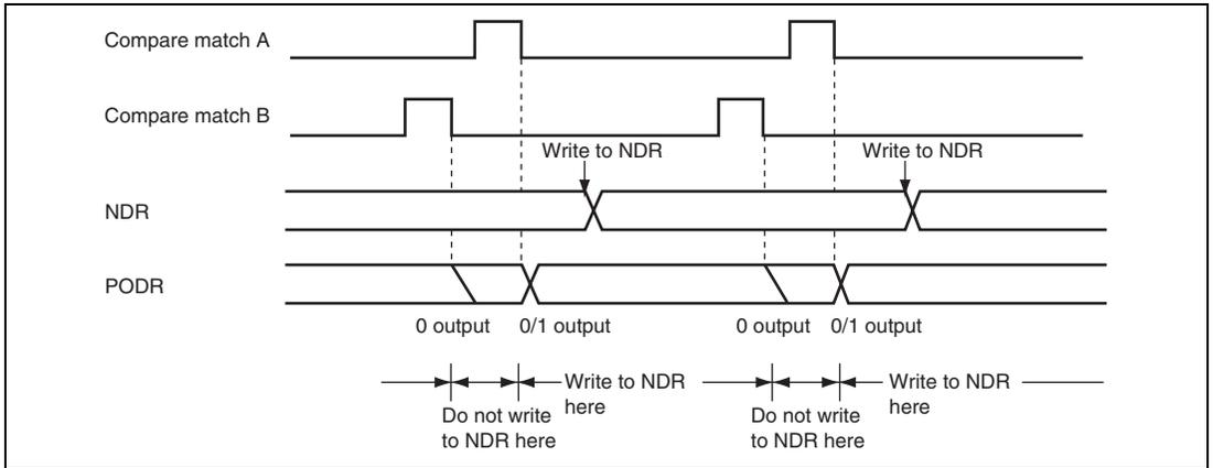
**Figure 15.9 Non-Overlapping Operation and NDR Write Timing**
