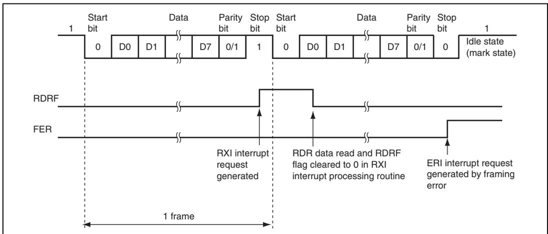
**Figure 19.11 Example of SCI Operation for Reception
