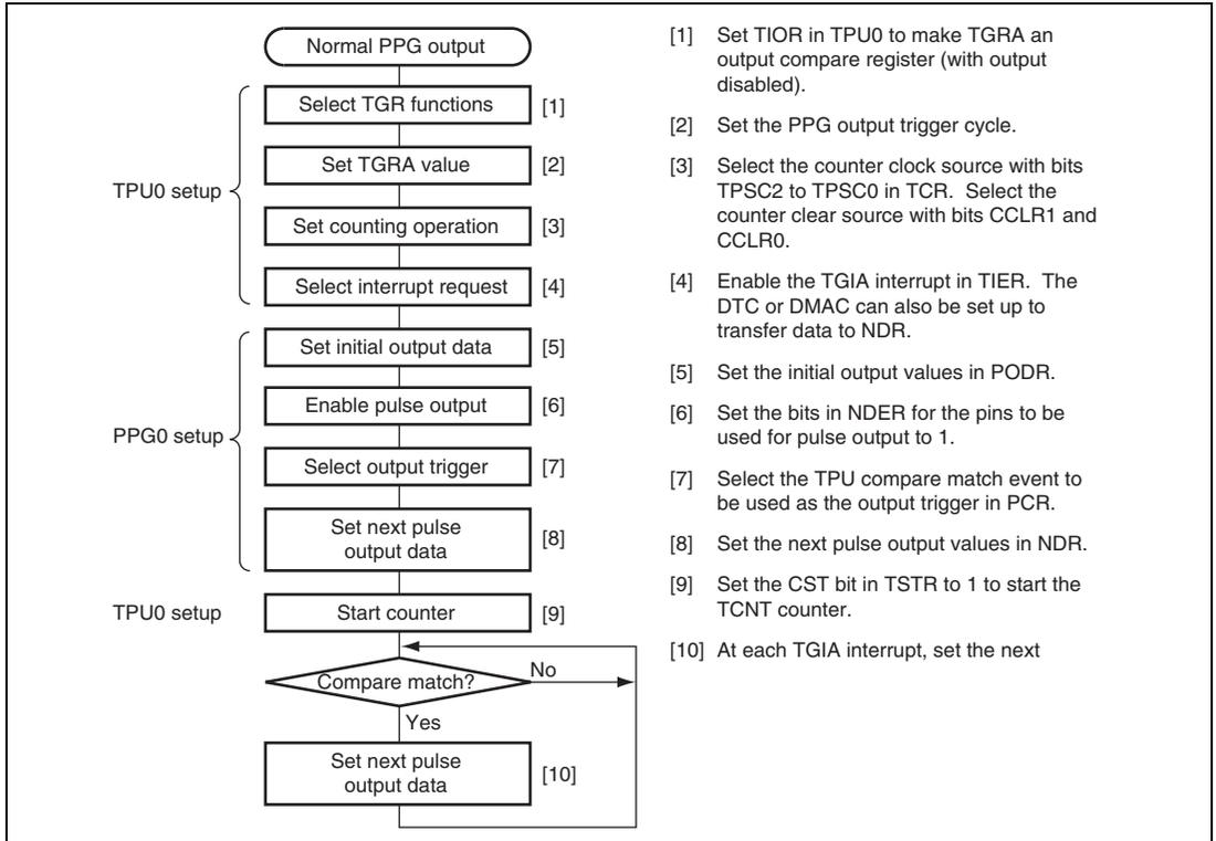
**Figure 15.5 Setup Procedure for Normal Pulse Output (PPG0)**
