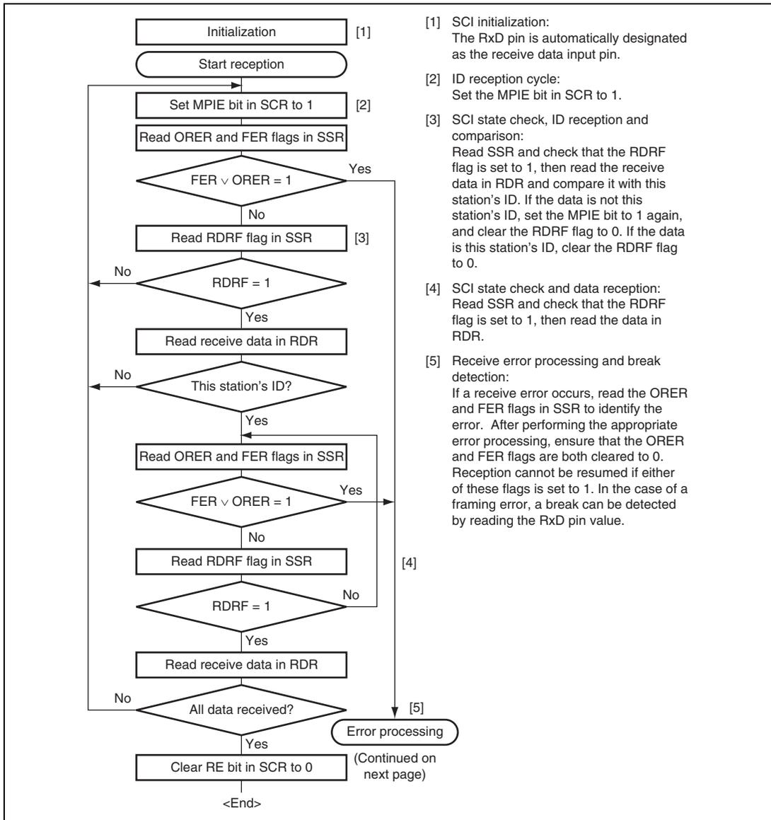
Figure 19.16 Sample Multiprocessor Serial Reception Flowchart (1)
