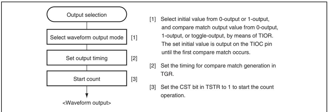
**Figure 14.6 Example of Setting Procedure for Waveform Output by Compare Match**
