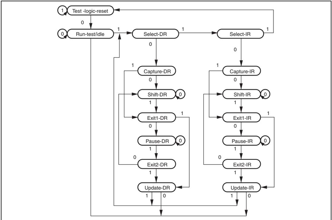
**Figure 25.2 State Transitions of the TAP Controller**
