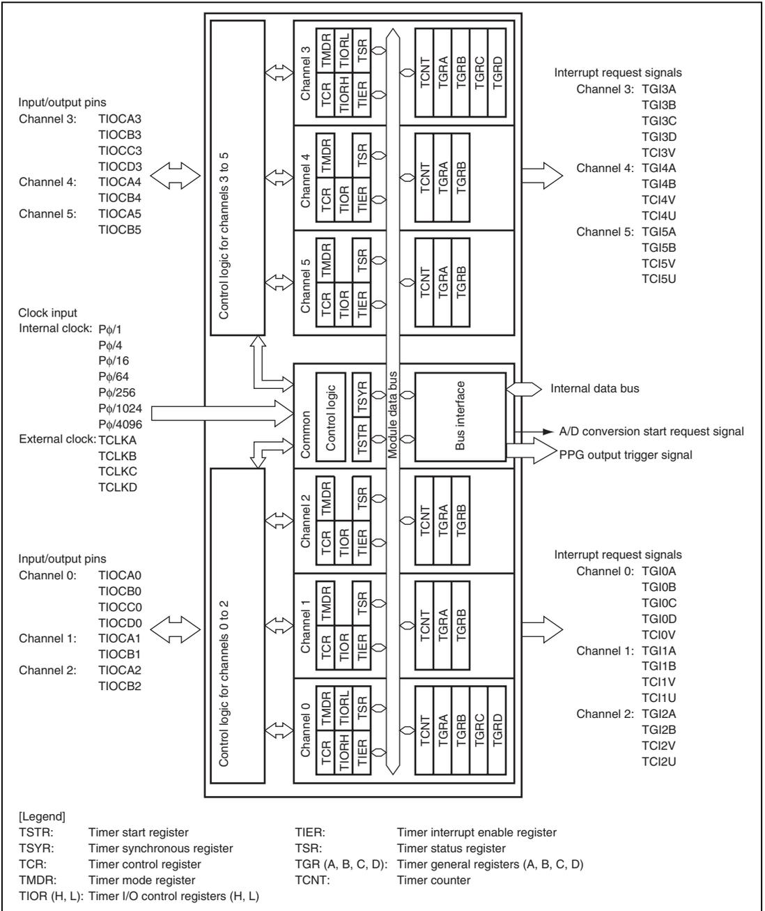
Figure 14.1 Block Diagram of TPU (Unit 0)
