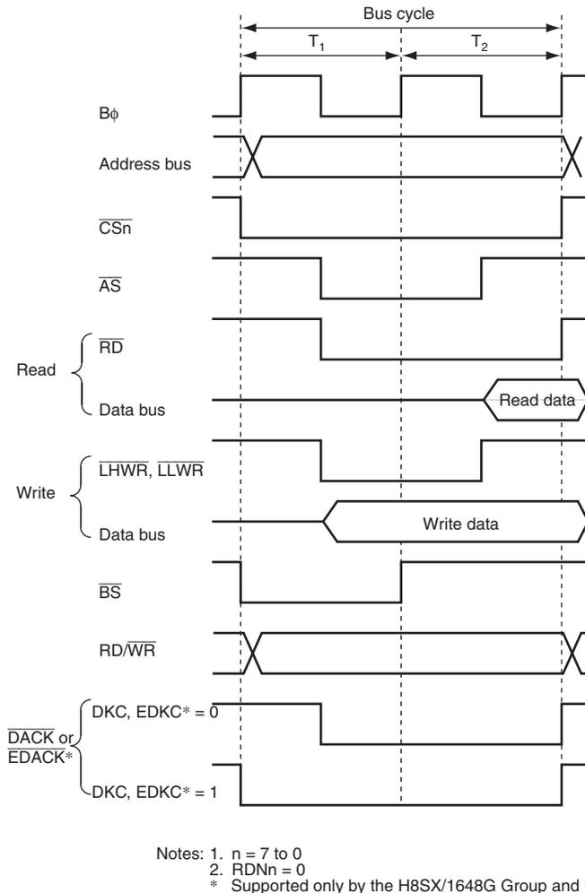
**Figure 9.24  $\overline{\text{DACK}}$  and  $\overline{\text{EDACK}}^*$  Signal Output Timing**
