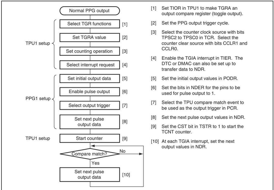
**Figure 15.6 Setup Procedure for Normal Pulse Output (PPG1)**
