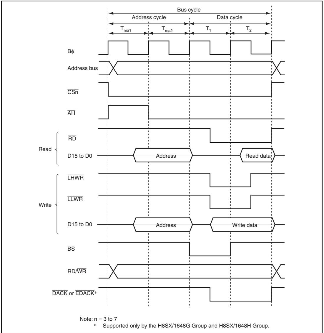
**Figure 9.32 16-Bit Access Space Access Timing (ABWHn = 0, ABWLn = 1)**
