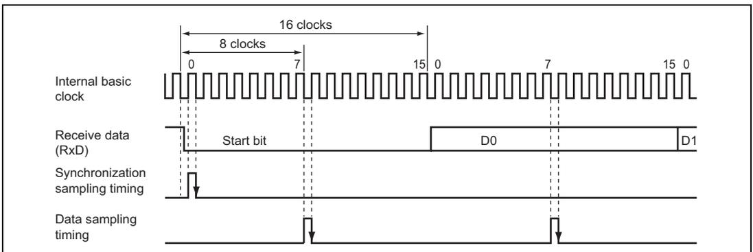
**Figure 19.6 Receive Data Sampling Timing in Asynchronous Mode**
