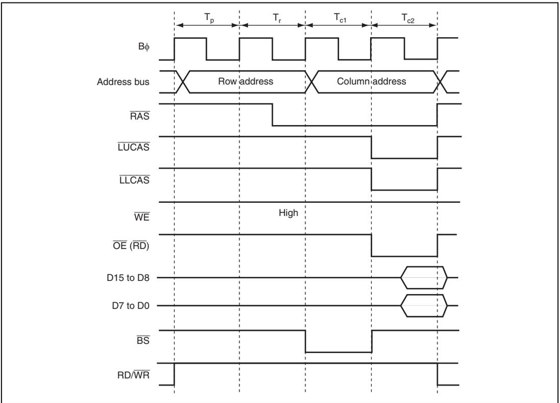
**Figure 9.46 Timing Example of Word Control with Use of Two CAS Signals
