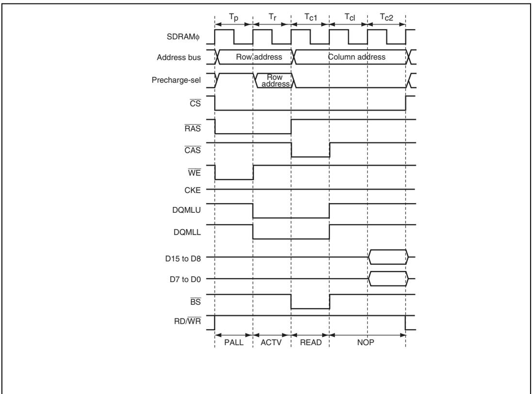
**Figure 9.60 SDRAM Basic Read Access Timing (CAS Latency = 2)**
