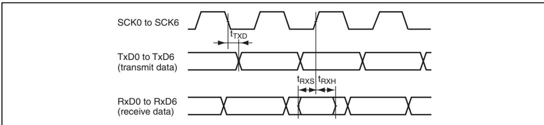
**Figure 29.51 SCI Input/Output Timing: Clocked Synchronous Mode**
