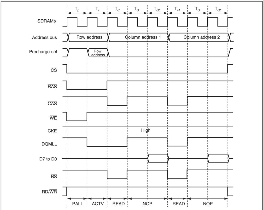
**Figure 9.73 Word Read Timing in 8-Bit Access Space
