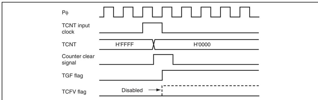
**Figure 14.54 Conflict between Overflow and Counter Clearing**
