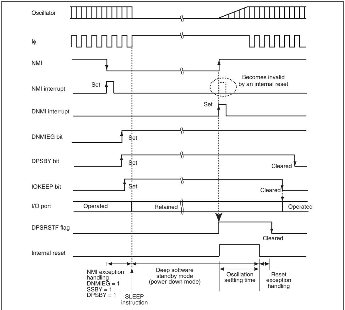
Figure 27.4 Deep Software Standby Mode Application Example (IOKEEP = 1)
