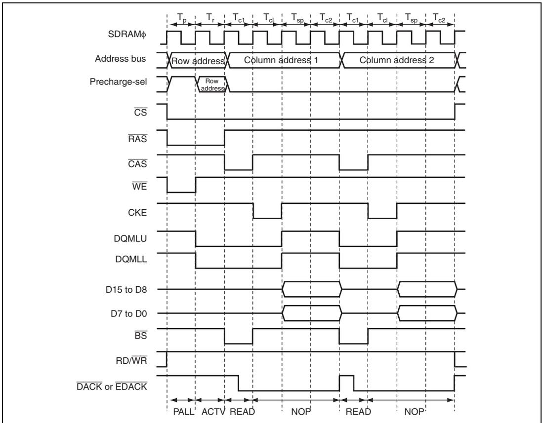
**Figure 9.88 Output Timing Example of  $\overline{\text{DACK}}$  and  $\overline{\text{EDACK}}$  when CKSPE = 1
