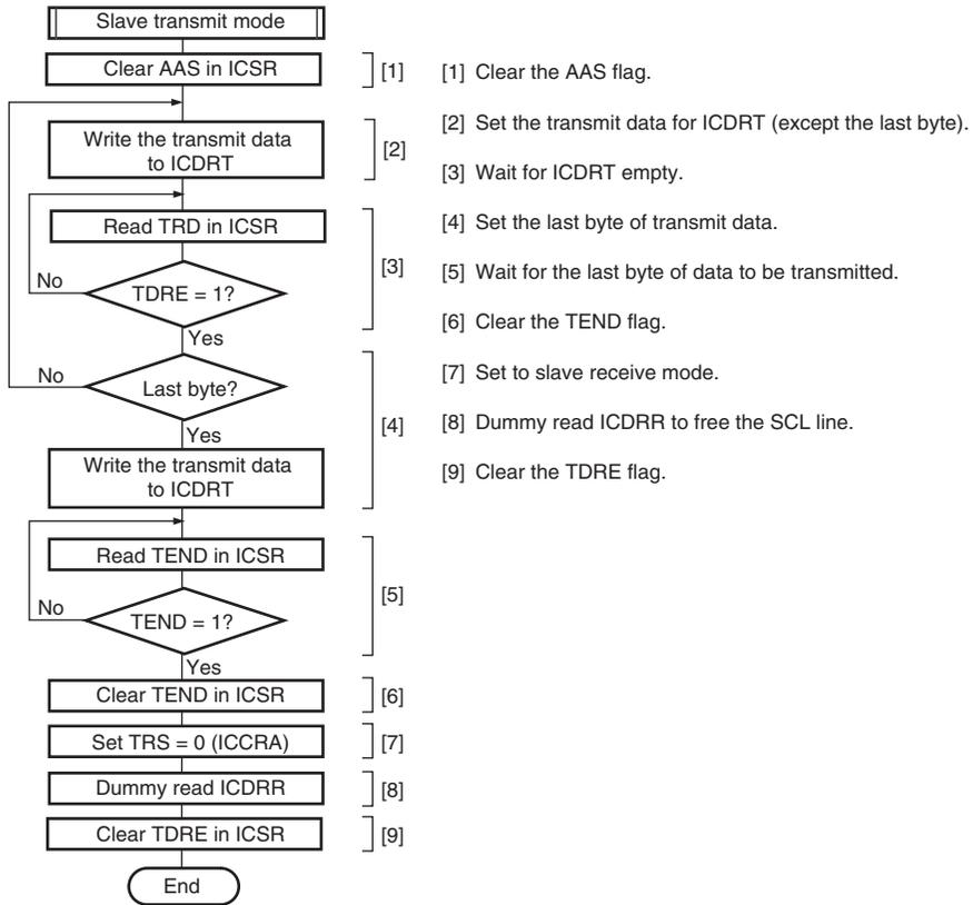
**Figure 20.16 Sample Flowchart for Slave Transmit Mode**
