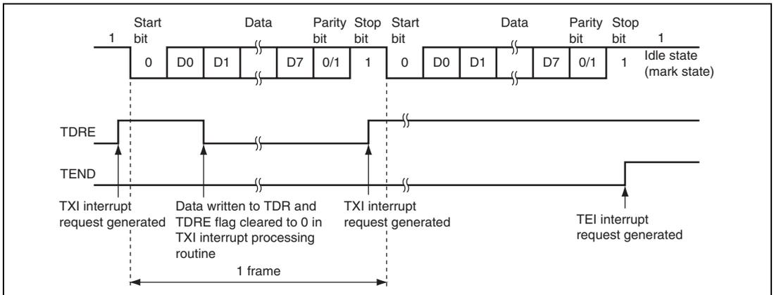
**Figure 19.9 Example of Operation for Transmission in Asynchronous Mode
