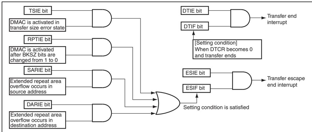
Figure 10.39 Interrupt and Interrupt Sources
