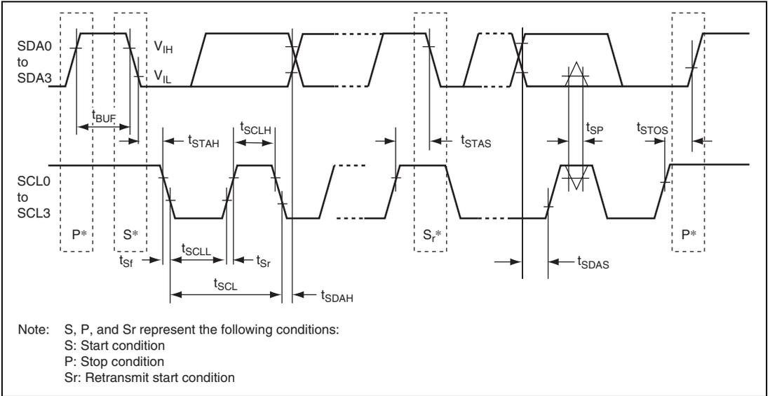
**Figure 29.53 I<sup>2</sup>C Bus Interface 2 Input/Output Timing (Option)**
