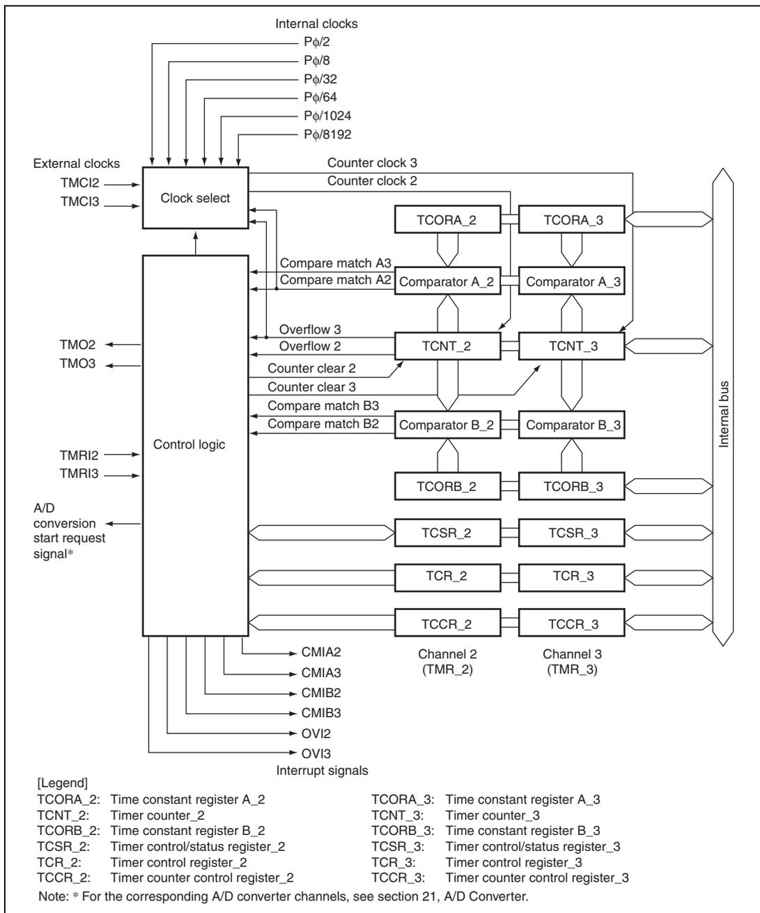
**Figure 16.2 Block Diagram of 8-Bit Timer Module (Unit 1)**
