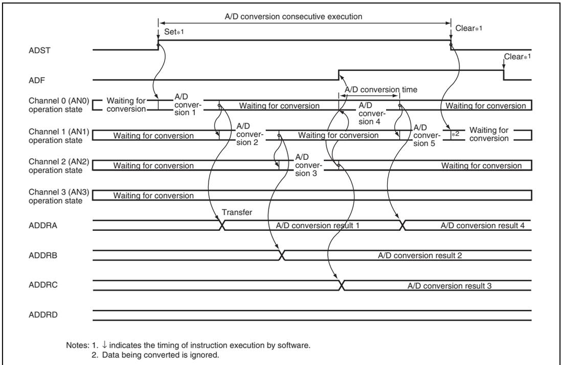
**Figure 21.5 Example of A/D Conversion
