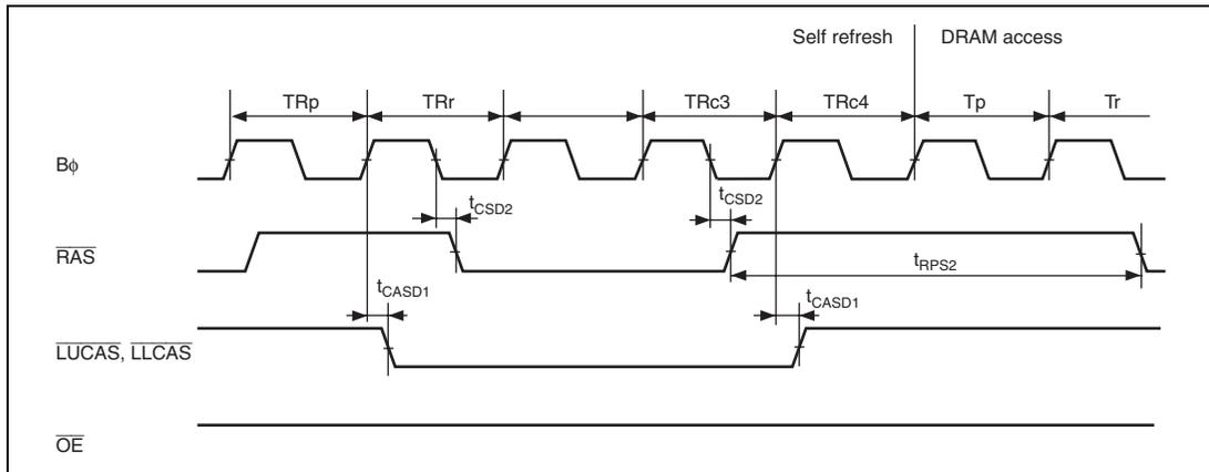
Figure 29.27 Self-Refresh Timing (After Leaving Software Standby: RAST=0)\*
