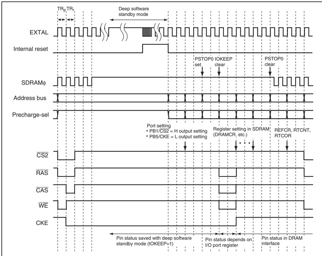
**Figure 9.81 Self-Refresh Timing in Deep Software Standby Mode**
