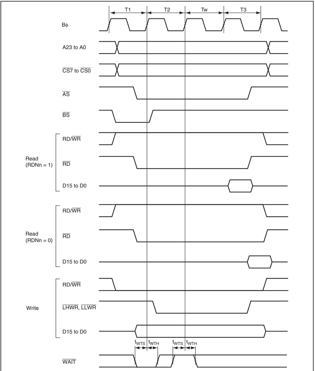
**Figure 29.10 Basic Bus Timing: Three-State Access, One Wait**
