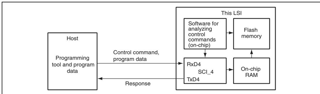
**Figure 24.6 System Configuration in Boot Mode**
