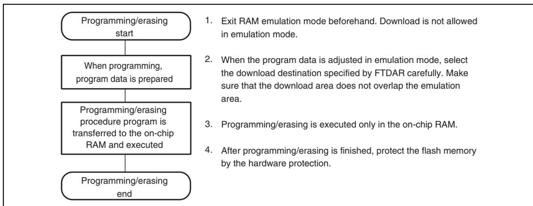
**Figure 24.9 Programming/Erasing Flow**
