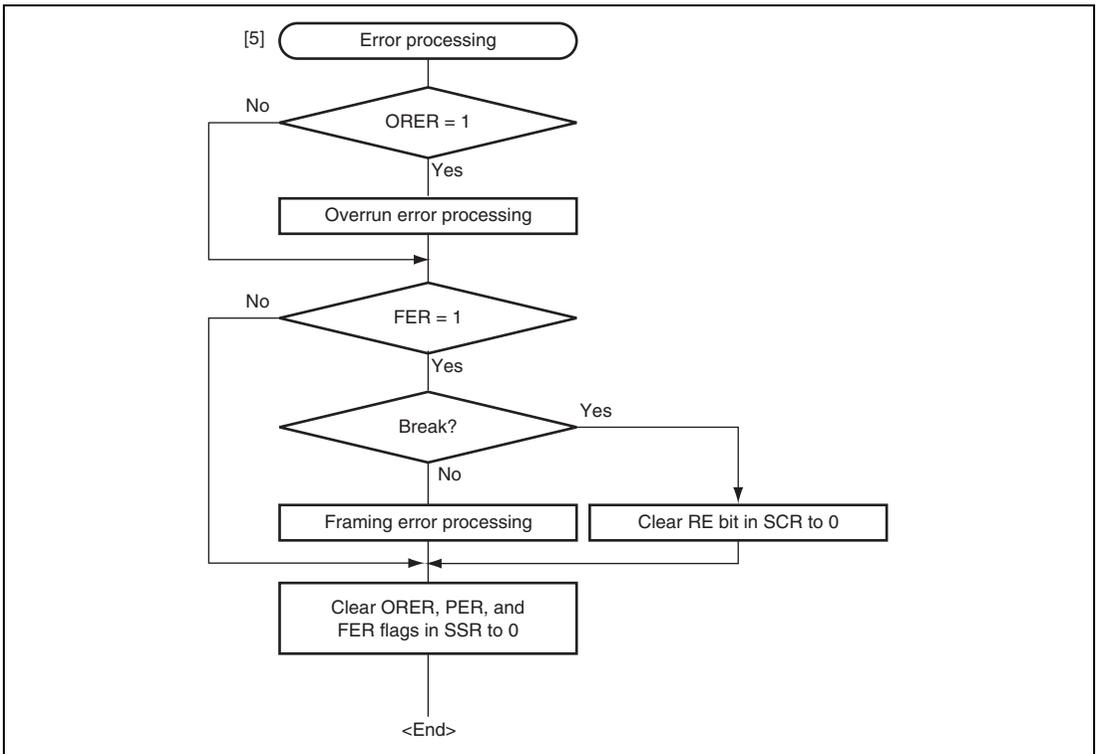
**Figure 19.16 Sample Multiprocessor Serial Reception Flowchart (2)**
