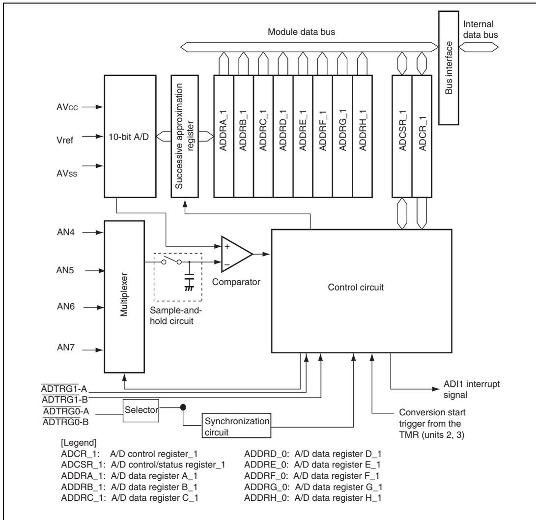
**Figure 21.2 Block Diagram of A/D Converter Unit 1 (AD\_1)**
