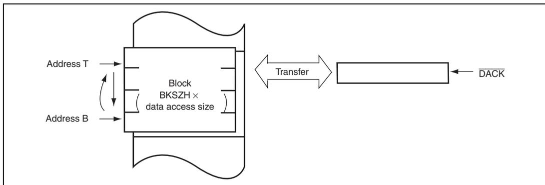
**Figure 10.11 Operation in Single Address Mode in Block Transfer Mode
