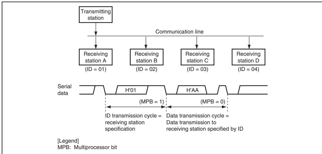
**Figure 19.13 Example of Communication Using Multiprocessor Format
