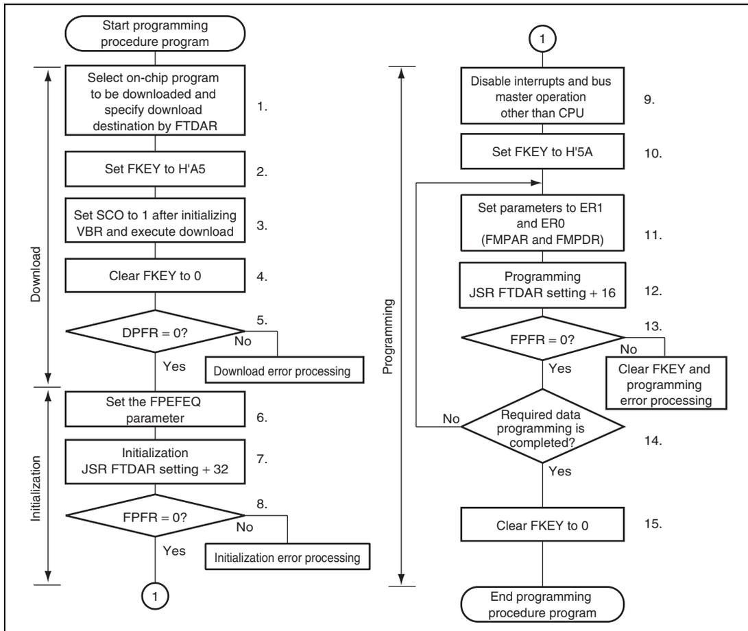
**Figure 24.11 Programming Procedure in User Program Mode**
