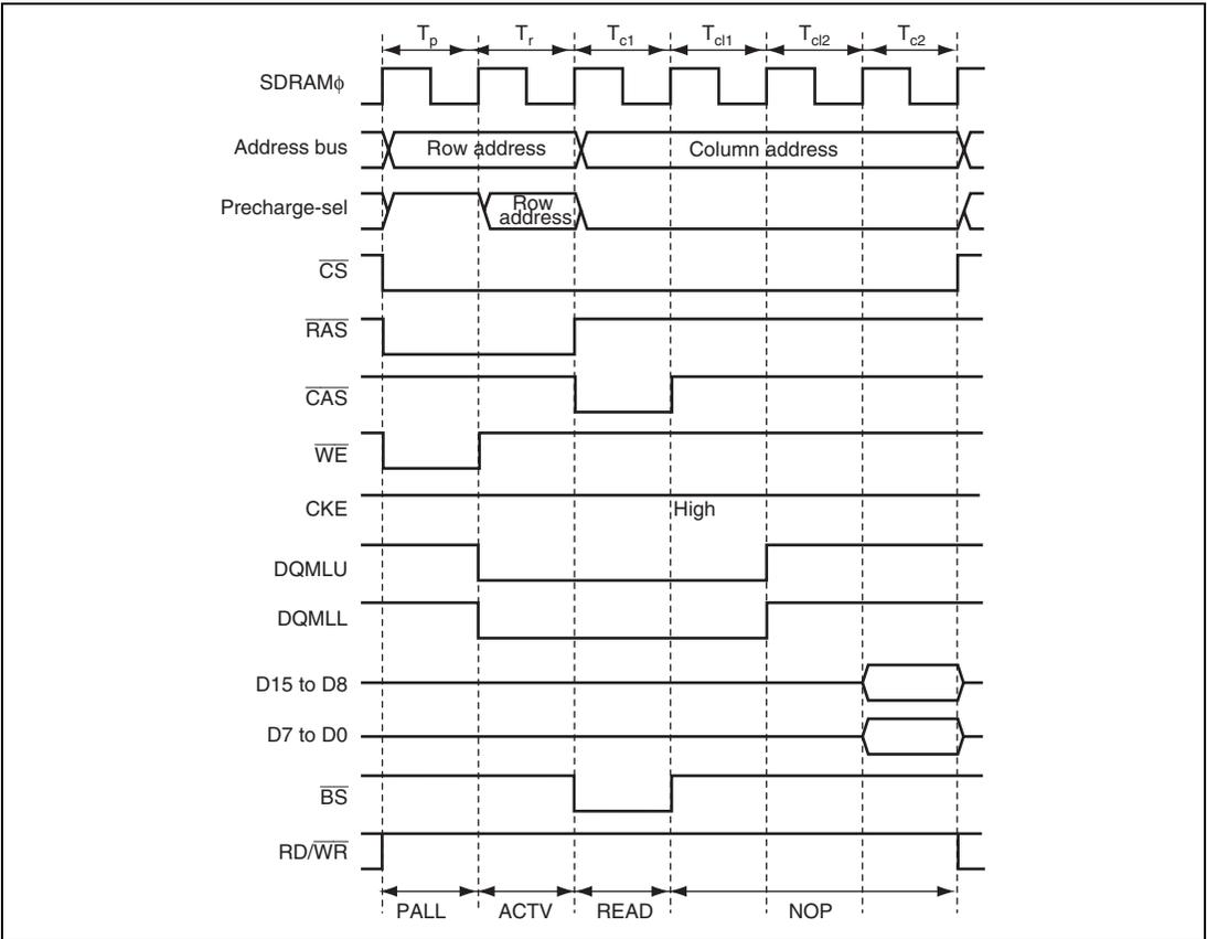
**Figure 9.62 Timing Example of CAS Latency (CAS Latency = 3)**
