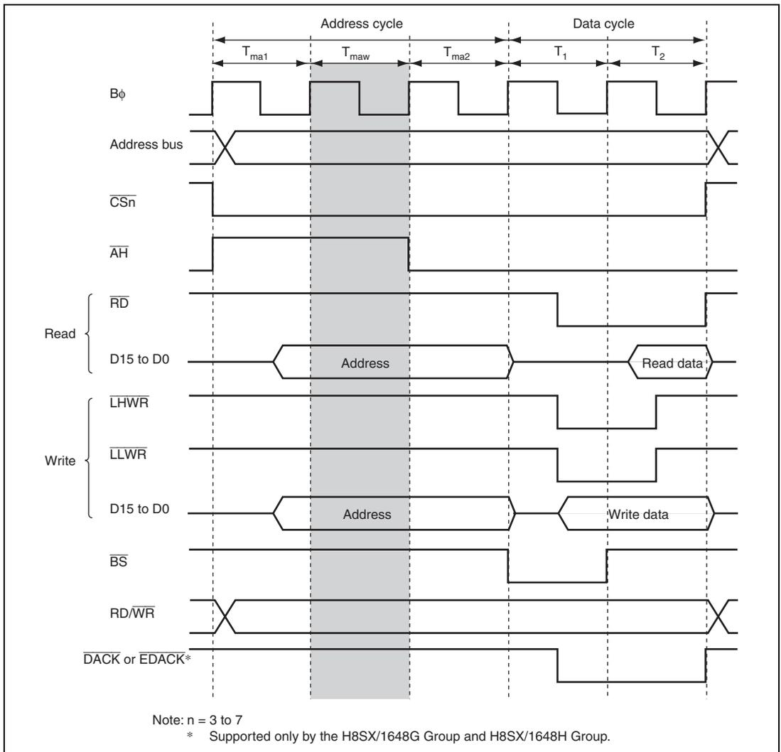
**Figure 9.33 Access Timing of 3 Address Cycles (ADDEX = 1)**
