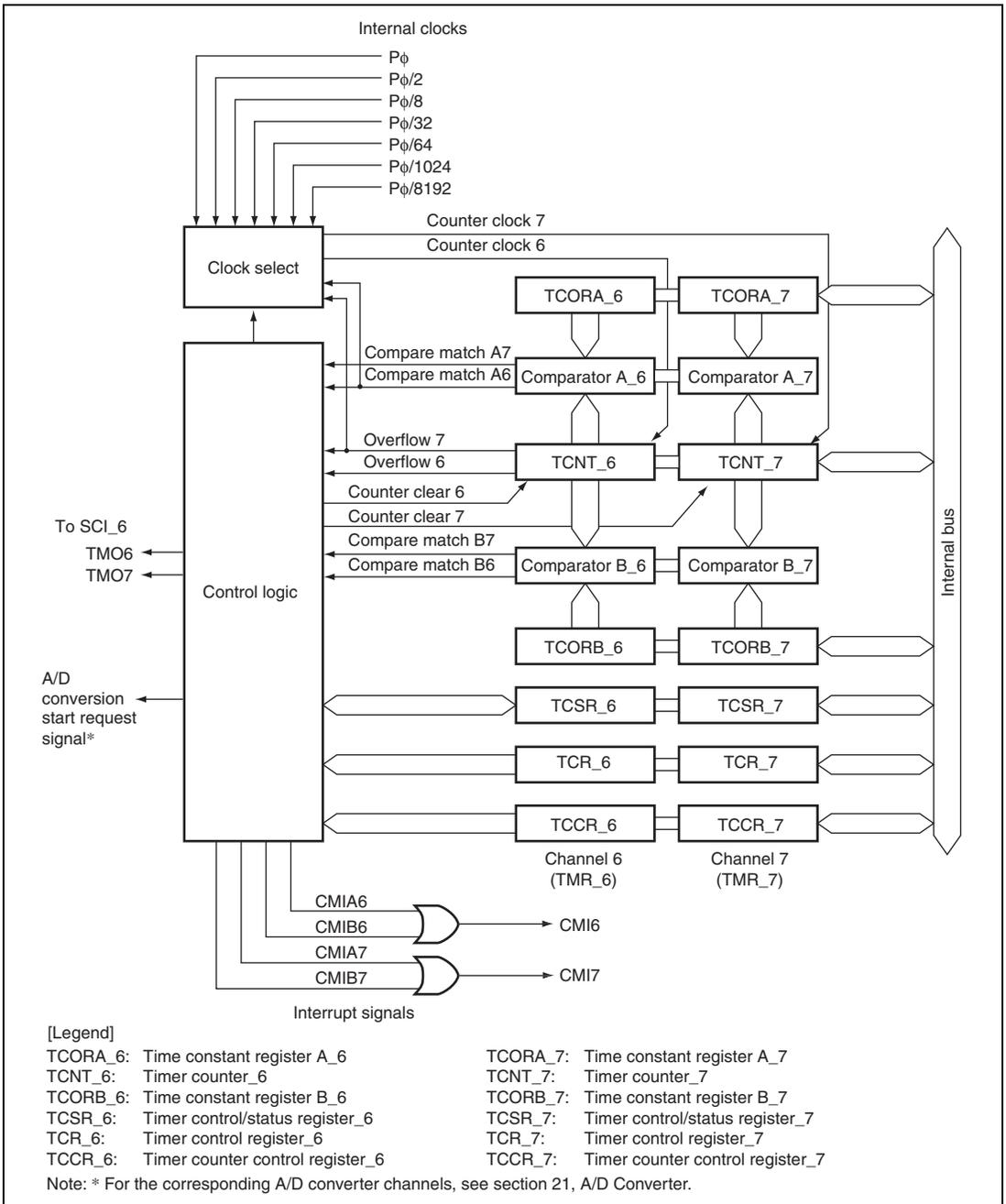
**Figure 16.4 Block Diagram of 8-Bit Timer Module (Unit 3)**
