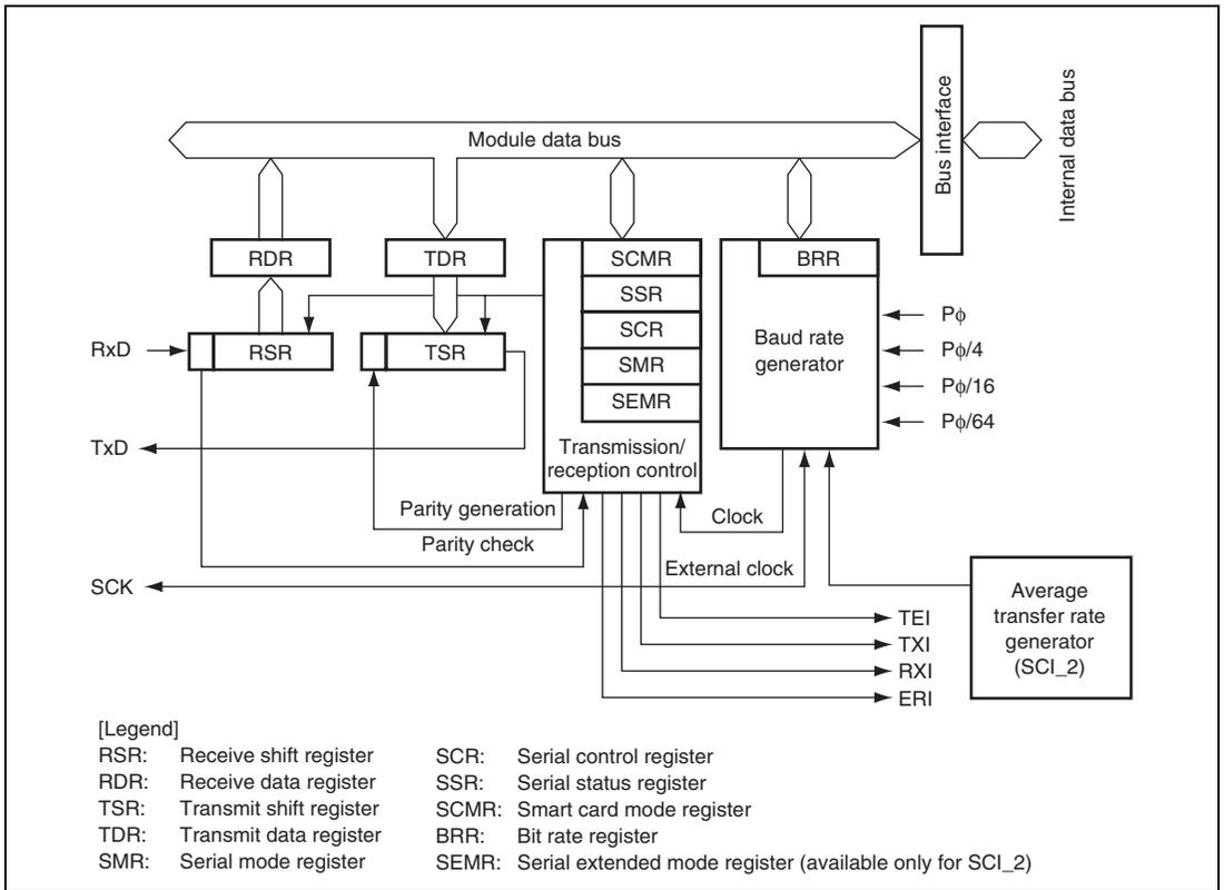
**Figure 19.1 Block Diagram of SCI\_0, 1, 2, 3, and 4**
