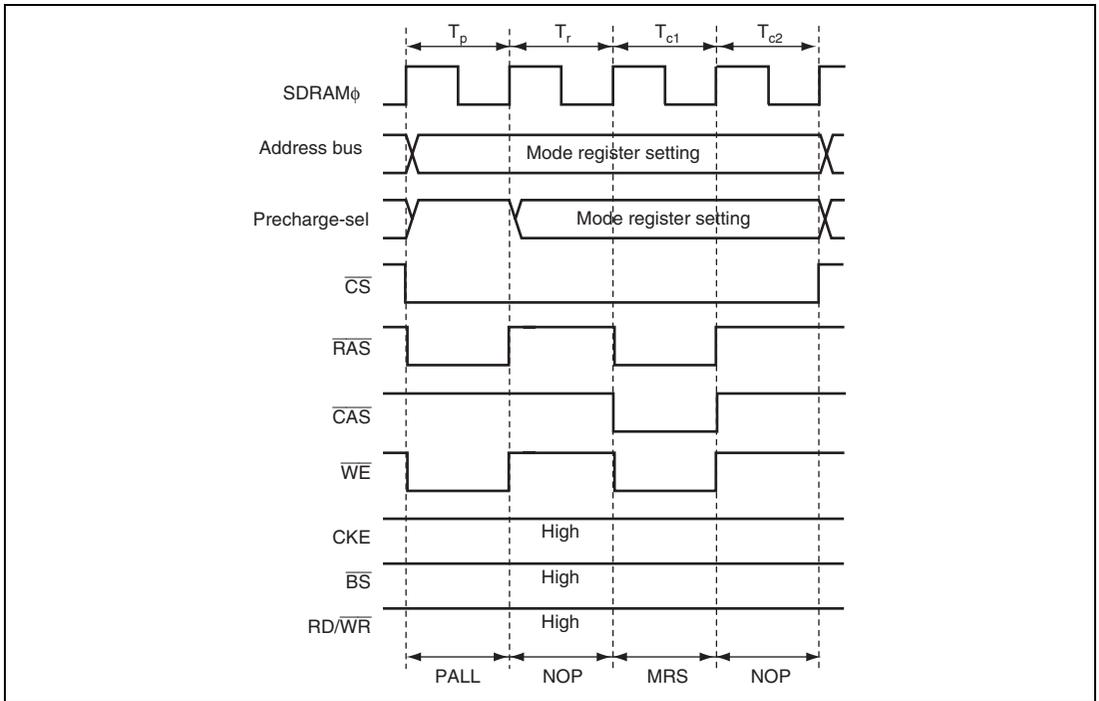
**Figure 9.82 Timing of Setting SDRAM Mode Register**
