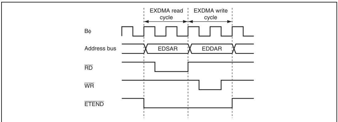
**Figure 11.2 Example of Timing in Dual Address Mode**
