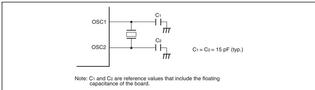
**Figure 26.6 Connection Example of 32.768-kHz Crystal Resonator**
