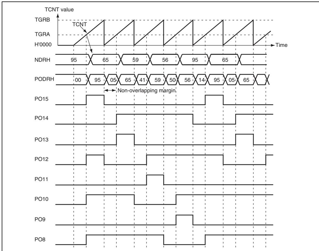
**Figure 15.12 Non-Overlapping Pulse Output Example (4-Phase Complementary)**
