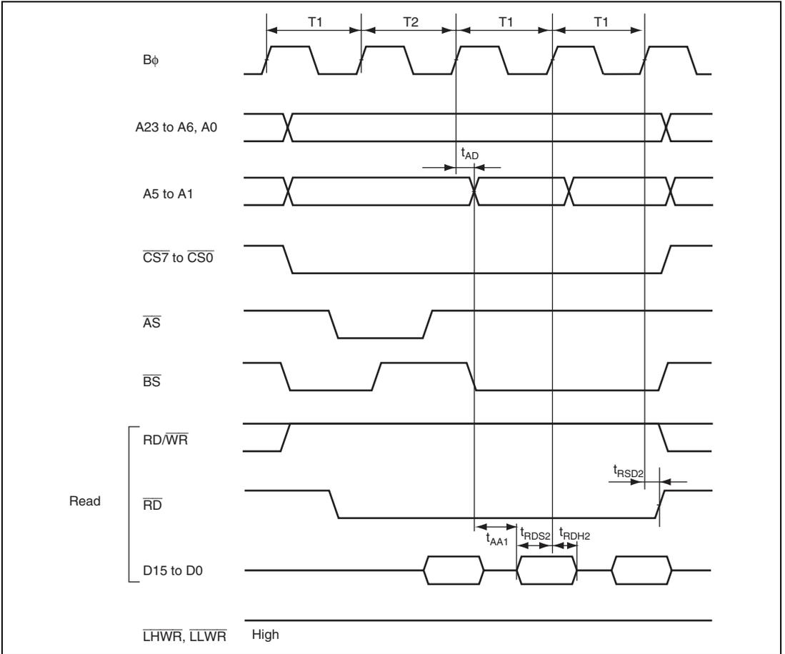
**Figure 29.15 Burst ROM Access Timing: One-State Burst Access**
