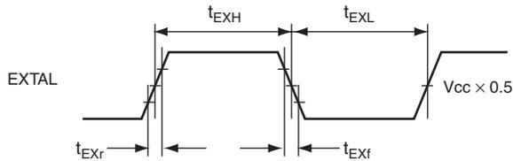
**Figure 29.5 External Input Clock Timing**
