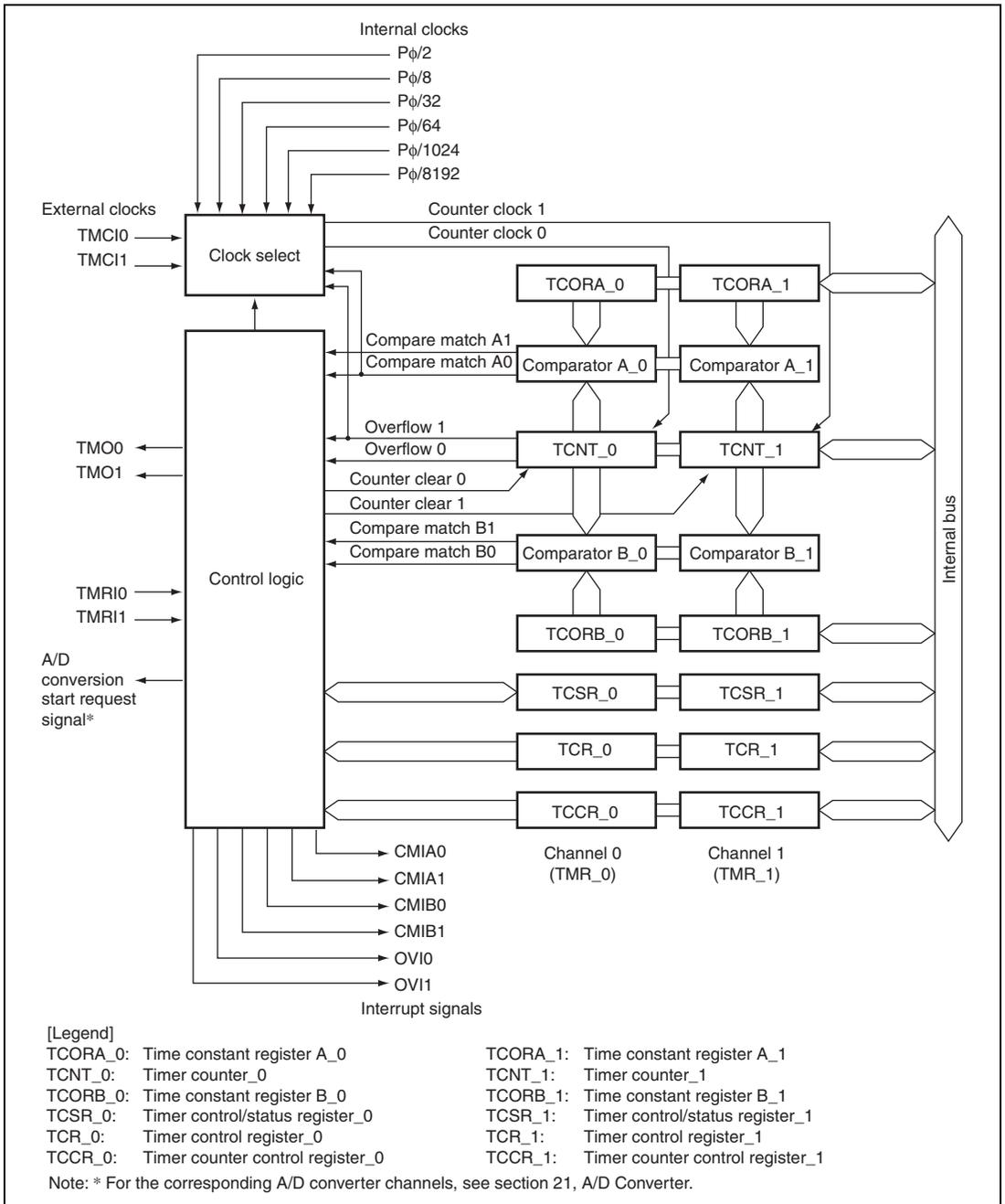
**Figure 16.1 Block Diagram of 8-Bit Timer Module (Unit 0)**
