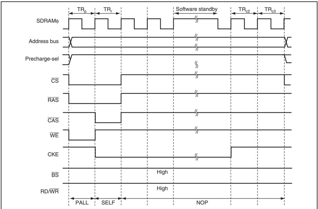
**Figure 9.79 Self-Refresh Timing in software standby mode**
