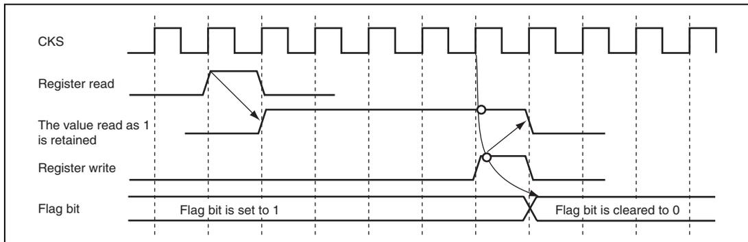
**Figure 8.3 Flag Bit Clearing Sequence (Condition Match Flag)**
