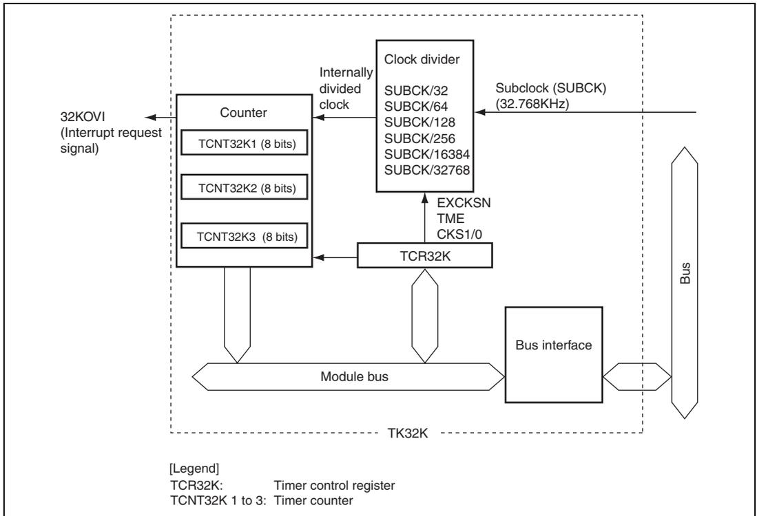
**Figure 17.1 Block Diagram of TM32K**
