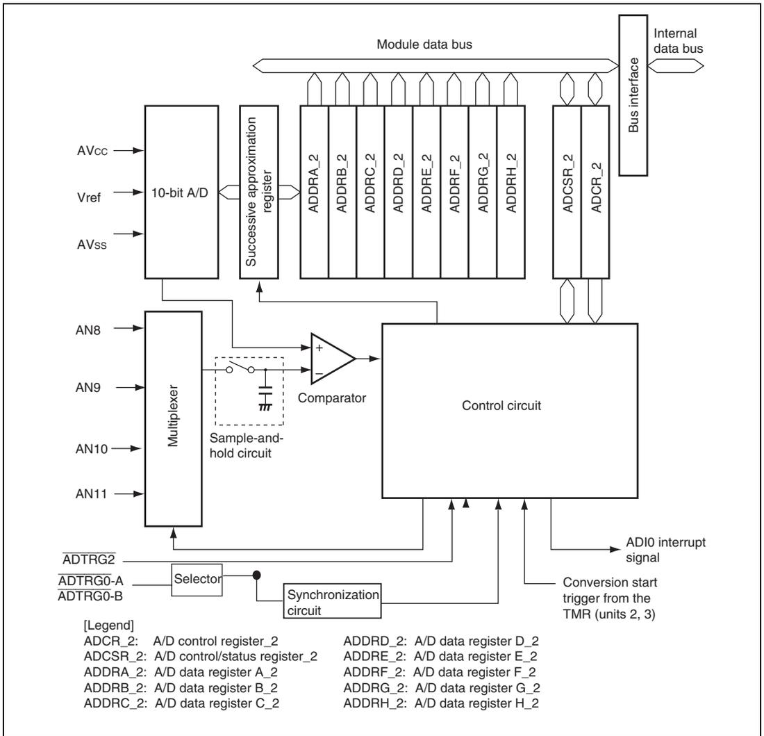
**Figure 21.3 Block Diagram of A/D Converter Unit 2 (AD\_2)**
