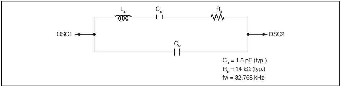
**Figure 26.7 Equivalent Circuit for 32.768-kHz Crystal Resonator**
