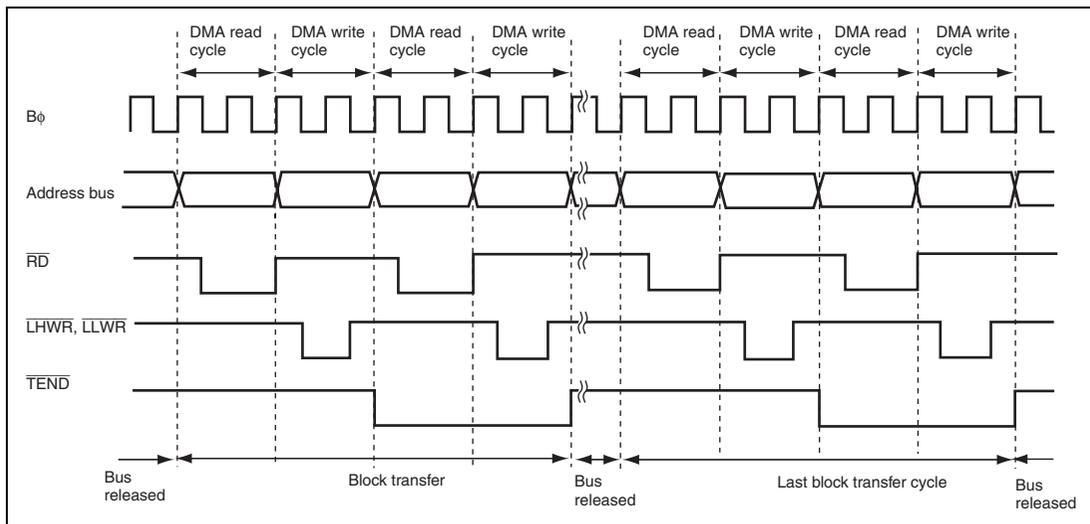
**Figure 10.28 Example of Transfer in Block Transfer Mode**
