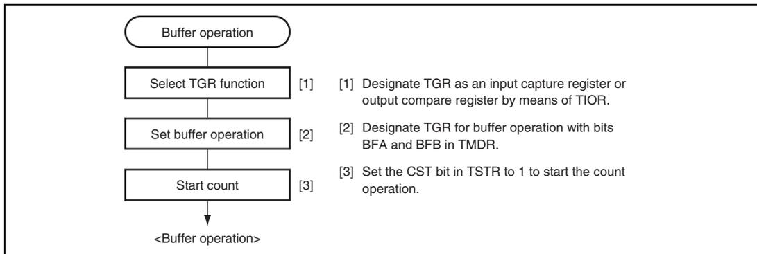
**Figure 14.15 Example of Buffer Operation Setting Procedure**
