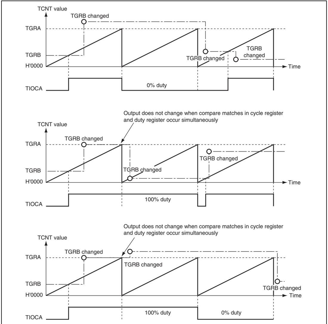
**Figure 14.24 Example of PWM Mode Operation (3)**
