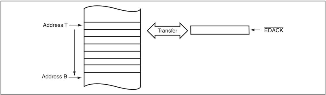
**Figure 11.6 Single Address Mode Operation**
