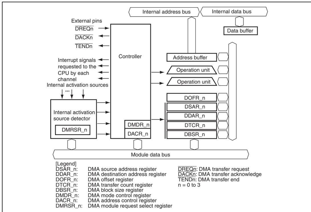
**Figure 10.1 Block Diagram of DMAC**
