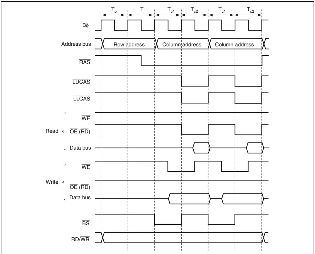
**Figure 9.48 Operation Timing of Fast-Page Mode (RAST = 0, CAST = 0)**
