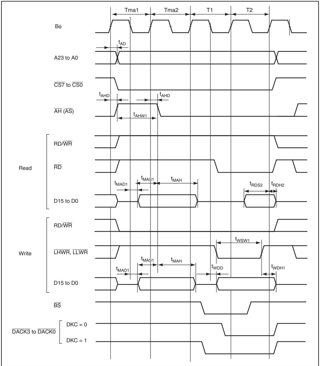
**Figure 29.17 Address/Data Multiplexed Access Timing (No Wait)**
