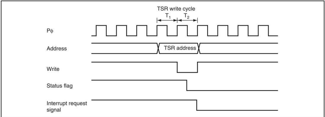
**Figure 14.43 Timing for Status Flag Clearing by CPU**
