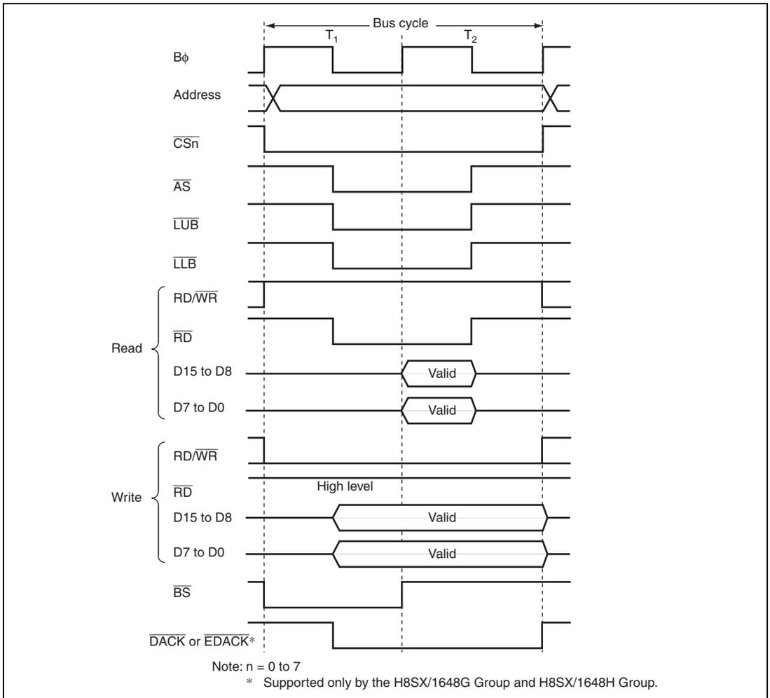
**Figure 9.25 16-Bit 2-State Access Space Bus Timing**
