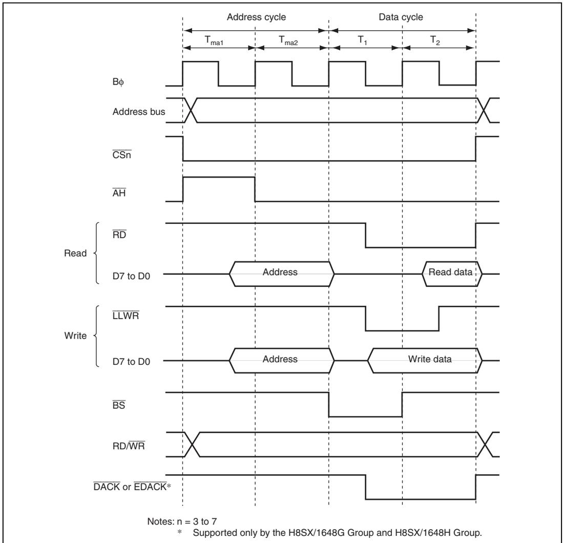
**Figure 9.31 8-Bit Access Space Access Timing (ABWH<sub>n</sub> = 1, ABWL<sub>n</sub> = 1)**
