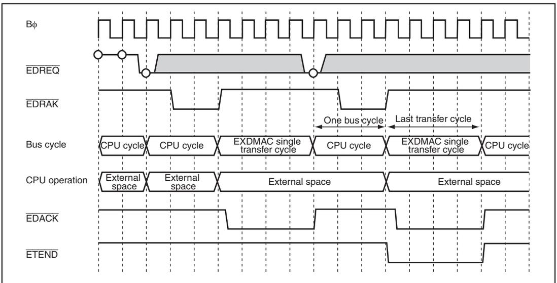
**Figure 11.45 External Request/Normal Transfer Mode/Cycle Steal Mode
