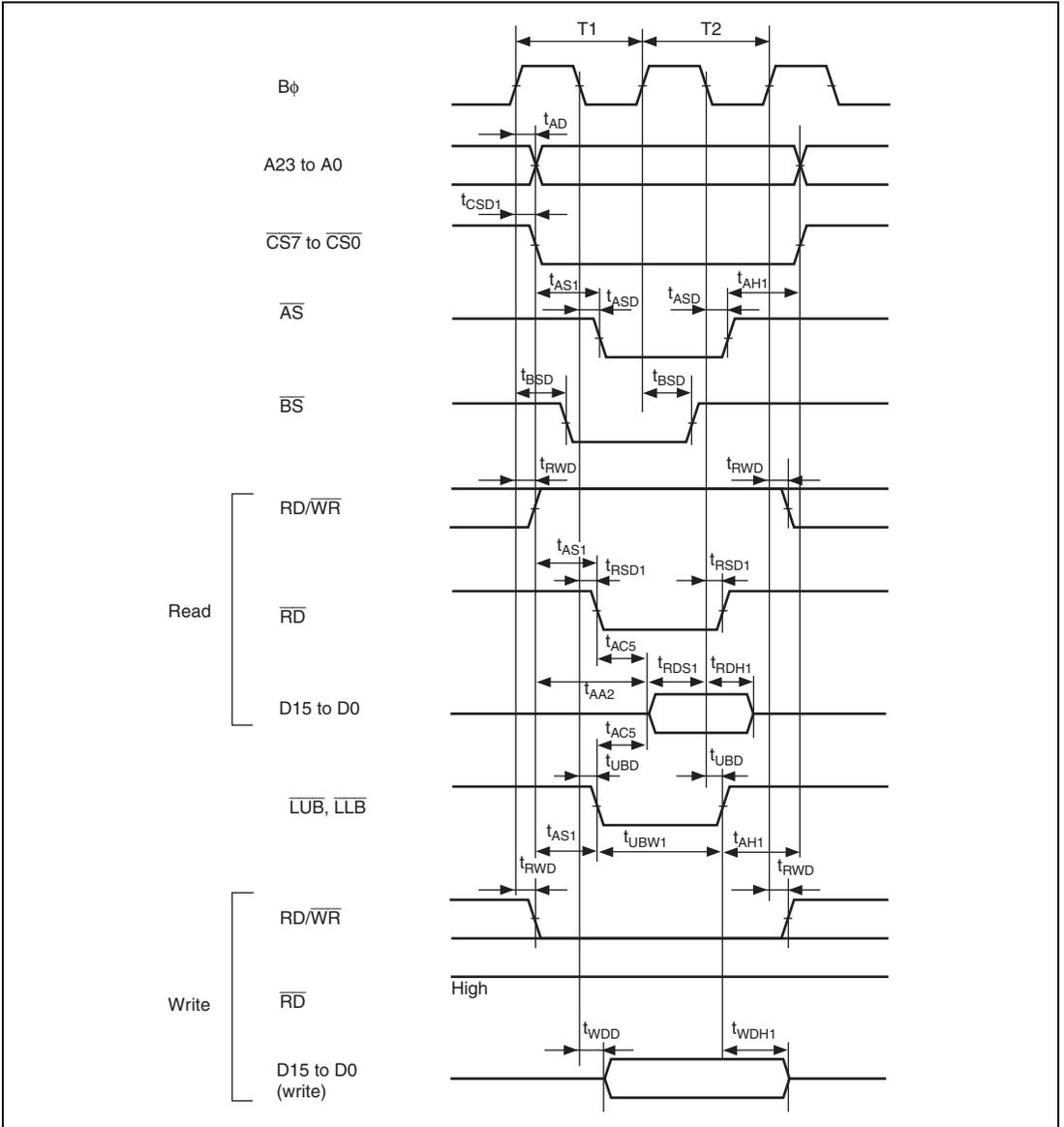
Figure 29.13 Byte Control SRAM: Two-State Read/Write Access
