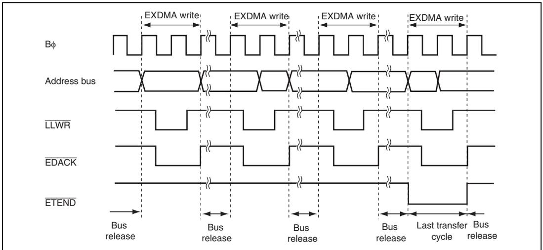
**Figure 11.35 Example of Single Address Mode (Byte Write) Transfer**
