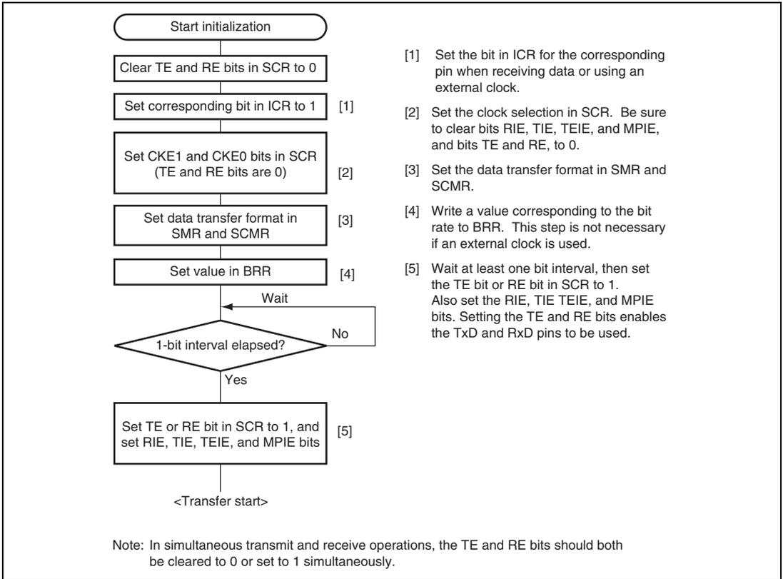
**Figure 19.18 Sample SCI Initialization Flowchart**
