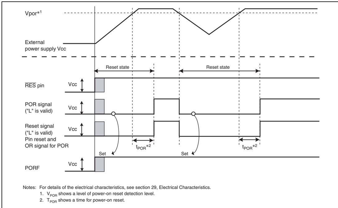
**Figure 4.2 Operation of a Power on Reset**
