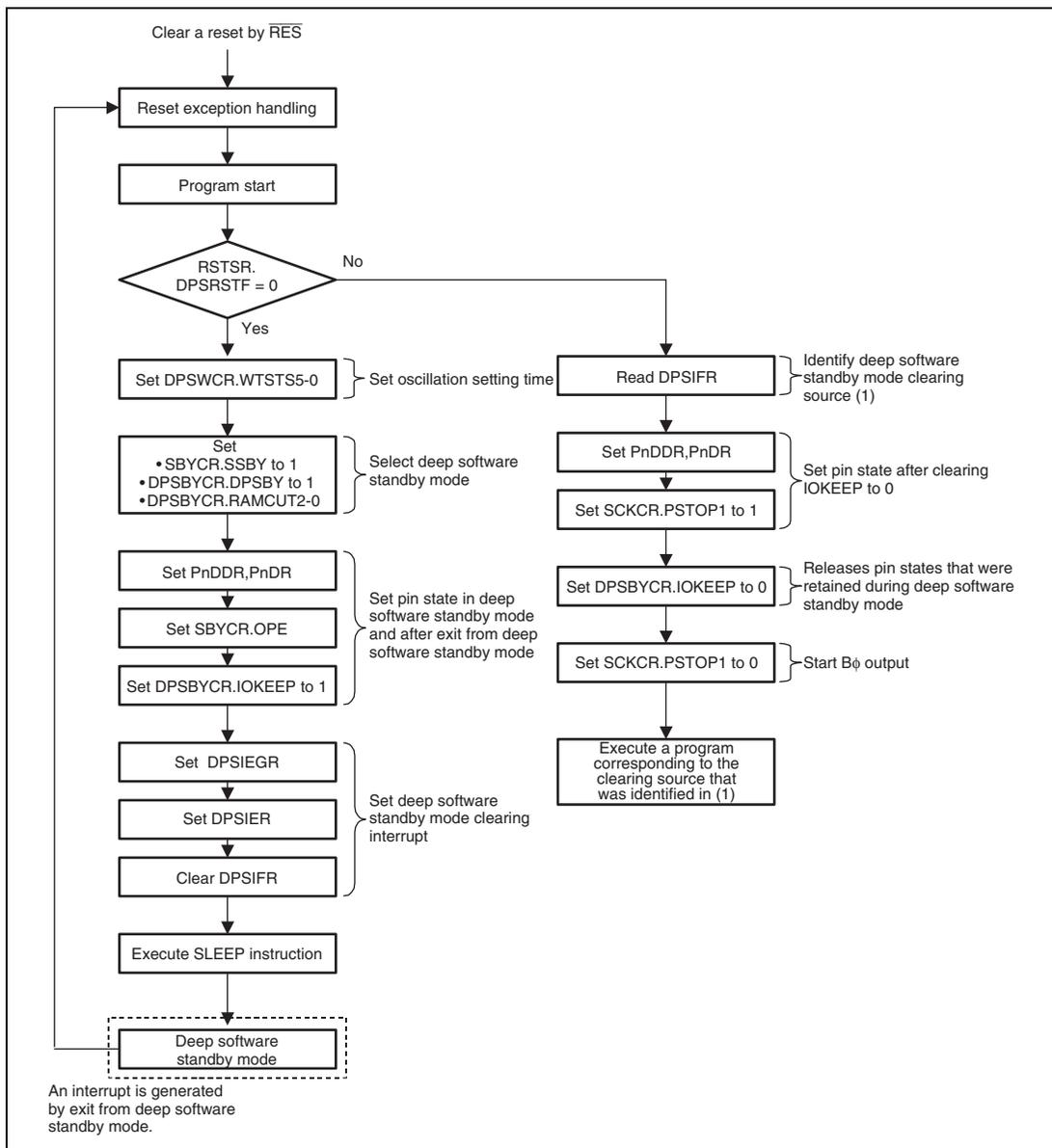
**Figure 27.7 Flowchart of Deep Software Standby Mode Operation**
