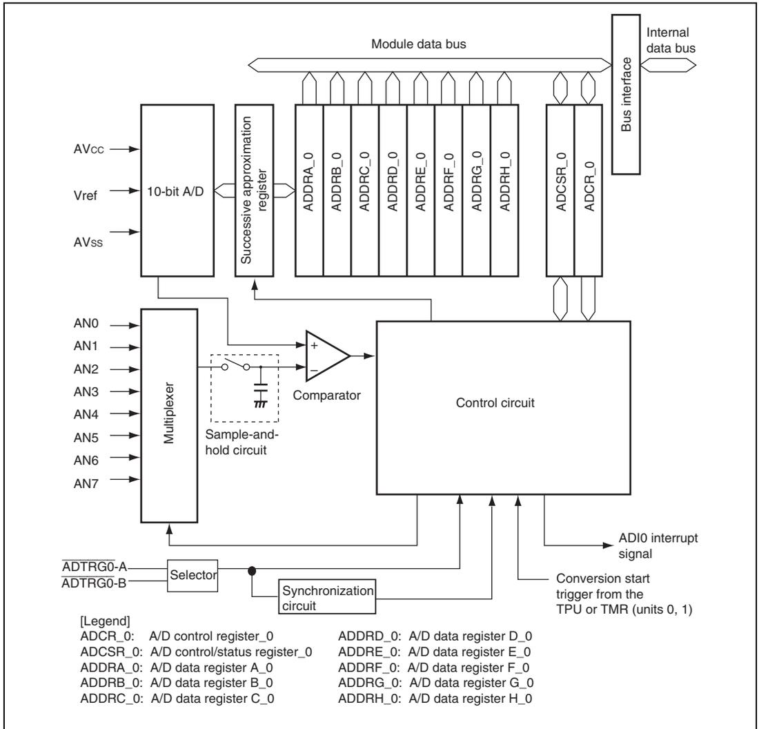
**Figure 21.1 Block Diagram of A/D Converter Unit 0 (AD\_0)**
