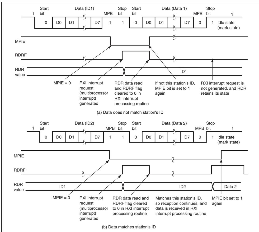
**Figure 19.15 Example of SCI Operation for Reception
