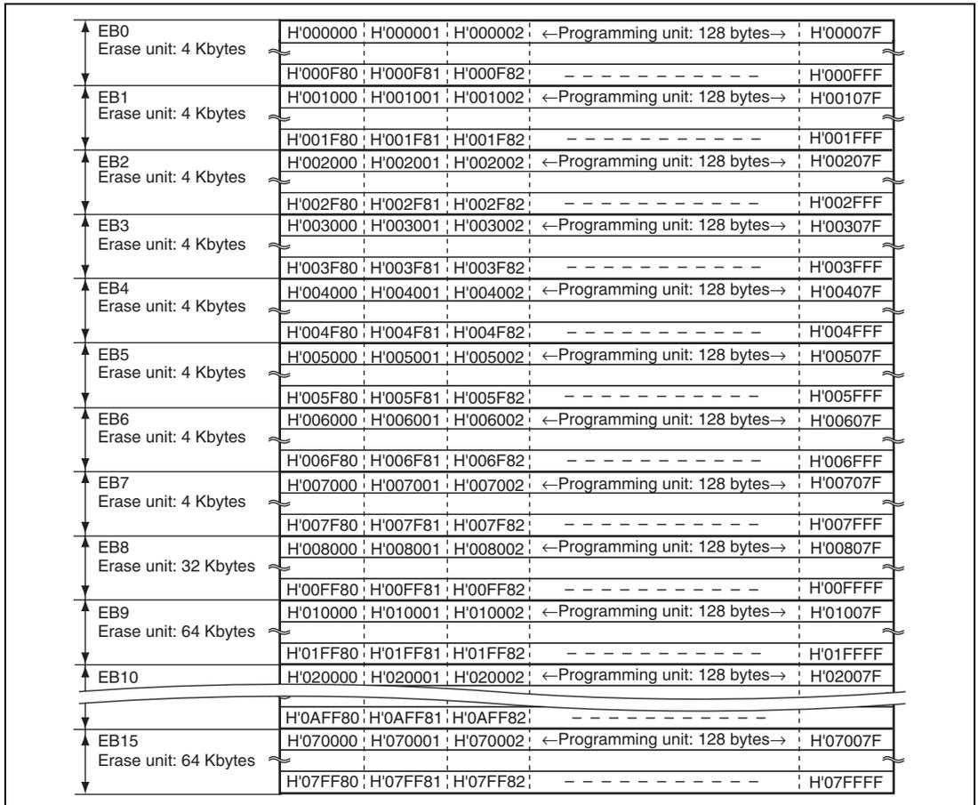
Figure 24.4 User MAT Block Structure of H8SX/1644
