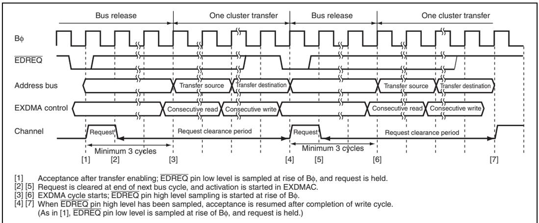
**Figure 11.62 Example of Cluster Transfer Mode Transfer Activated by  $\overline{\text{EDREQ}}$  Pin Falling Edge**
