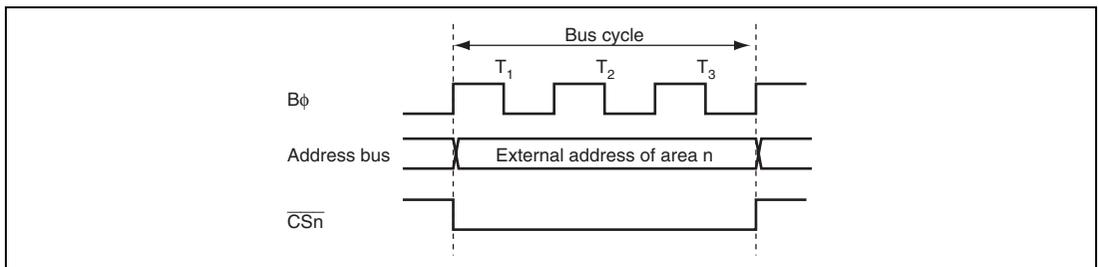
**Figure 9.9**  $\overline{CSn}$  Signal Output Timing ( $n = 0$  to 7)
