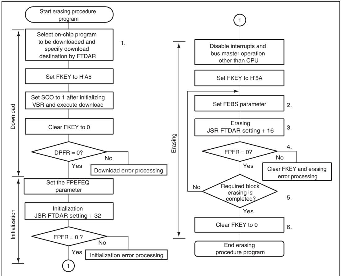
Figure 24.12 Erasing Procedure in User Program Mode
