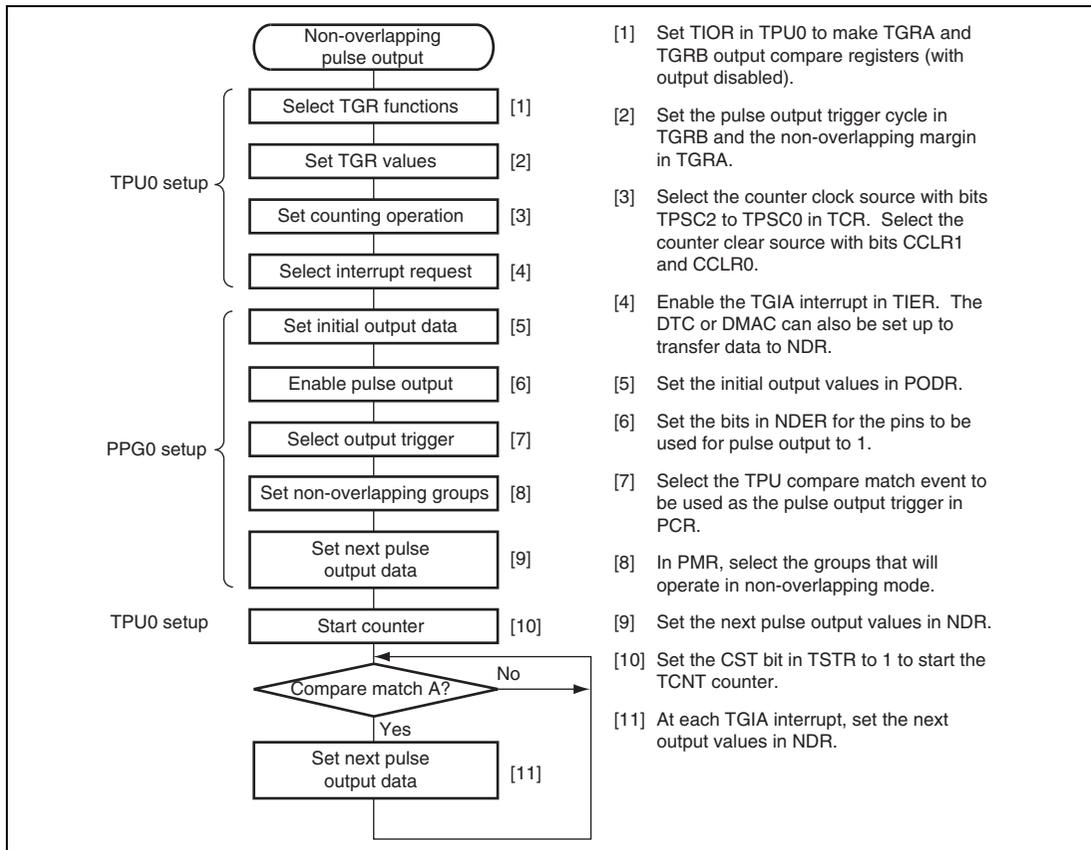
**Figure 15.10 Setup Procedure for Non-Overlapping Pulse Output (PPG0)**
