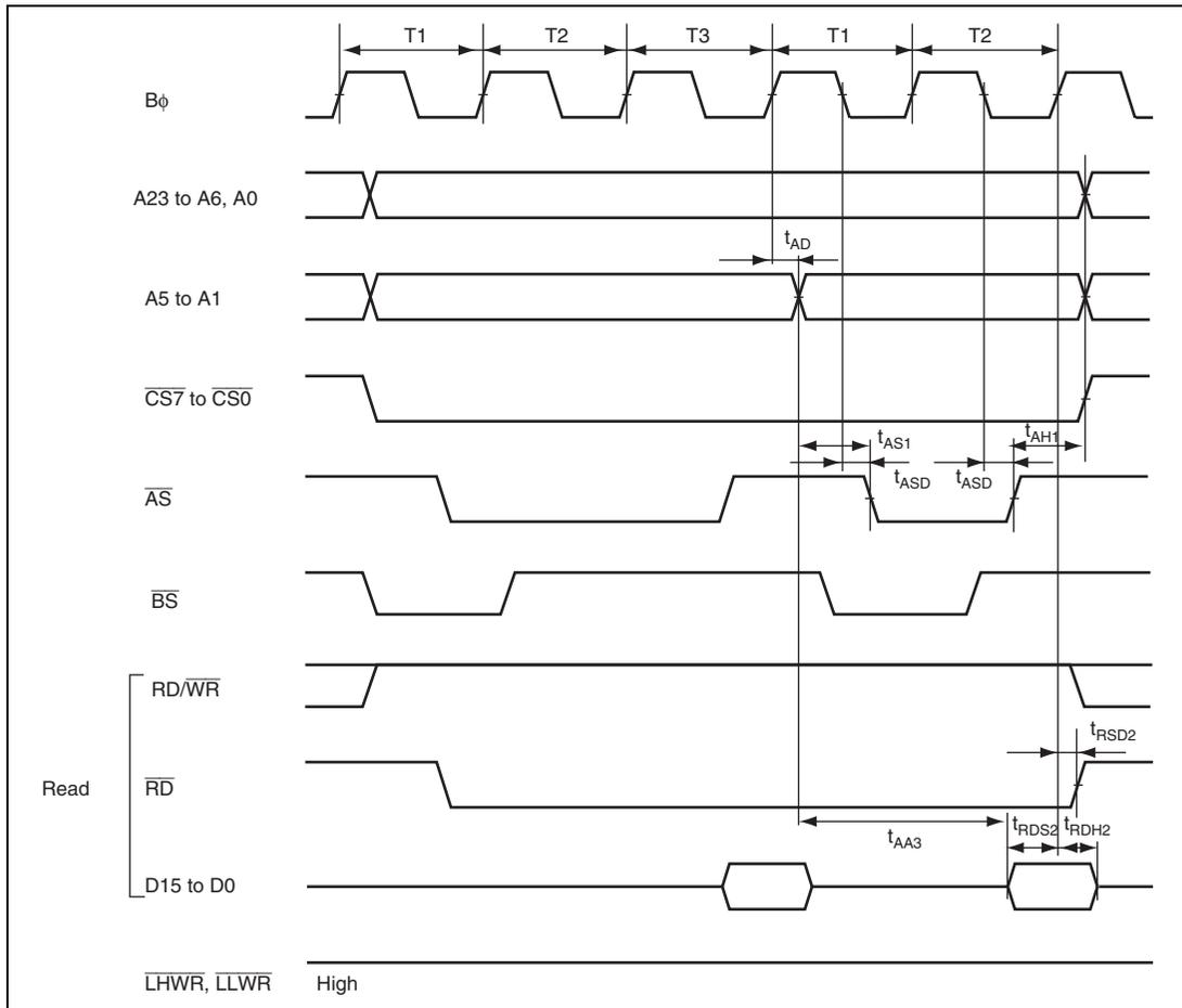
**Figure 29.16 Burst ROM Access Timing: Two-State Burst Access**
