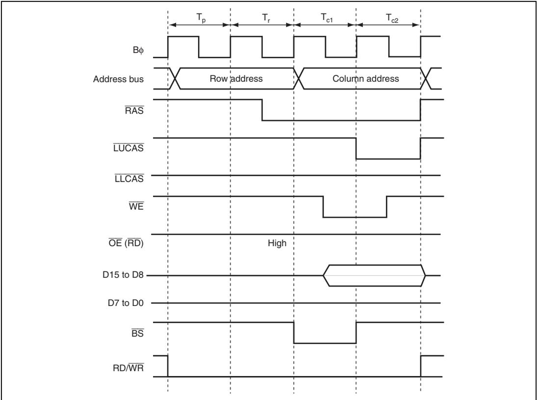
**Figure 9.45 Timing Example of Byte Control with Use of Two CAS Signals
