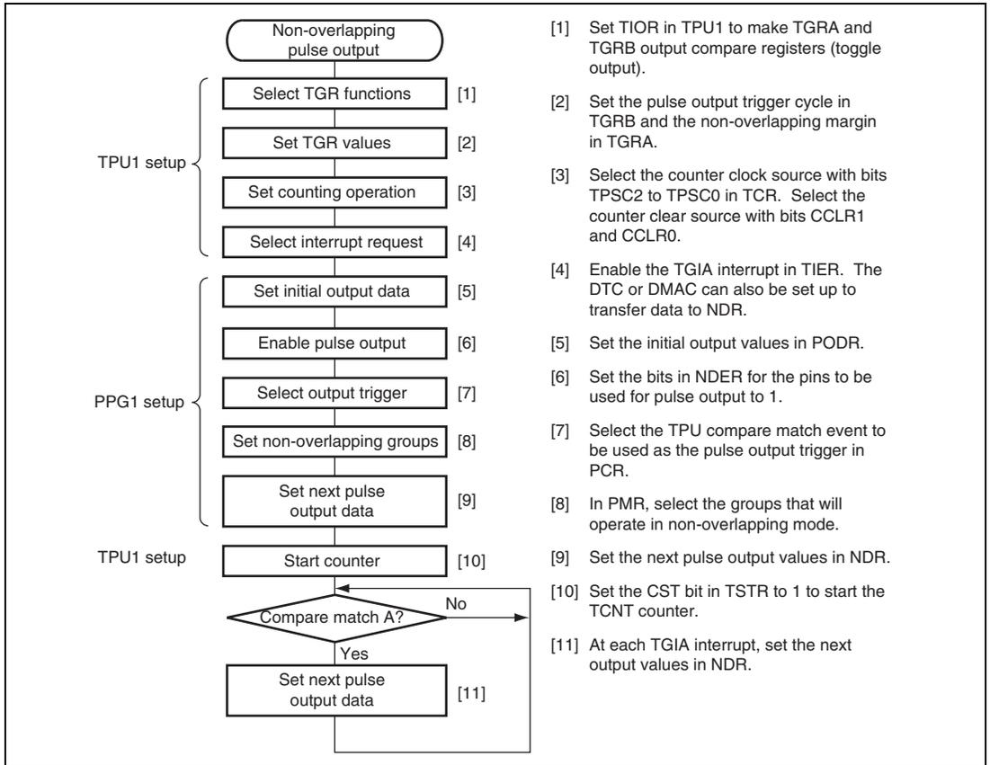
**Figure 15.11 Setup Procedure for Non-Overlapping Pulse Output (PPG1)**
