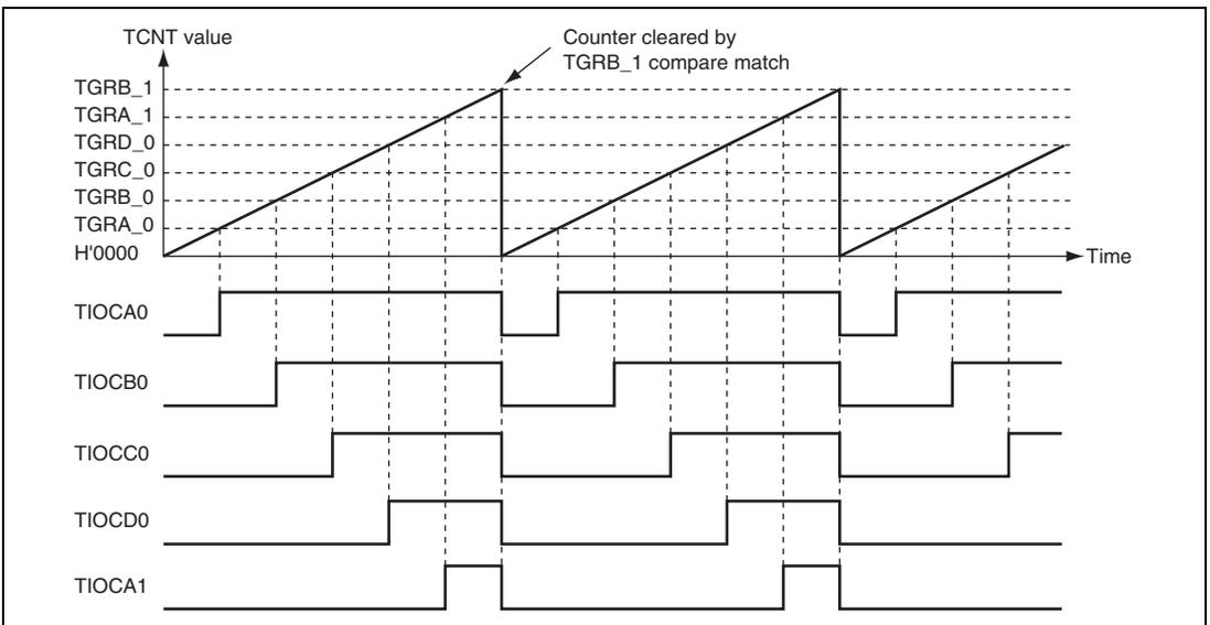
**Figure 14.23 Example of PWM Mode Operation (2)**
