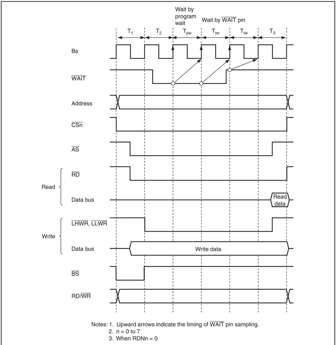
**Figure 9.21 Example of Wait Cycle Insertion Timing**
