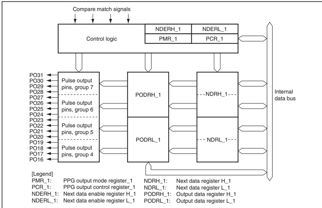
**Figure 15.2 Block Diagram of PPG (Unit 1)**
