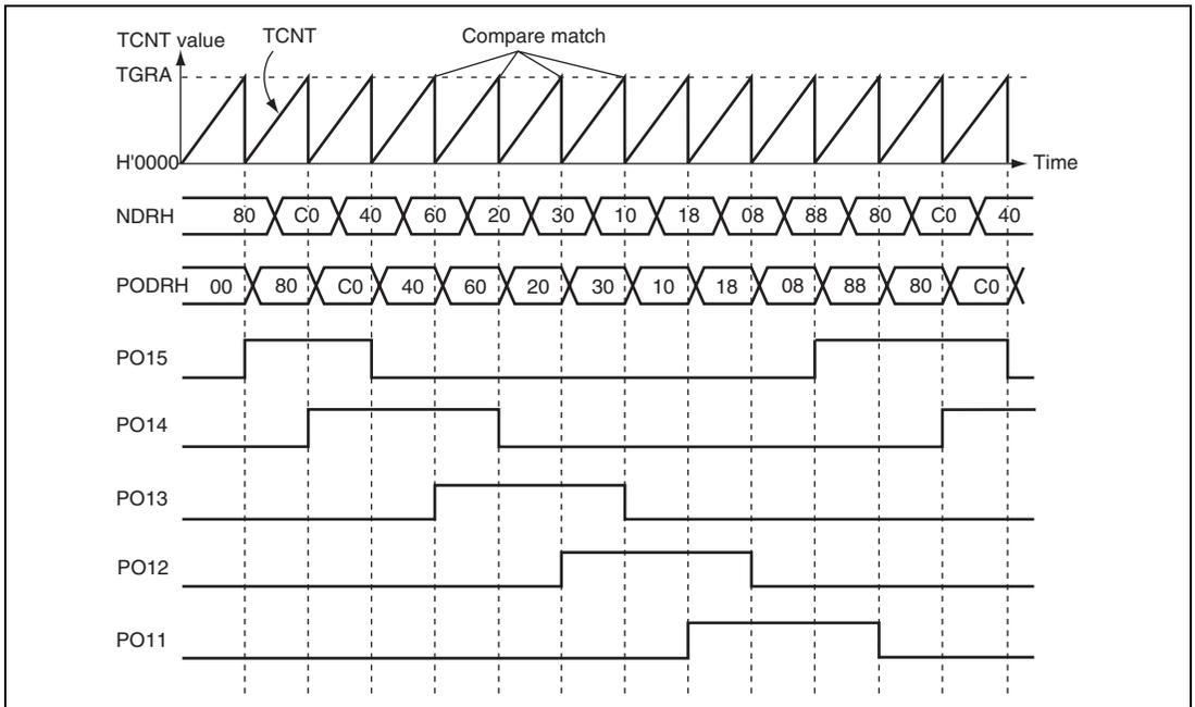
**Figure 15.7 Normal Pulse Output Example (5-Phase Pulse Output)**
