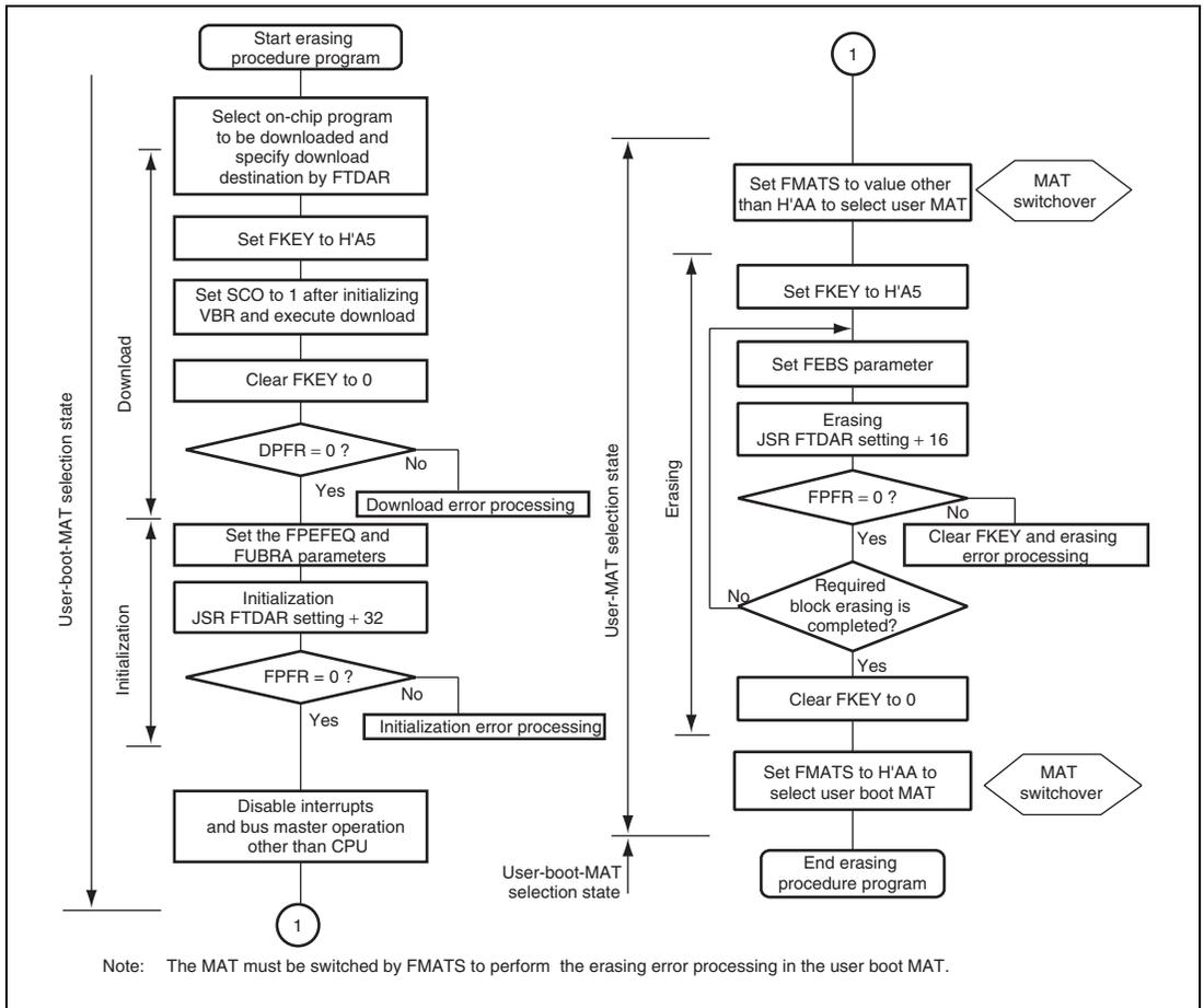
**Figure 24.15 Procedure for Erasing User MAT in User Boot Mode**
