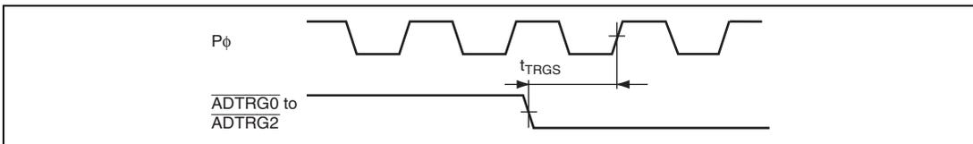
**Figure 29.52 A/D Converter External Trigger Input Timing**
