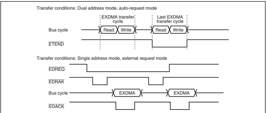
**Figure 11.7 Examples of Timing in Normal Transfer Mode**
