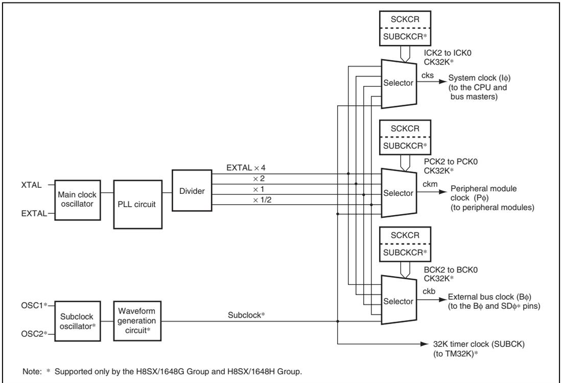
**Figure 26.1 Block Diagram of Clock Pulse Generator**
