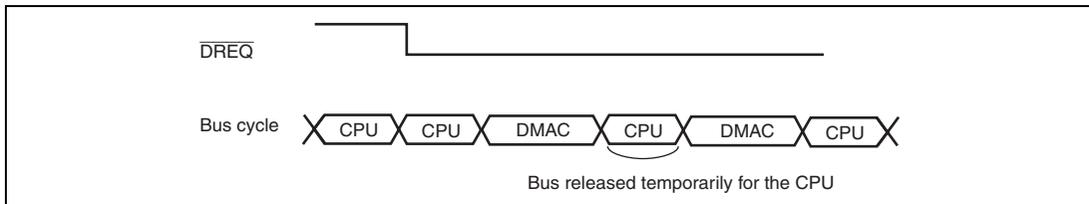
**Figure 10.13 Example of Timing in Cycle Stealing Mode**
