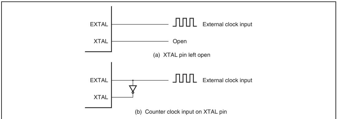
**Figure 26.4 External Clock Input (Examples)**
