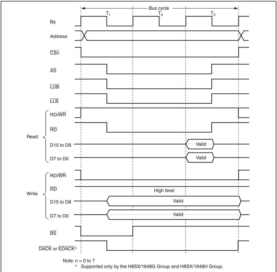
**Figure 9.26 16-Bit 3-State Access Space Bus Timing**
