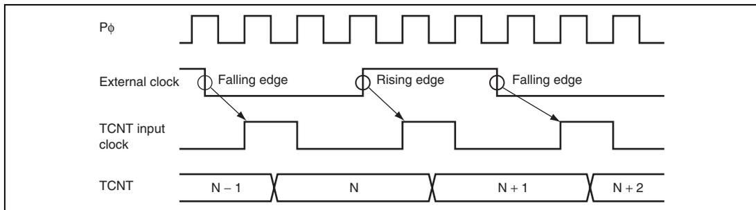
**Figure 14.32 Count Timing in External Clock Operation**
