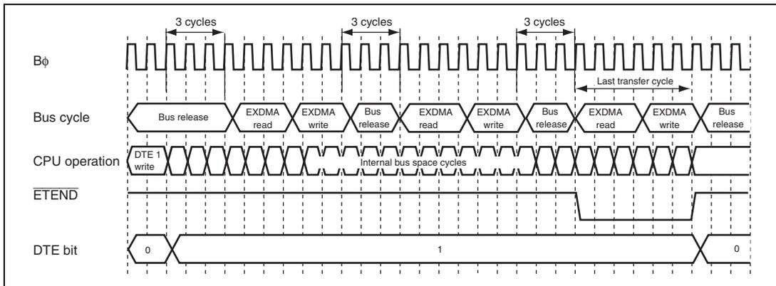
**Figure 11.39 Auto-Request/Normal Transfer Mode/Cycle Steal Mode
