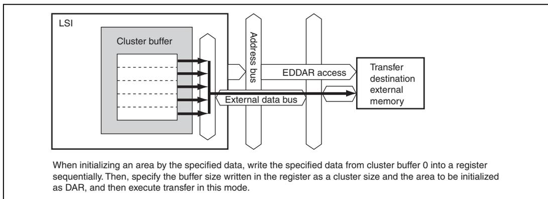
**Figure 11.59 Data Flow in Cluster Transfer Write Address Mode
