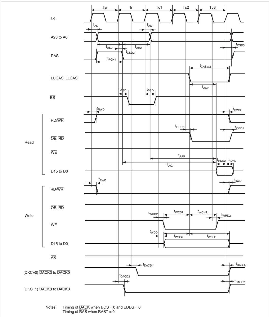
Figure 29.22 DRAM Access Timing / Three-State Access (When  $RAST=1$ )\*
