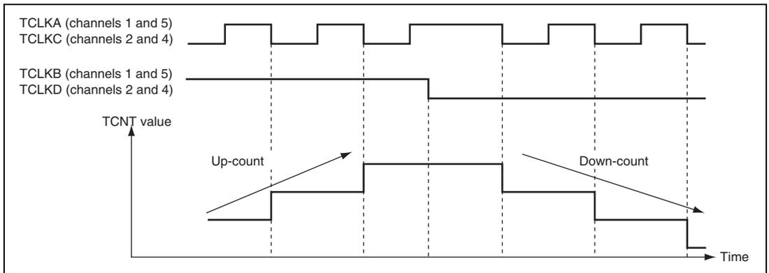
**Figure 14.27 Example of Phase Counting Mode 2 Operation**
