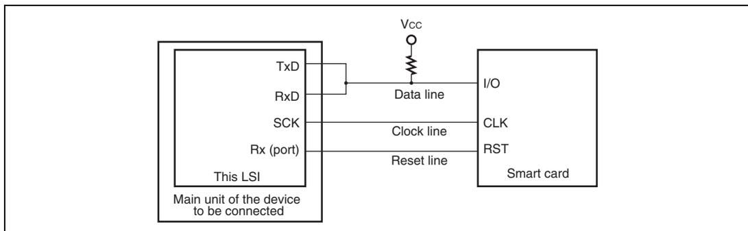
**Figure 19.24 Pin Connection for Smart Card Interface**
