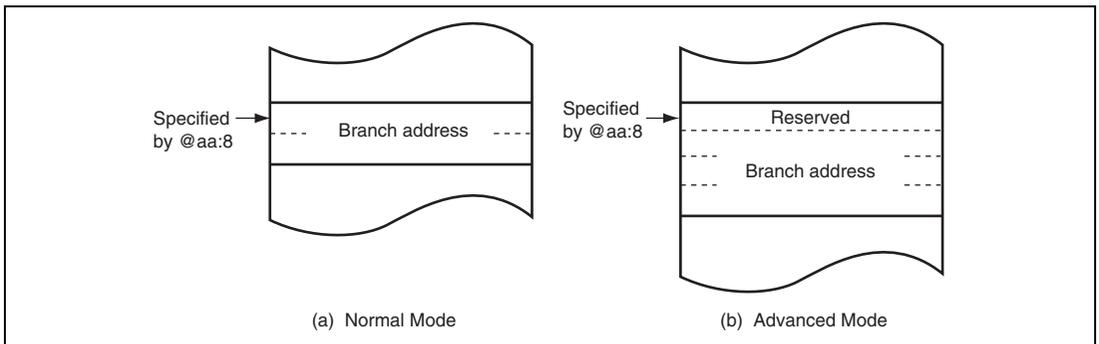
**Figure 2.15 Branch Address Specification in Memory Indirect Mode**
