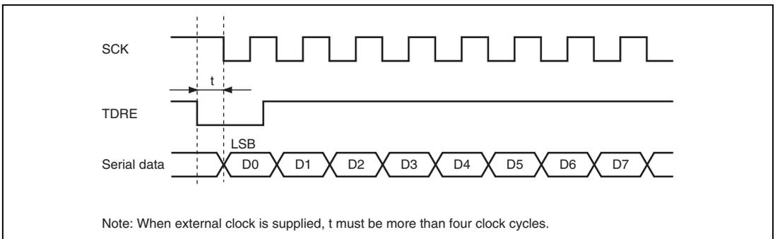
**Figure 19.38 Sample Transmission using DTC in Clock Synchronous Mode**
