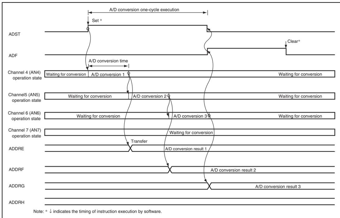
**Figure 21.6 Example of A/D Conversion
