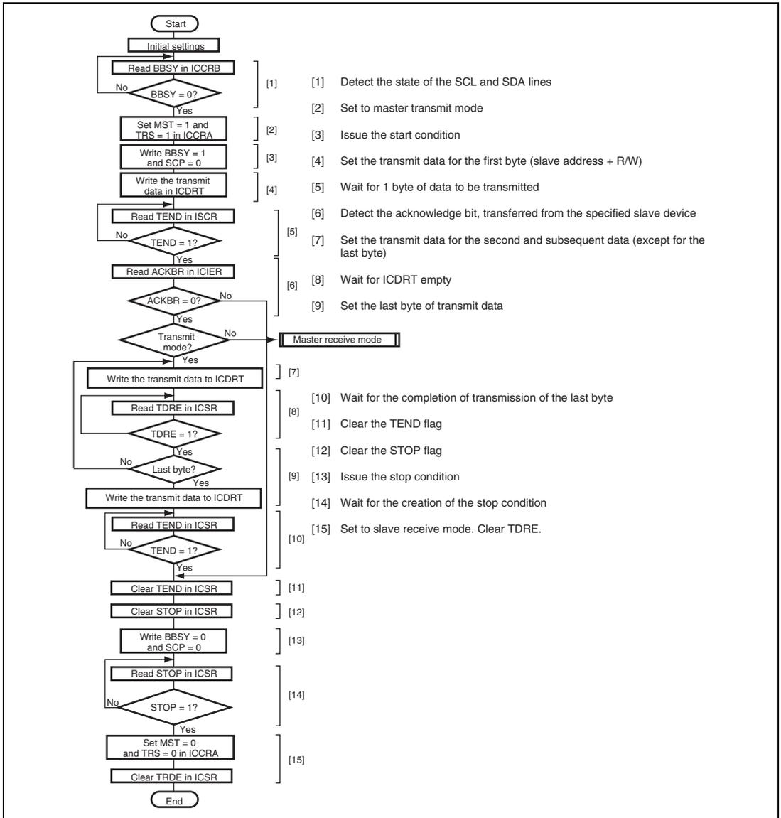
**Figure 20.14 Sample Flowchart of Master Transmit Mode**
