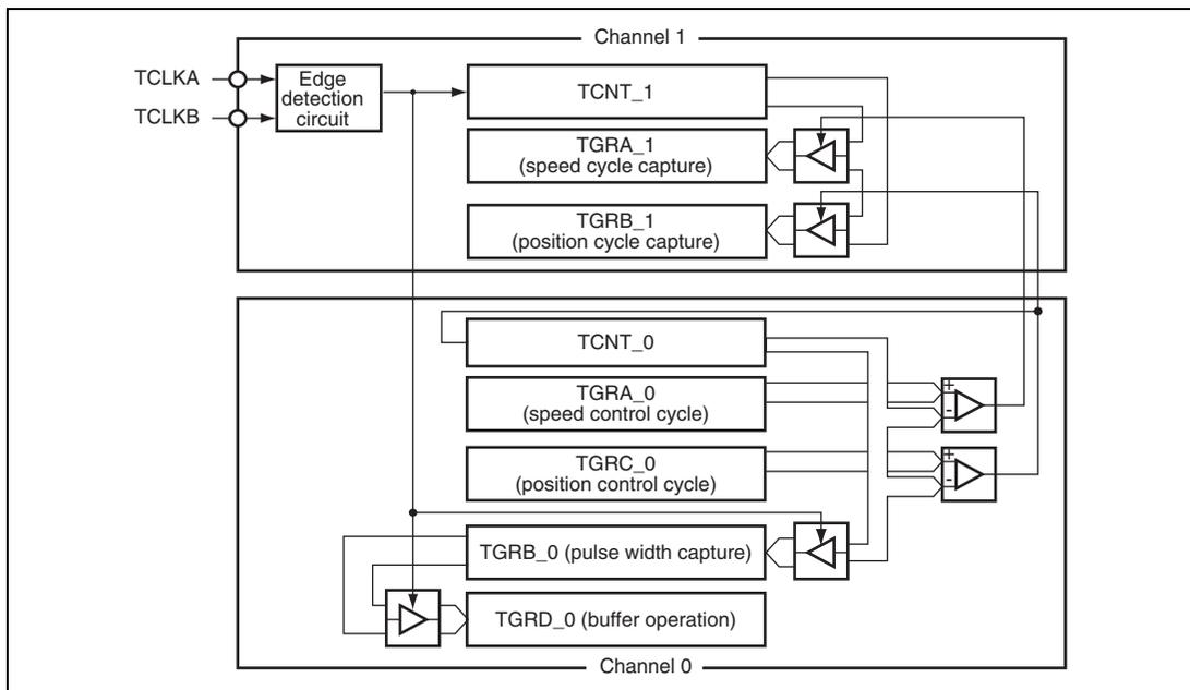
**Figure 14.30 Phase Counting Mode Application Example**
