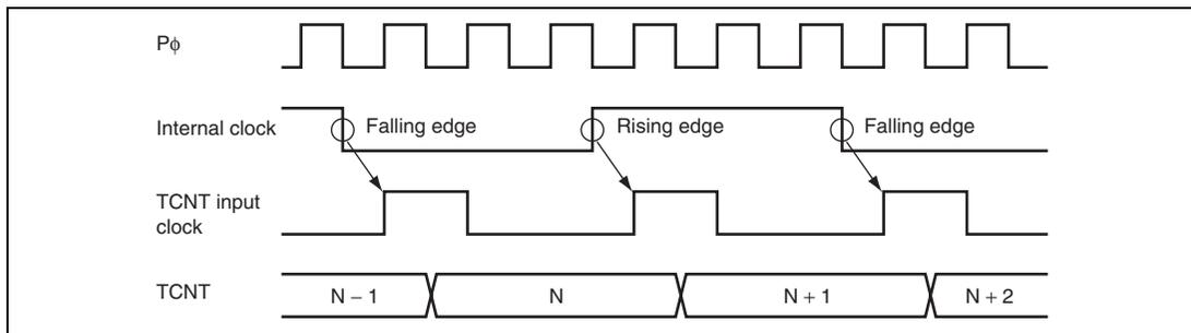
**Figure 14.31 Count Timing in Internal Clock Operation**
