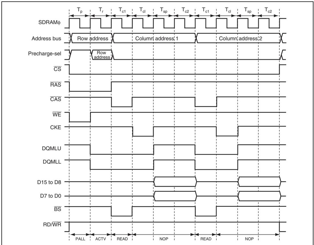
**Figure 9.67 Read Timing Example when  $CKSPE = 1$  (CAS Latency = 2)**
