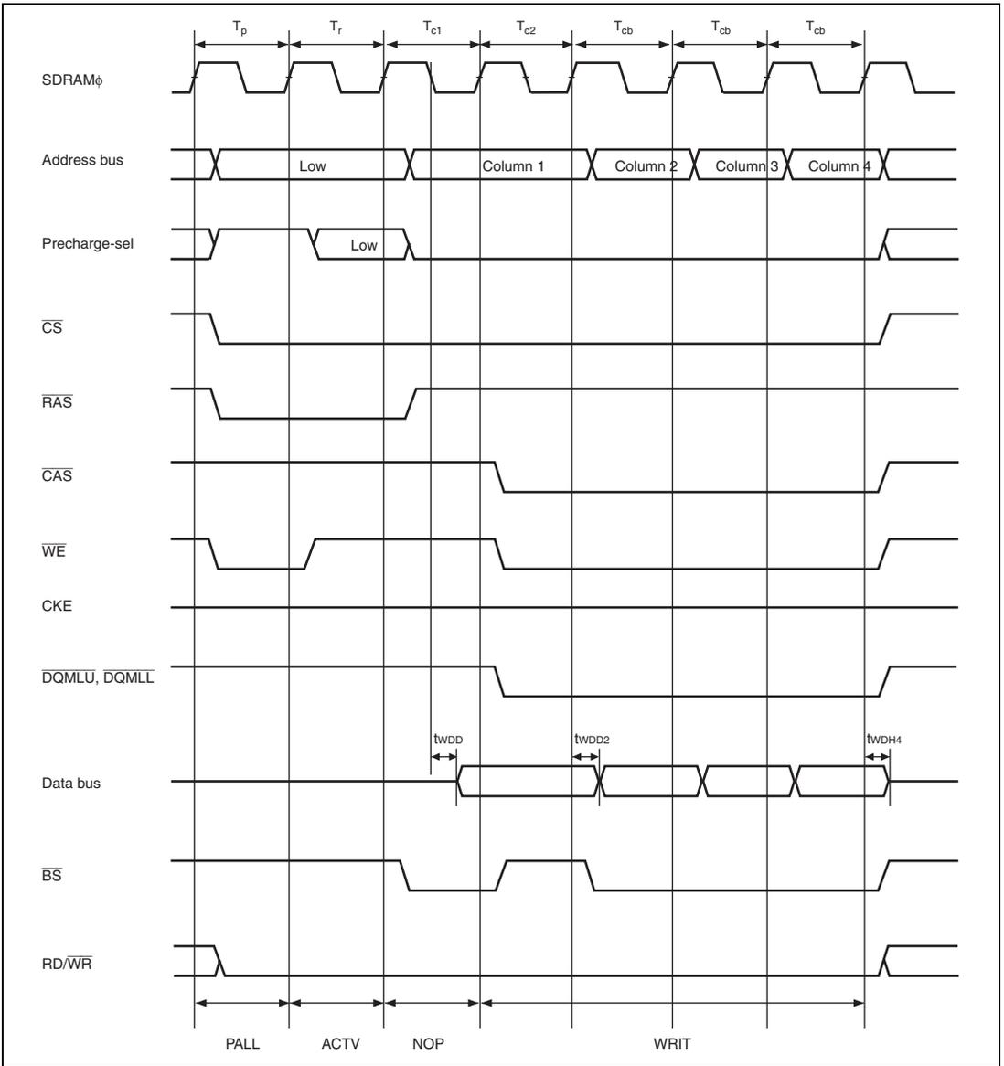
Figure 29.33 Synchronous DRAM Cluster Transfer Access Timing (Write)\*
