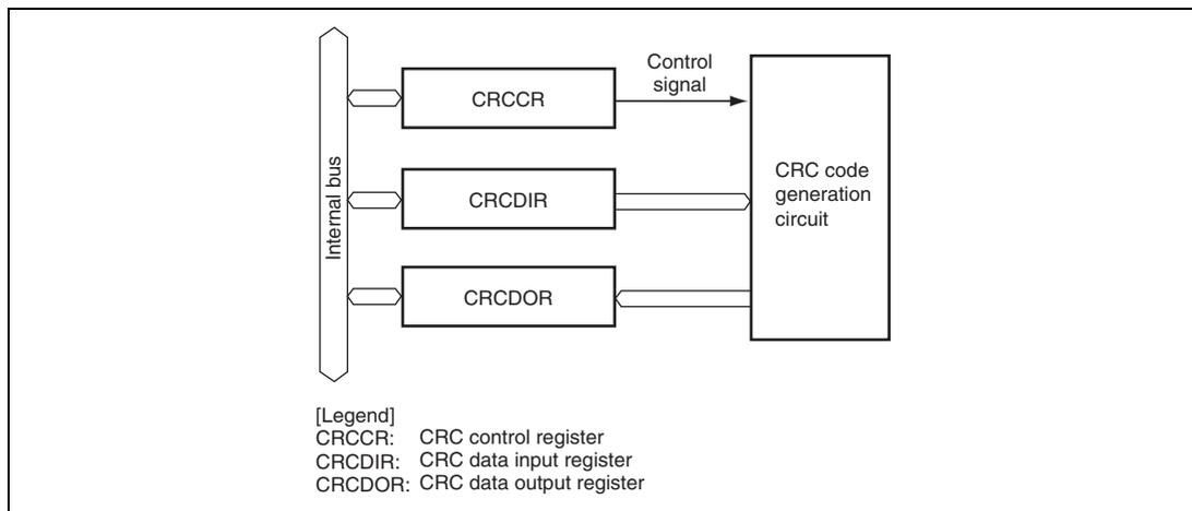
**Figure 19.43 Block Diagram of CRC Operation Circuit**
