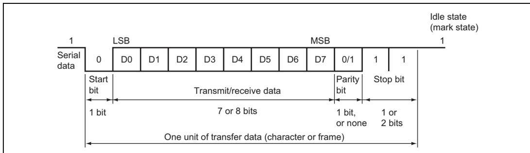
**Figure 19.5 Data Format in Asynchronous Communication
