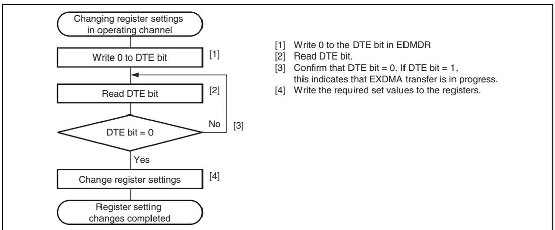
**Figure 11.21 Procedure for Changing Register Settings in Operating Channel**
