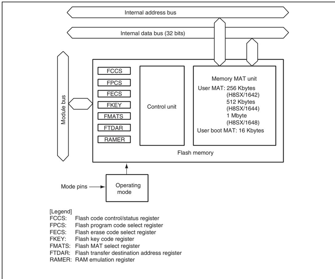
**Figure 24.1 Block Diagram of Flash Memory**
