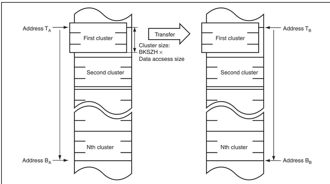
**Figure 11.55 Cluster Transfer Dual Address Mode Operation**
