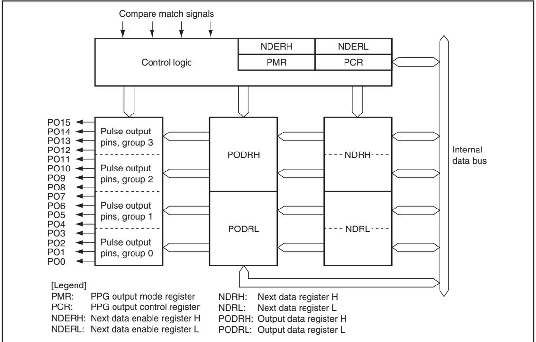
**Figure 15.1 Block Diagram of PPG (Unit 0)**
