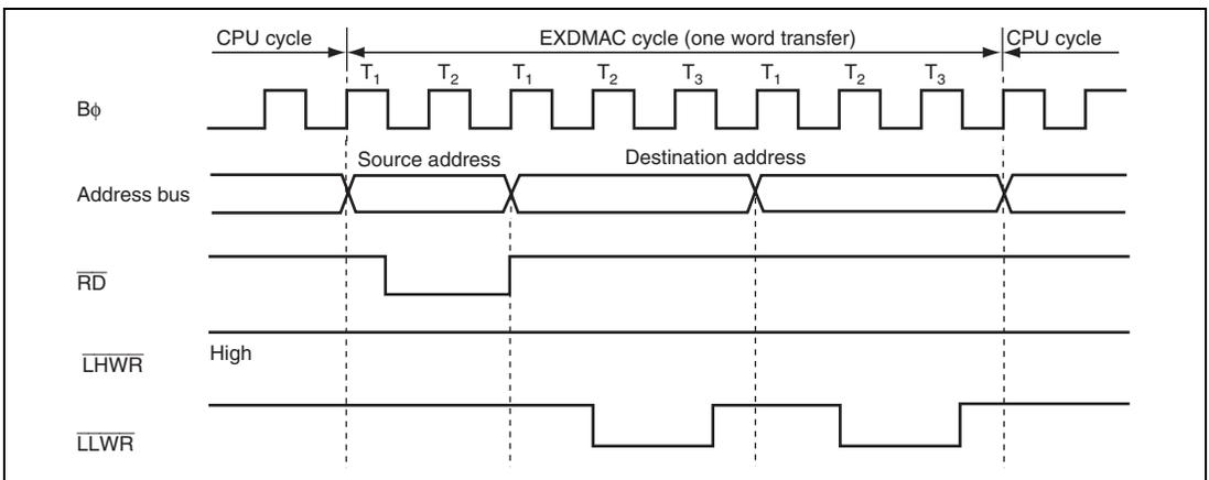
**Figure 11.23 Example of EXDMA Transfer Bus Timing**
