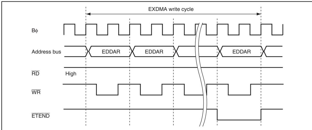
**Figure 11.60 Timing in Cluster Transfer Write Address Mode
