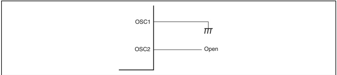
**Figure 26.8 Pin Handling when Subclock is not Used**
