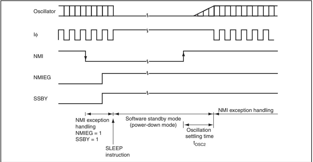
**Figure 29.3 Oscillation Settling Timing after Software Standby Mode**
