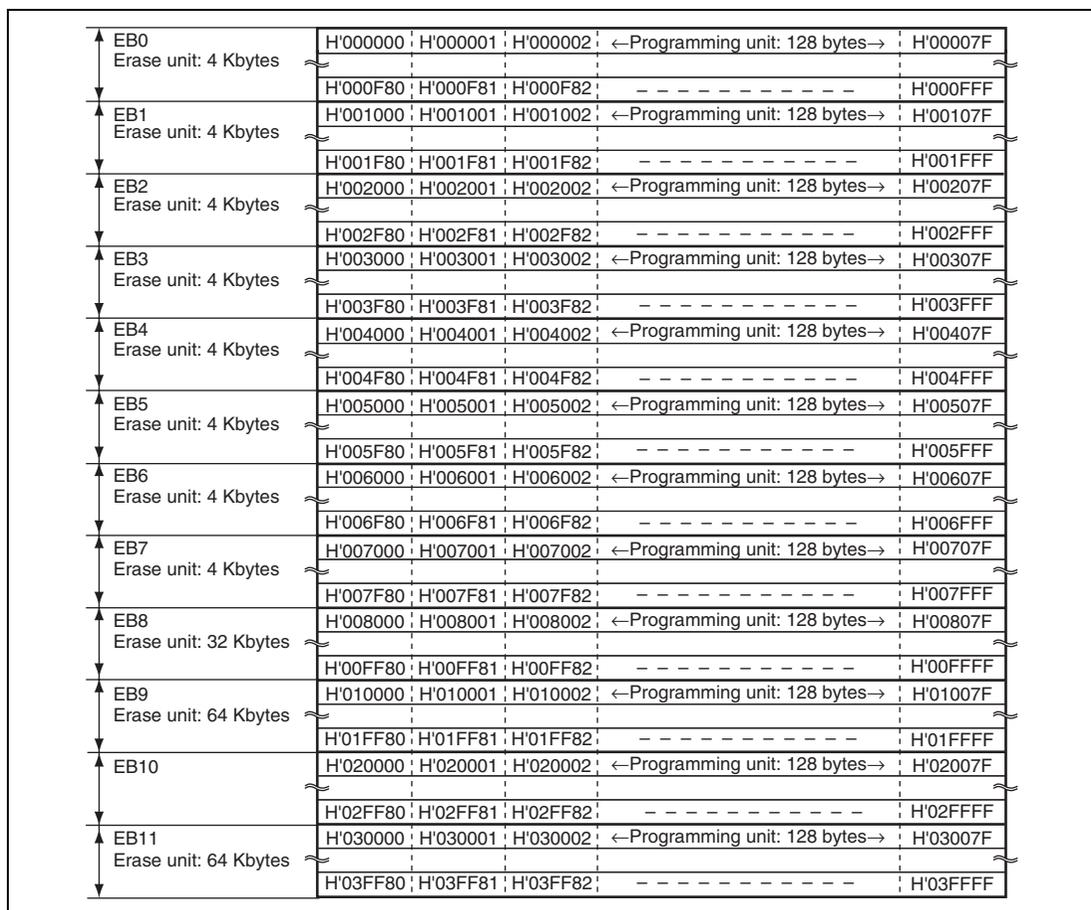
Figure 24.4 User MAT Block Structure of H8SX/1642
