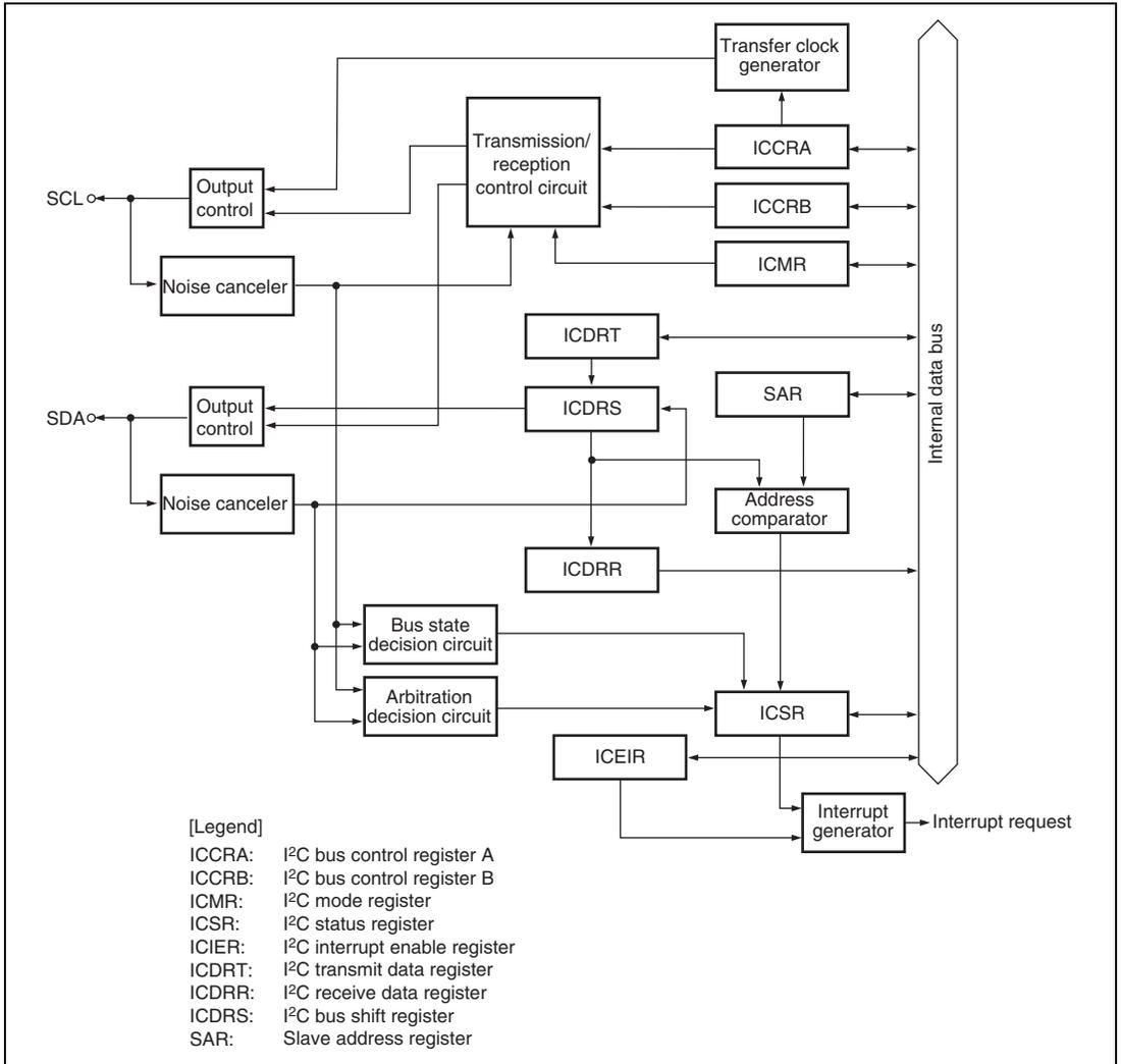
**Figure 20.1 Block Diagram of I<sup>2</sup>C Bus Interface 2**
