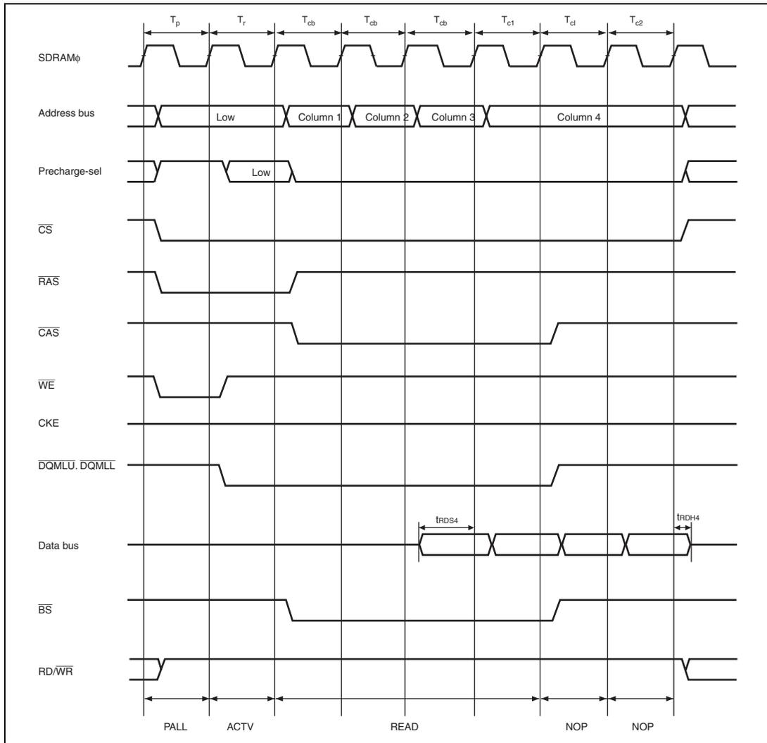
**Figure 29.32 Synchronous DRAM Cluster Transfer Access Timing (Read)\***
