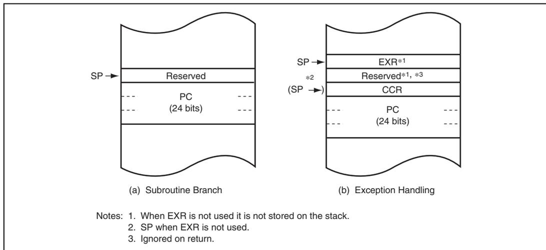
**Figure 2.5 Stack Structure (Middle and Advanced Modes)**
