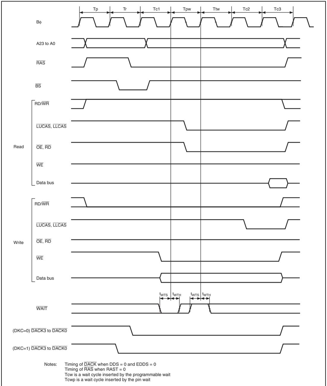
**Figure 29.23 DRAM Access Timing / Three-State Access, One Wait\***
