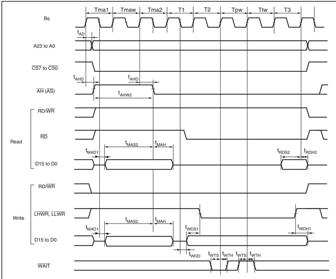
**Figure 29.18 Address/Data Multiplexed Access Timing (Wait Control)**
