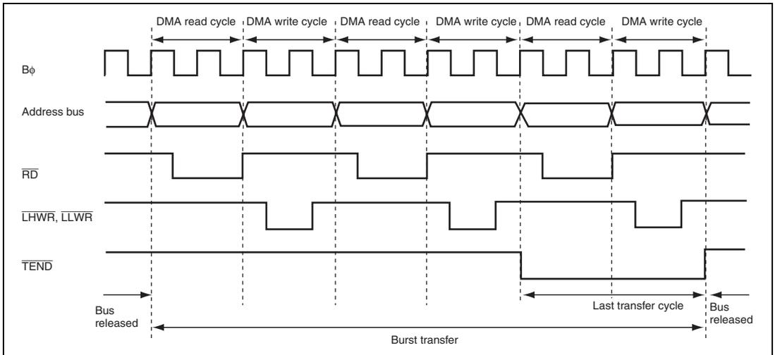
**Figure 10.27 Example of Transfer in Normal Transfer Mode by Burst Access**
