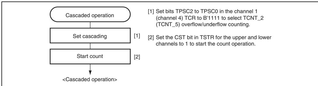
**Figure 14.18 Cascaded Operation Setting Procedure**
