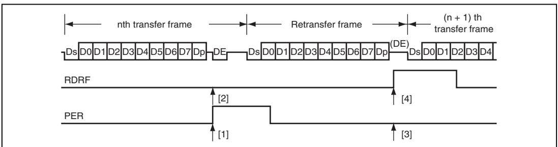
**Figure 19.32 Data Re-Transfer Operation in SCI Reception Mode**
