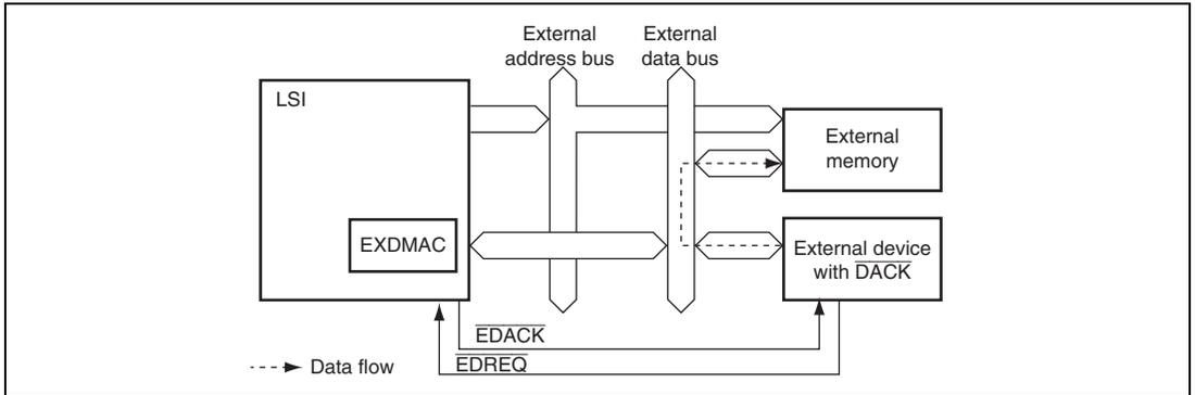
**Figure 11.4 Data Flow in Single Address Mode**
