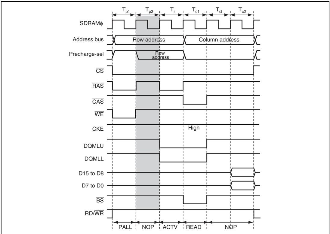
**Figure 9.65 Read Timing Example of Two Precharge Cycles**
