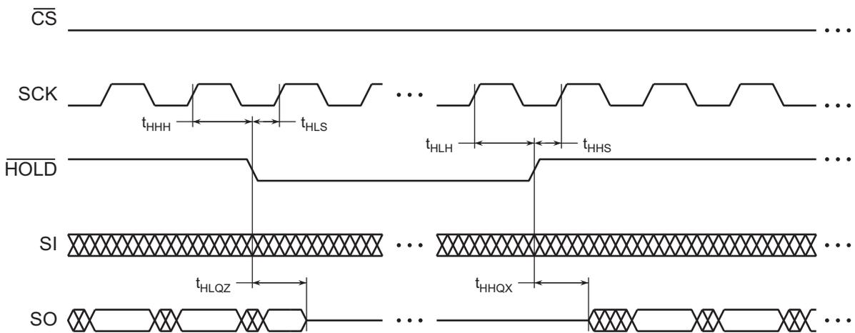
Figure 37.  $\overline{HOLD}$  Timing – Serial Output
