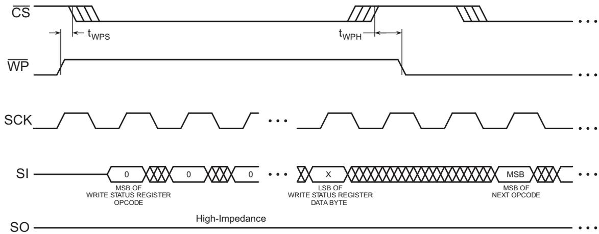
Figure 35.  $\overline{WP}$  Timing for Write Status Register Command
