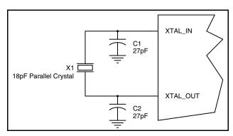
Figure 1. Crystal Input Interface
