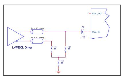
Figure 2B. General Diagram for LVPECL Driver to XTAL Input Interface
