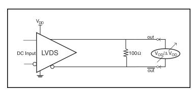
**Differential Output Voltage Setup**
