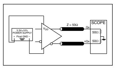
3.3V LVDS Output Load AC Test Circuit
