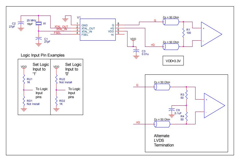
Figure 4. ICS844201-45 Schematic Example
