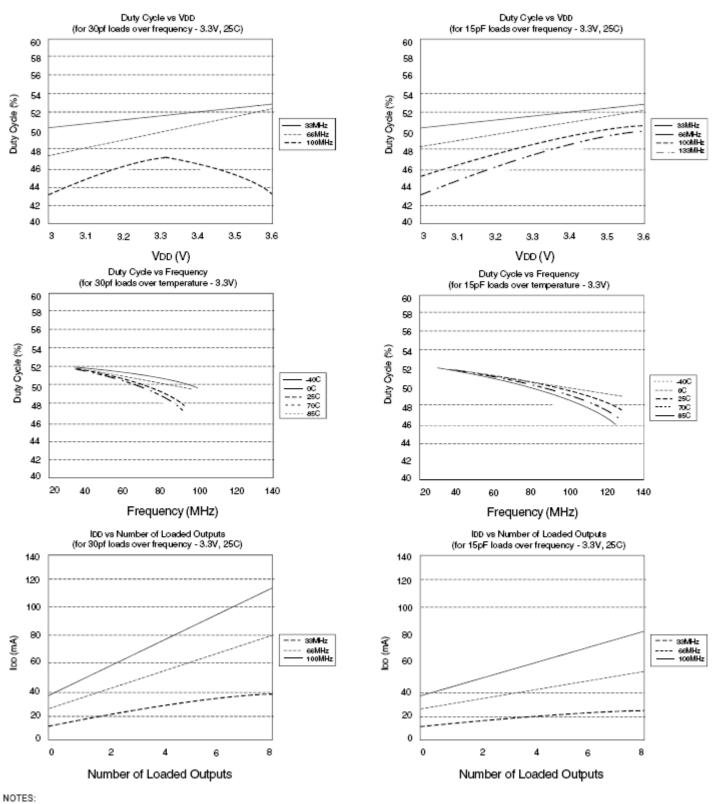
Duty Cycle is taken from typical chip measured at 1.4V.
