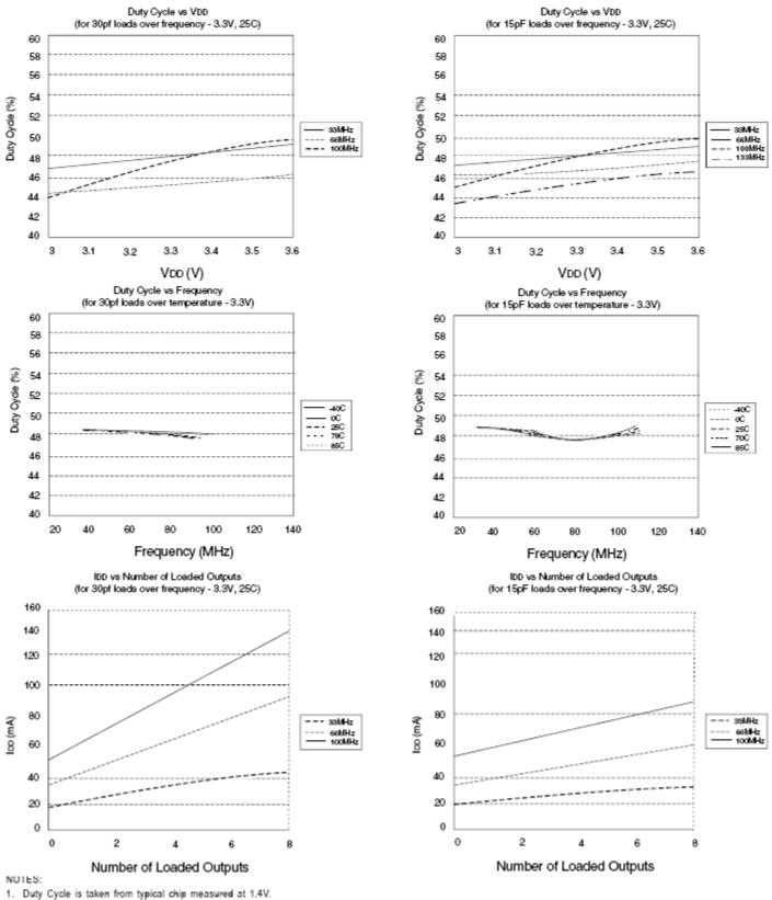
IDD data is calculated from IDD = ICORE + nCVf, where ICORE is the Unloaded Current (n = Number of Outputs; C = Capacitance Load per Output (F); V = Voltage Supply(V); f = Frequency (Hz).
