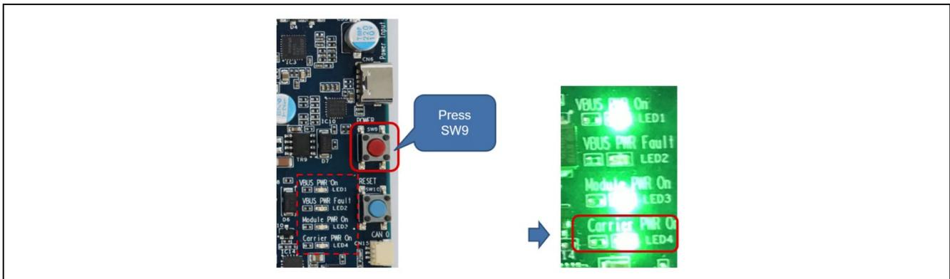
Figure 36: LED Status after Turning on EVK
