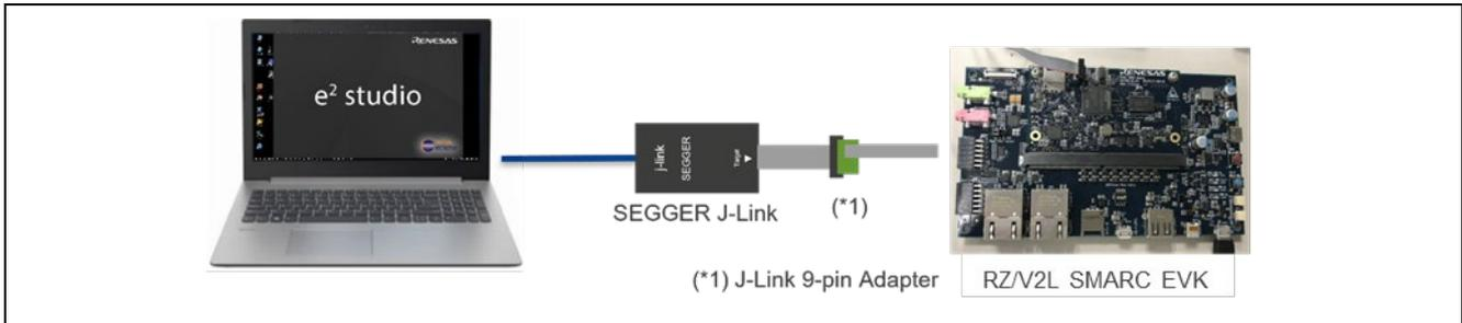
Figure 31: System Configuration Example – RZ/V2L SMARC EVK
