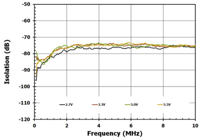
Figure 9. RFX – RFC Isolation Vs. Voltage
