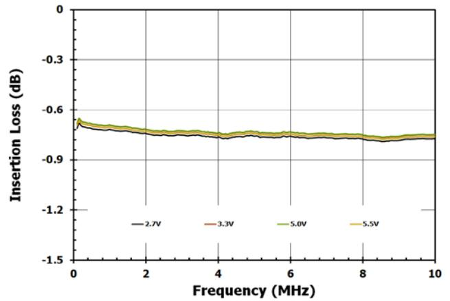
Figure 3. RFX – RFC Insertion Loss Vs. Voltage
