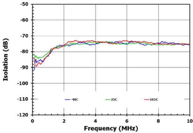
Figure 8. RFX – RFC Isolation Vs. Temperature
