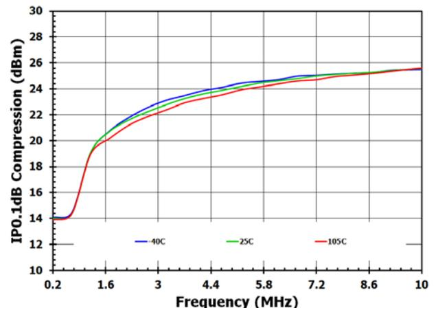
Figure 13. Input 0.1dB Compression Vs. Temperature
