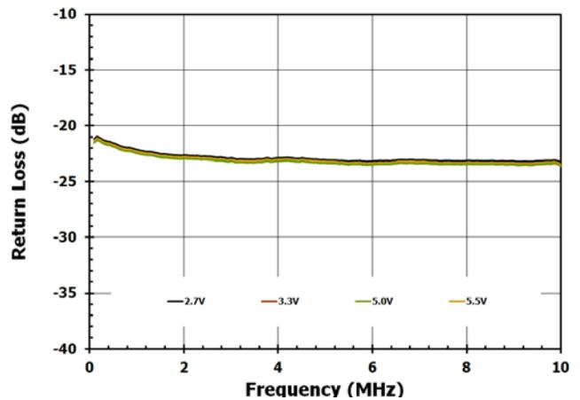
Figure 7. RFX – RFC Return Loss Vs. Voltage
