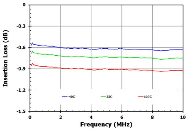
Figure 4. RFX – RFC Insertion Loss Vs. Temperature
