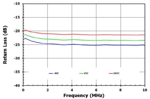
Figure 5. RFX – RFC Return Loss Vs. Temperature
