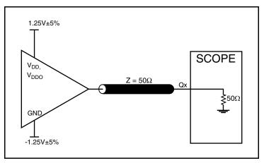
2.5V Core/2.5V LVCMOS Output Load Test Circuit
