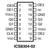
16-Lead TSSOP 4.4mm x 5.0mm x 0.92mm package body G Package Top View
