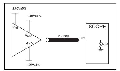
3.3V Core/2.5V LVCMOS Output Load Test Circuit
