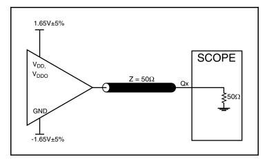
3.3V Core/3.3V LVCMOS Output Load Test Circuit
