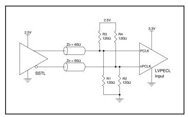
Figure 3E. PCLK/nPCLK Input Driven by an SSTL Driver
