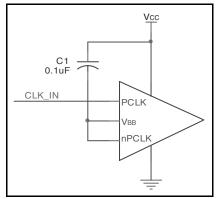
Figure 2. Single-Ended LVPECL Signal Driving Differential Input
