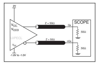
LVPECL Output Load AC Test Circuit
