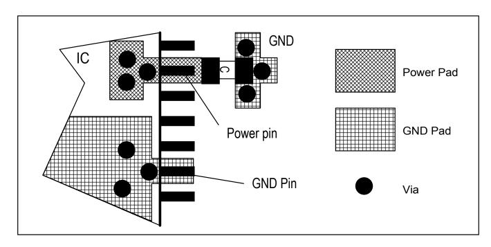
Figure 5B. Recommended Layout of Bypass Capacitor Placement
