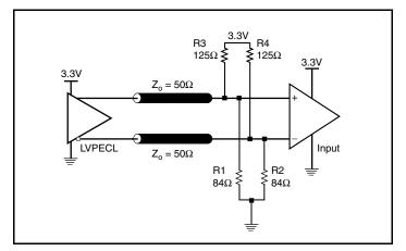
Figure 4B. 3.3V LVPECL Output Termination
