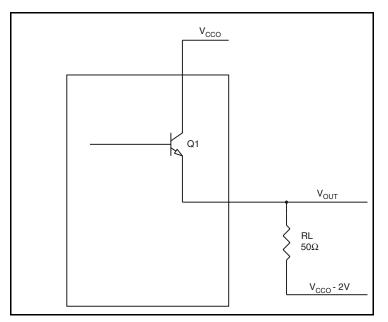
Figure 6. LVPECL Driver Circuit and Termination
