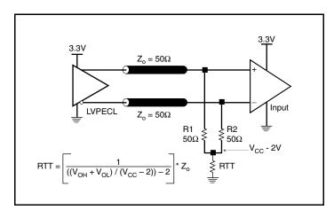
Figure 4A. 3.3V LVPECL Output Termination
