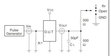
Test Circuits for All Outputs
