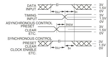
Set-up, Hold, and Release Times
