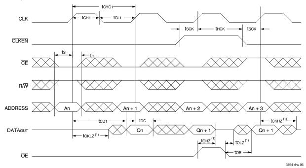
Timing Waveform of Left Port Write to Flow-Through Right Port Read  $(FT/Piped_R = VIL)^{(2,3)}$
