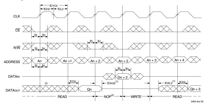
Timing Waveform of Pipelined Read-to-Write-to-Read (**OE** Controlled)
