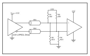
Figure 5A. 2.5V LVPECL Driver Termination Example
