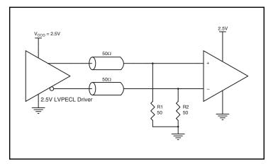
Figure 5C. 2.5V LVPECL Driver Termination Example
