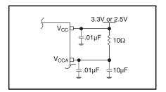
Figure 1. Power Supply Filtering
