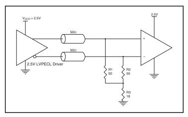
Figure 5B. 2.5V LVPECL Driver Termination Example
