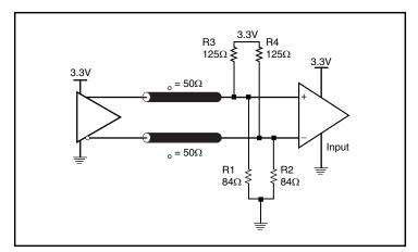
Figure 4B. 3.3V LVPECL Output Termination
