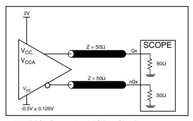
2.5V LVPECL Output Load AC Test Circuit
