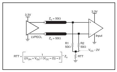
Figure 4A. 3.3V LVPECL Output Termination
