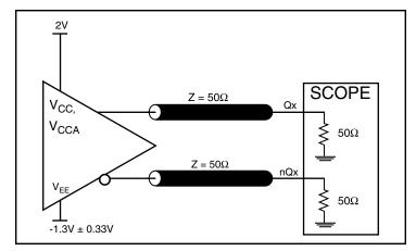
3.3V LVPECL Output Load AC Test Circuit
