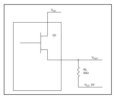
Figure 6. LVPECL Driver Circuit and Termination
