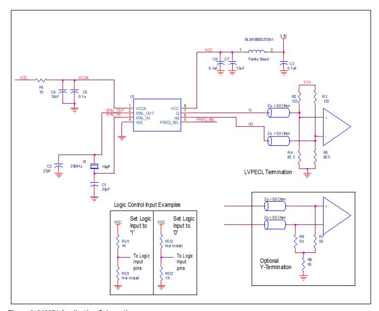
Figure 6. 843071 Application Schematic
