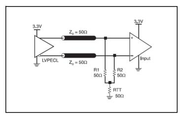
Figure 3A. 3.3V LVPECL Output Termination
