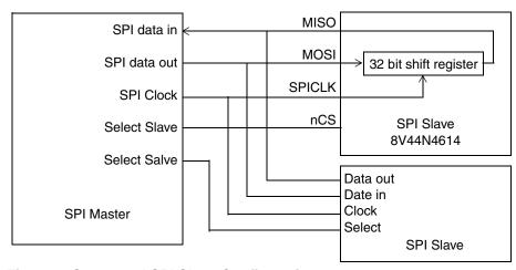
Figure 1. Supported SPI Slave Configuration
