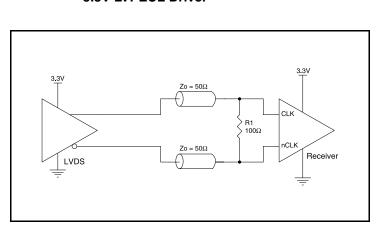
Figure 1C. CLK/nCLK Input Driven by a 3.3V LVDS Driver
