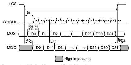
Figure 2. SPI Timing Diagram (Single Transfer)
