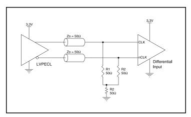
Figure 1B. CLK/nCLK Input Driven by a 3.3V LVPECL Driver
