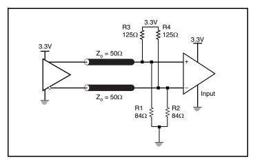
Figure 3B. 3.3V LVPECL Output Termination
