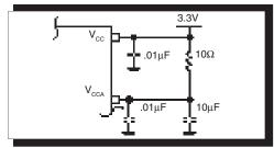
FIGURE 1. POWER SUPPLY FILTERING
