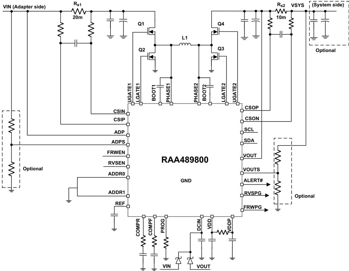
Figure 1. Typical Application Circuit in 4-Switch Buck-Boost Configuration
