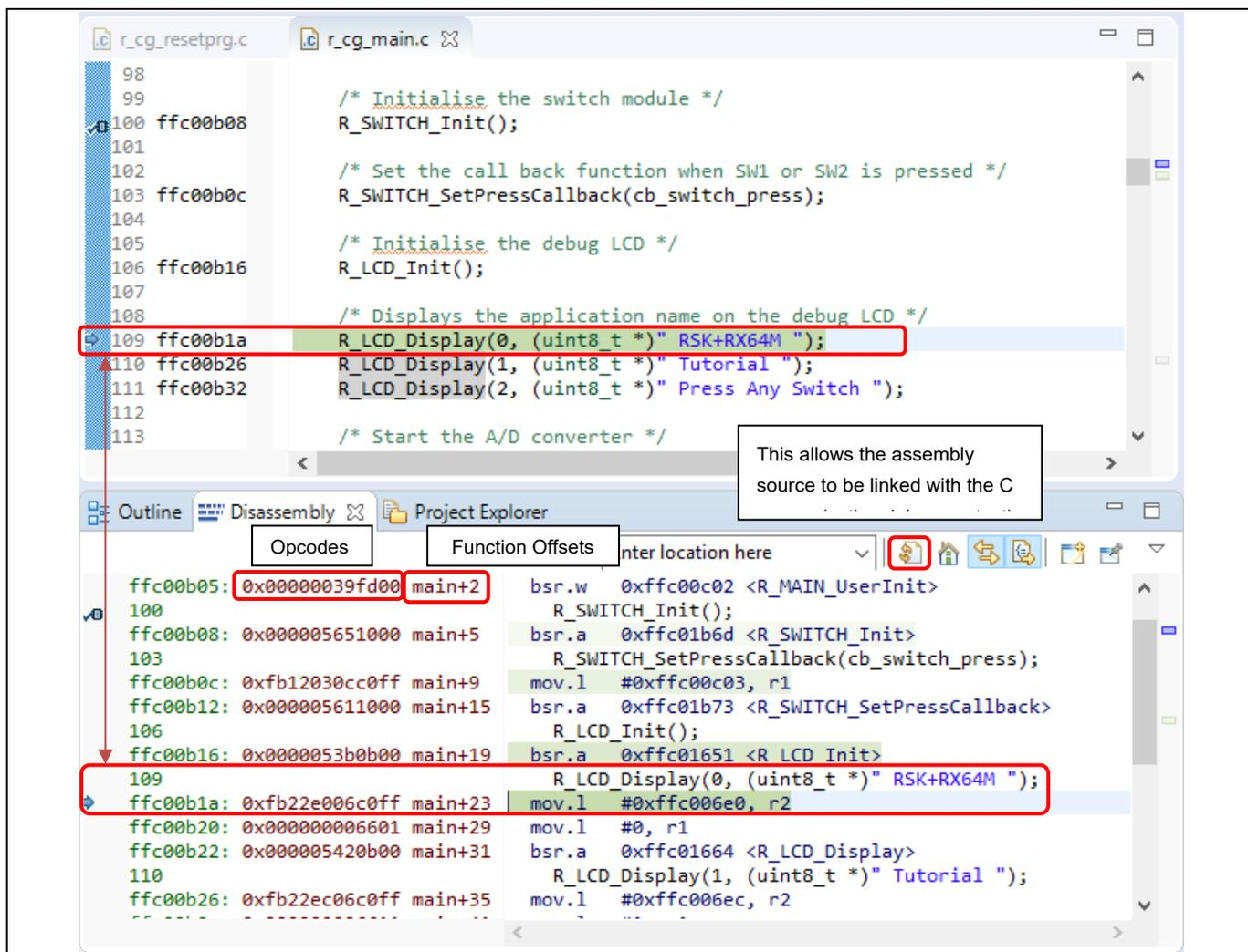
Figure 5-18 [Disassembly] View
