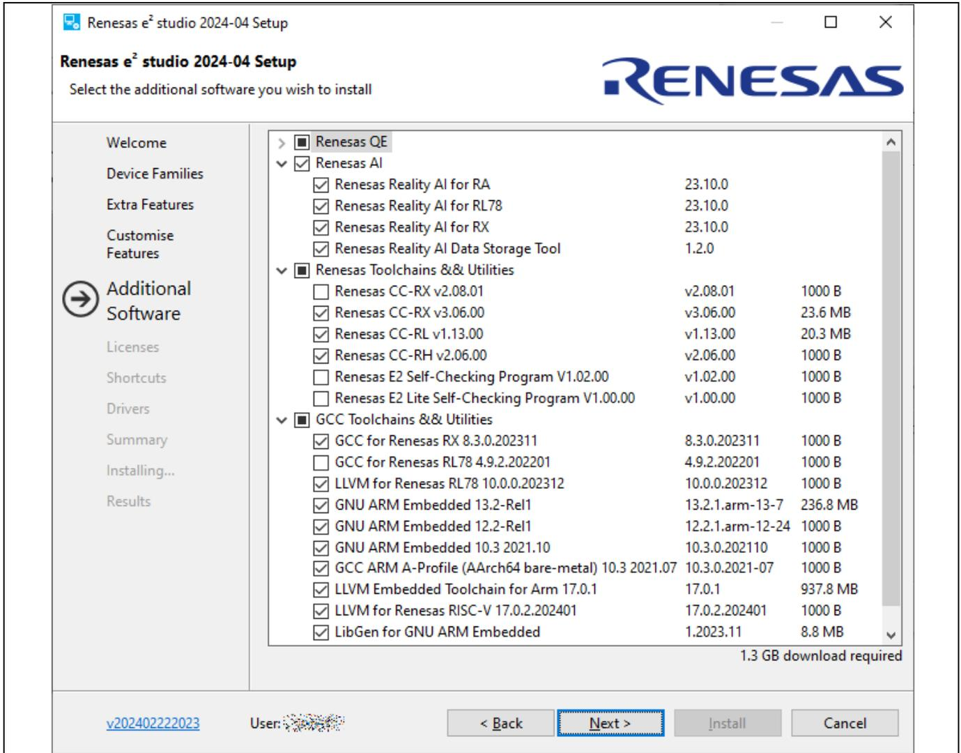
Figure 2-8 e<sup>2</sup> studio installation – Additional Software
