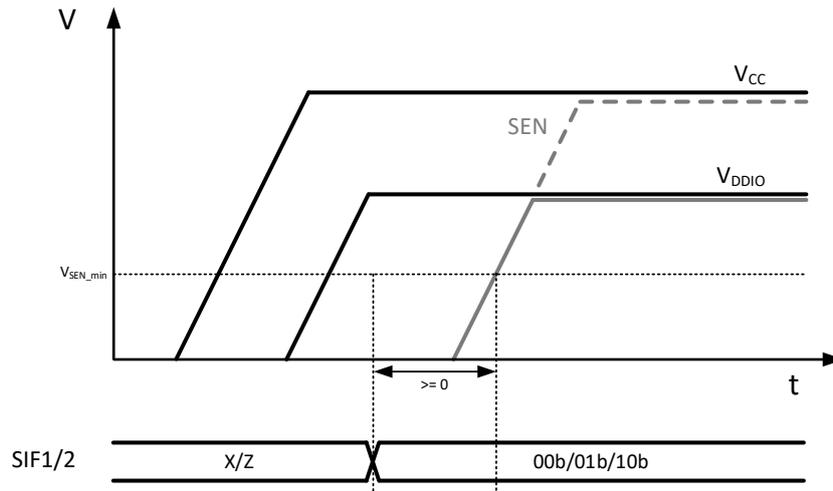
**Figure 4: Supply Ramping Up (SEN at logic-low)**
