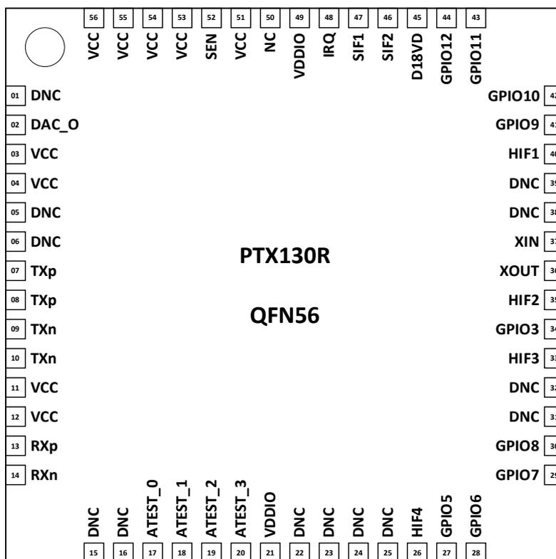
Figure 2: Pin Diagram
