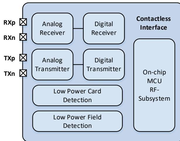
Figure 6: Contactless Interface
