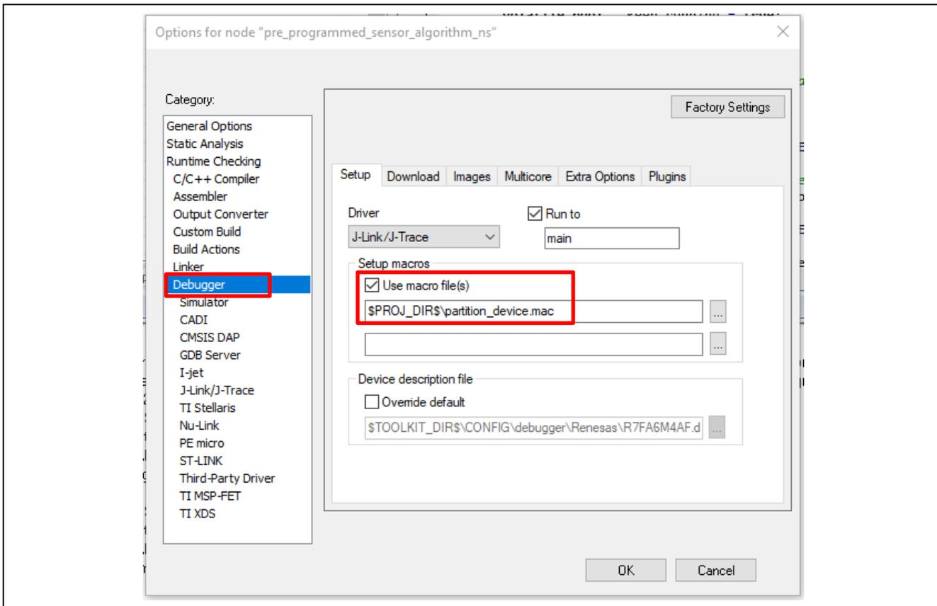
**Figure 8. Debug Configuration for IDAU Region Setup**
