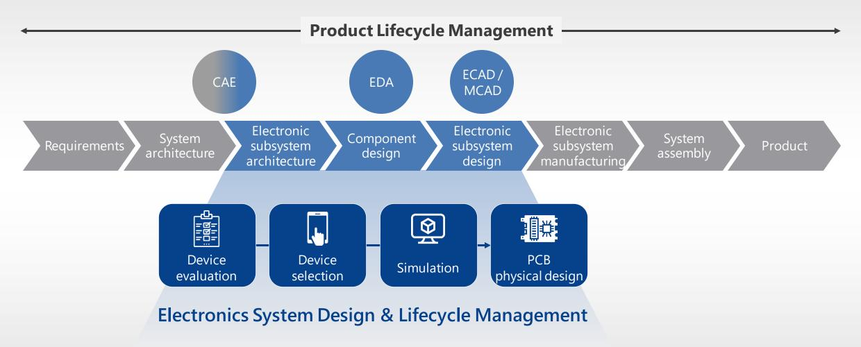
CAE: Computer Aided Engineering EDA: Electronic Design Automation ECAD: Electrical CAD MCAD: Mechanical CAD
