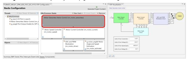
For RX family devices, the motor software configuration GUI is displayed in the [Motor Middleware Configurator (QE)] view of the e<sup>2</sup> studio. The [Motor Middleware Configurator (QE)] view is opened by selecting the sample project supporting this feature and clicking [Start Configuration] button on [Motor Main (QE)] view. For the sample projects supporting this feature, refer to **1.4 Supported Software of Motor Software Configuration GUI**.
