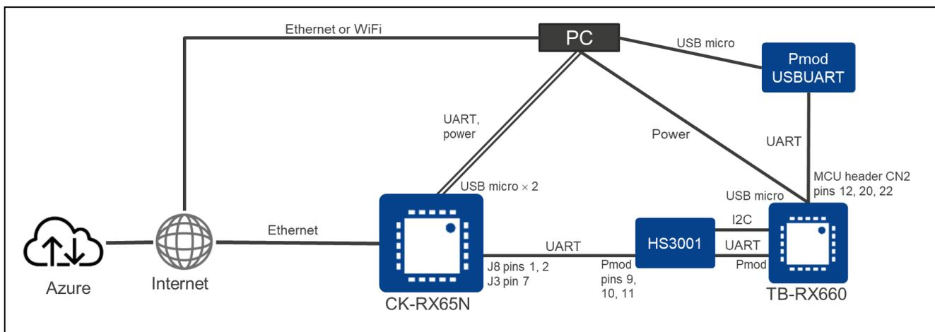
Figure 6-1 Overall Hardware Structure for This Demo
