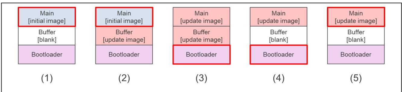
Figure 4-3 States of ROM in the Secondary MCU during Updating
