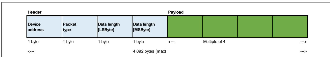
Figure 4-4 Data Format of a Whole Packet
