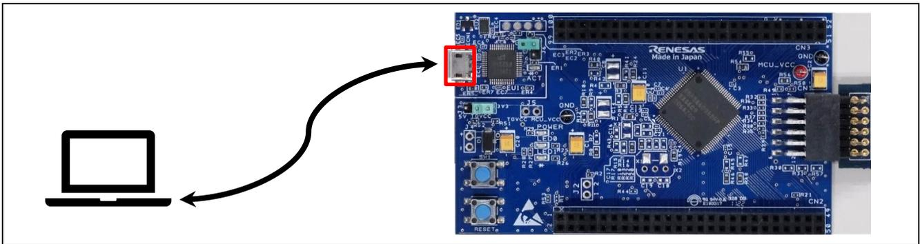
Figure 6-10 Connecting the USB Cable for the Power Supply and Emulator
