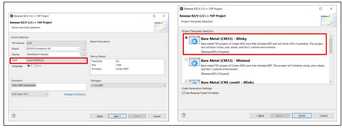
Figure 93 : Setting of CM33 core project
