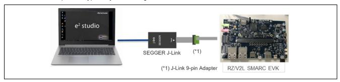
Figure 31: System Configuration Example – RZ/V2L SMARC EVK
