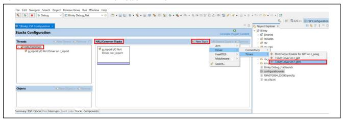
Figure 80: e<sup>2</sup> studio Project configurator - Adding drivers
