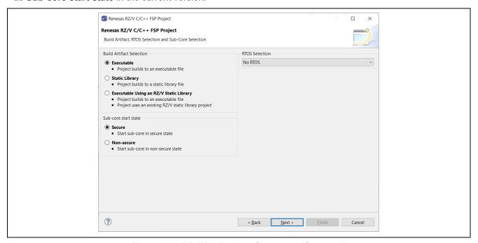
Figure 68: RZ MPU Project Generator (Screen 3)
