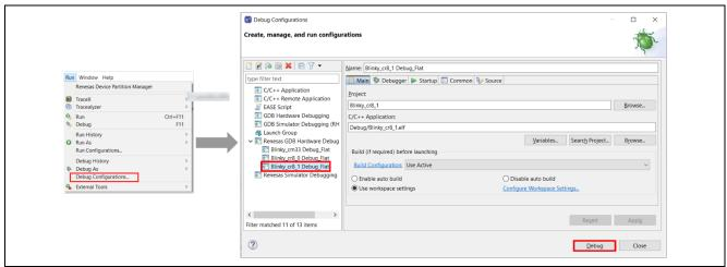
Figure 101 : CR8 Core1 Debug Configuration
