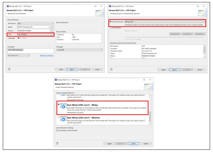
Figure 95 : Setting of CR8 core1 project
