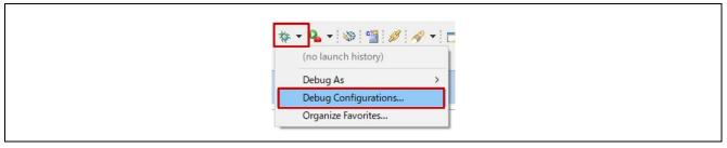
Figure 55: e<sup>2</sup> studio Debugger Configurations selection option
