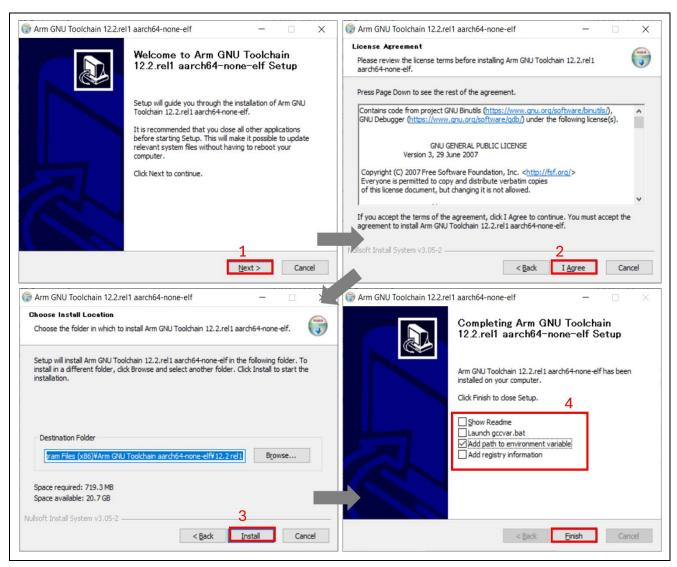
Figure 11: Installation of GNU ARM Embedded Toolchain
