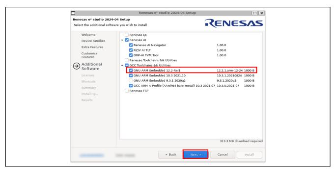
Figure 19: Installation of e<sup>2</sup> studio - Additional Software
