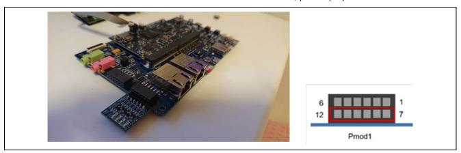
Figure 43: Connection Pmod LED module (410-076)
