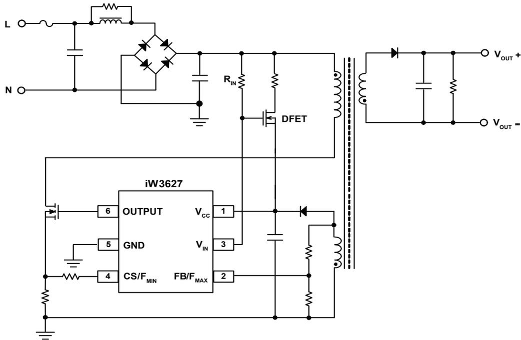
Figure 3.1 : iW3627 Typical Application Circuit (Isolated Flyback Application)
