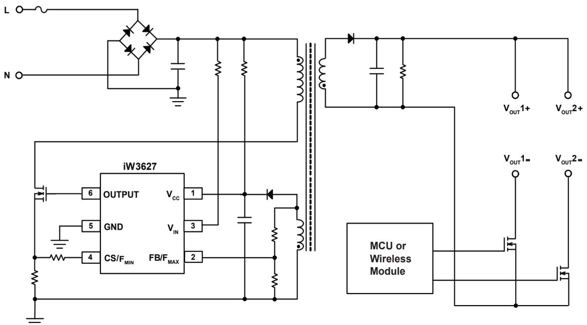
Figure 3.4 : iW3627 Typical Application Circuit (Smart Lighting)
