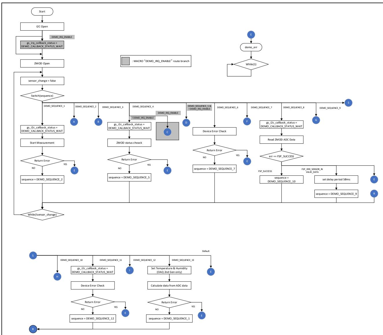
Figure 6-6 Flow 1 of ZMOD4510 Sample Software Main Processing
