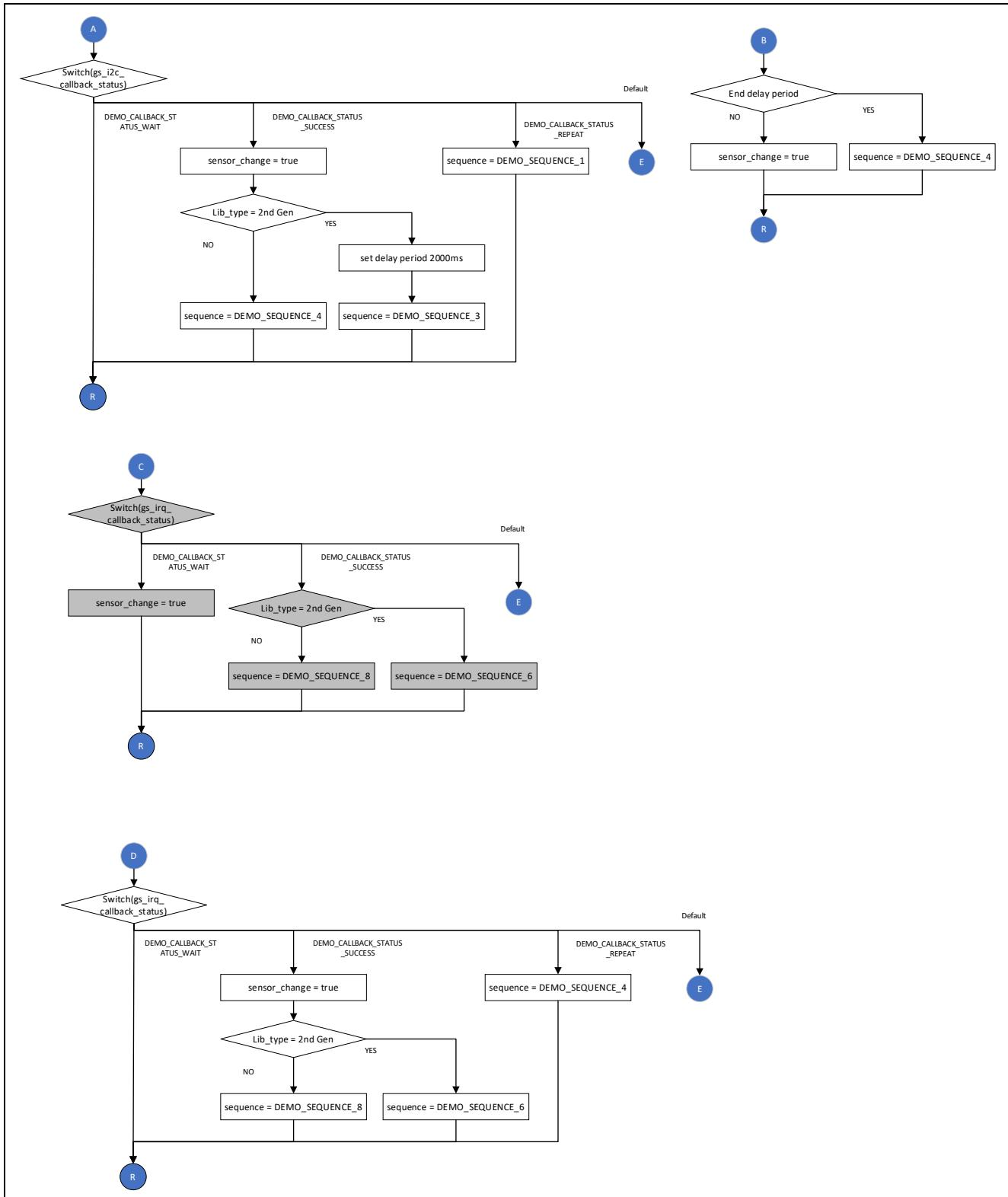
Figure 6-7 Flow 2 of ZMOD4510 Sample Software Main Processing
