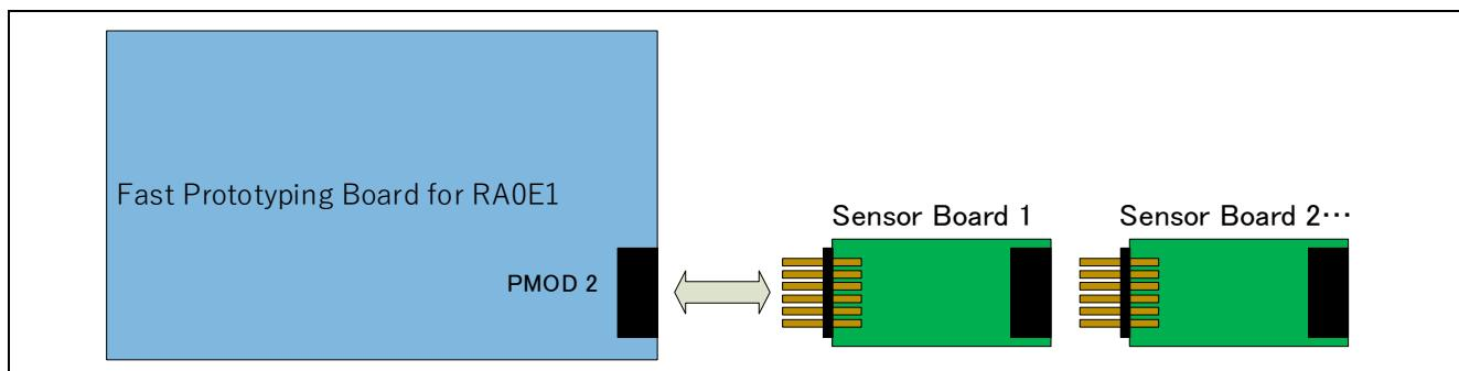
Figure 2-2 Hardware Connections for the RA0E1 Family
