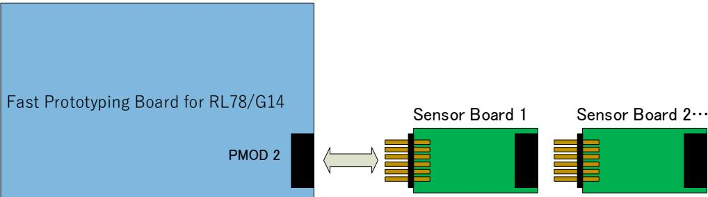
Figure 2-4 Hardware Connections for RL78/G14 Group
