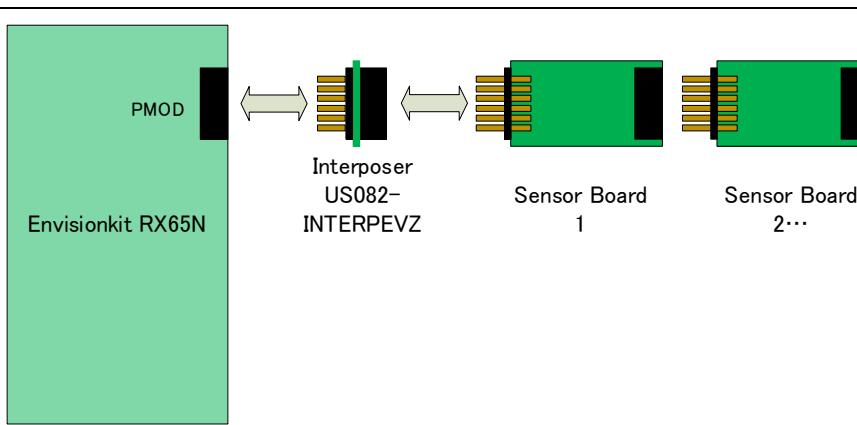
Figure 2-3 Hardware Connections for RX Family
