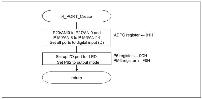
Figure 5.4 I/O Port Setup
