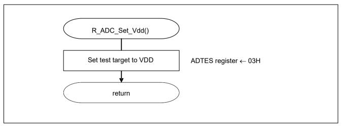
Figure 5.11 Setting the Test Voltage to VDD
