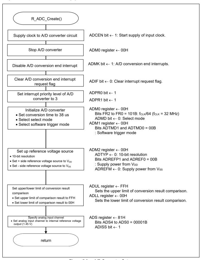
Figure 5.6 A/D Converter Setup
