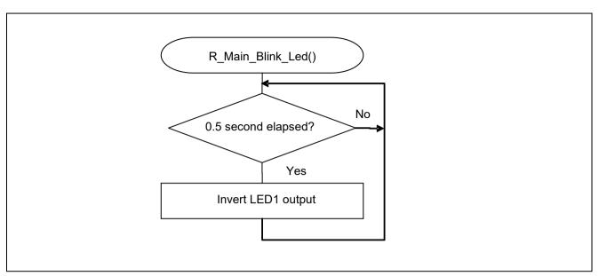
Figure 5.19 Blinking the LED
