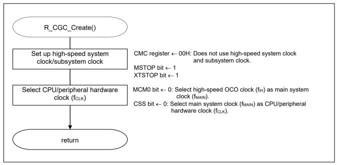
Figure 5.5 CPU Clock Setup
