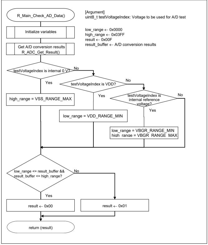
Figure 5.17 Checking the A/D Conversion Results
