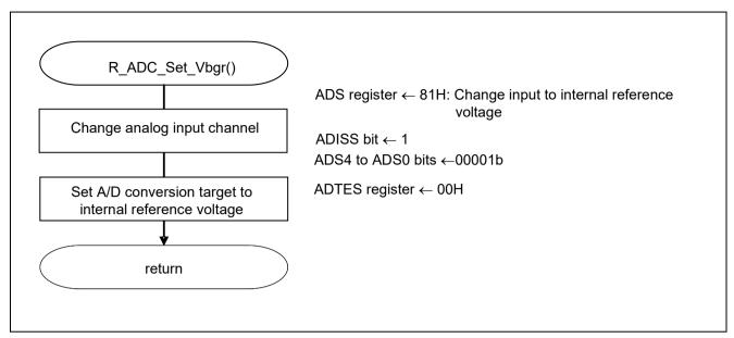
Figure 5.12 Setting The Test Voltage to Internal Reference Voltage
