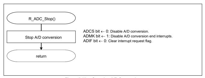
Figure 5.16 Stopping A/D Conversion
