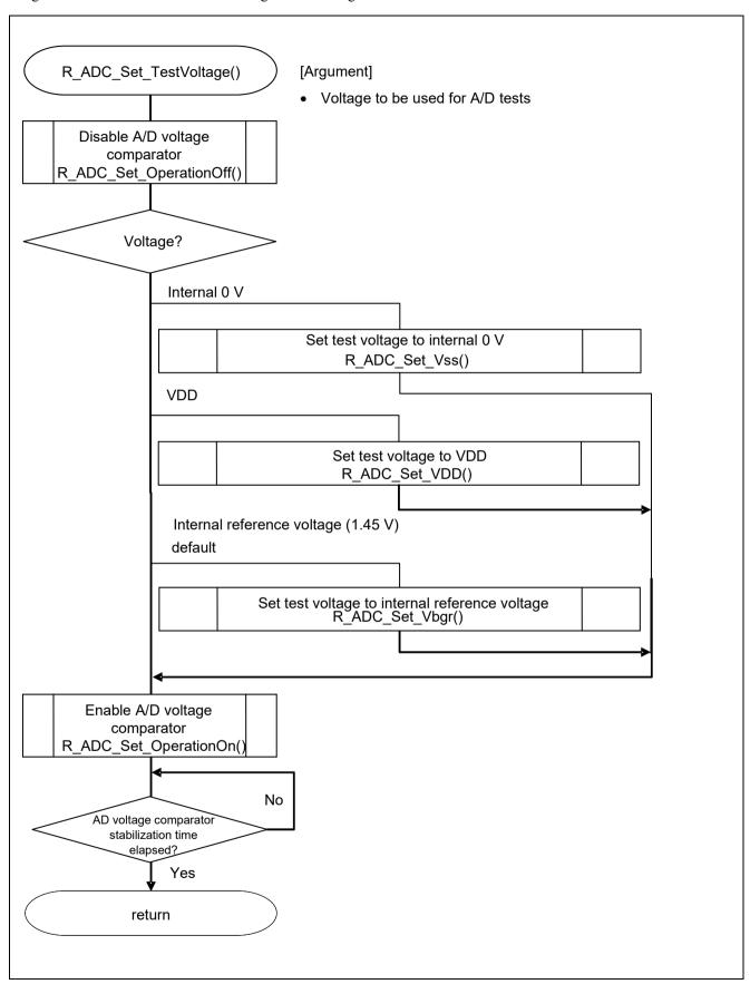
Figure 5.9 Setting the Test Voltage
