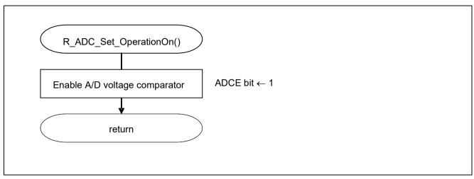
Figure 5.13 **Enabling the A/D Voltage Comparator**
