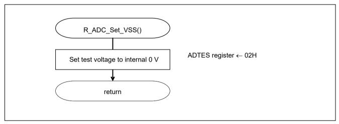
Figure 5.10 Setting the Test Voltage to Internal 0 V
