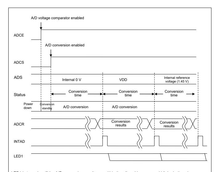
LED1 is turned on if the A/D conversion results are within the allowable range and blinked otherwise.
